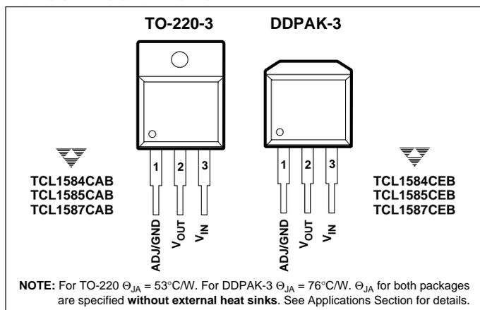
The TCL1584/1585/1587 are low dropout, positive linear voltage regulators. They have a maximum current output specification of 7A, 5A, 4.6A and 3A respectively. All three devices are supplied in fixed and adjustable output voltage versions.
