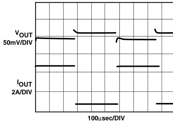
\*TRANSIENT RESPONSE MEASURED WITH AN INTEL POWER VALIDATOR™.  $V_{OUT}$  IS MEASURED AT THE POWER VALIDATOR.
