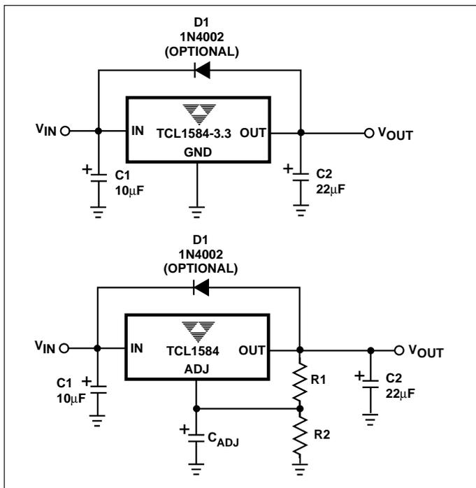
Figure 2. Protection Diodes and C<sub>ADJ</sub>
