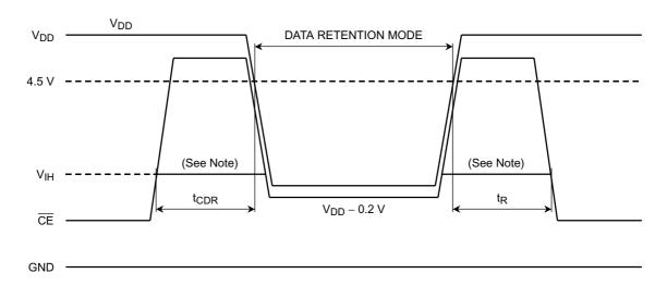
Note: When  $\overline{\text{CE}}$  is operating at the VIH level (2.2V), the standby current is given by IDDS1 during the transition of VDD from 3.6 to 2.4V.
