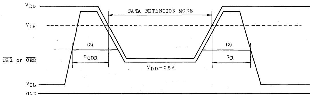
2. If the  $V_{IH}$  level of  $\overline{CE}_2$  ( $\overline{CE}_1$ ) is 2.2V, during the period that the  $V_{DD}$  voltage is going down from 4.5V to 2.7V, I<sub>DD1</sub> current flows.
