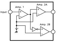
(Fig.1) Block diagram
