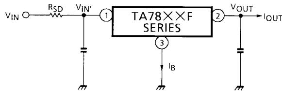
The power dissipation  $P_D$  of IC is expressed in the following equation.
