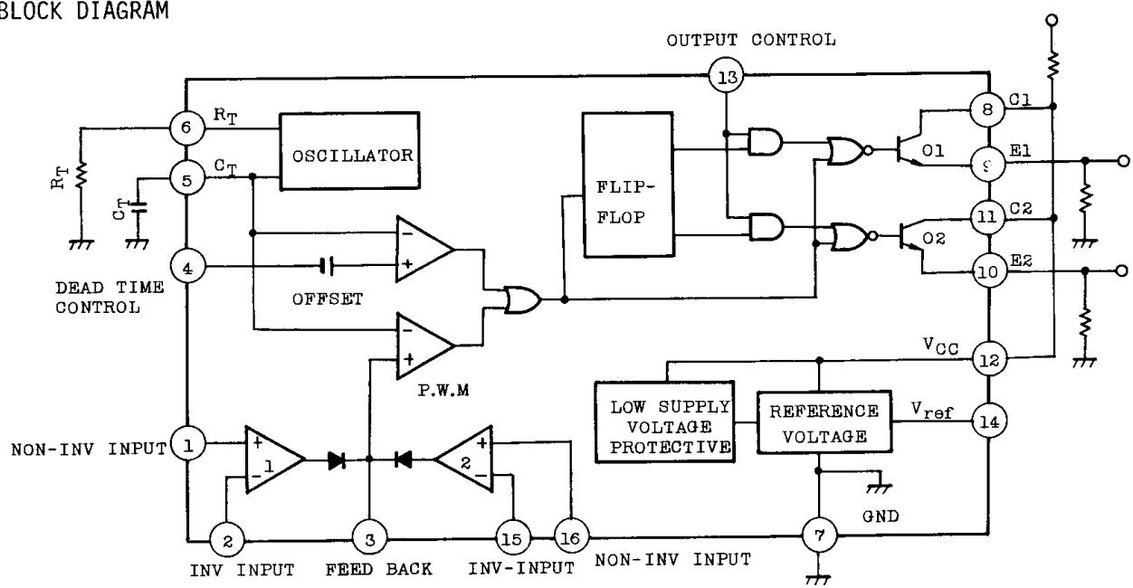
(Note) PIN 13 BECOMES SINGLE MODE AT "L" AND PUSH-PULL MODE AT "H".
