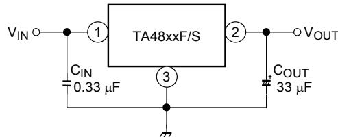
Be sure to connect a capacitor near the input terminal and output terminal between both terminals and GND. The capacitances should be determined experimentally. In particular, adequate investigation should be made so that there is no problem even in high or low temperature.
