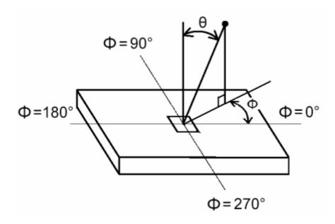
Fig.4-3 Viewing Angle Definition
