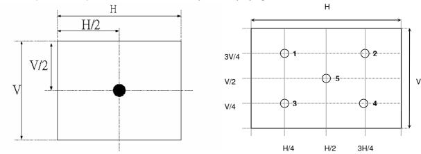
Fig.4-2 Optical measurement point
