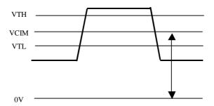
Figure: LVDS Differential Voltage
