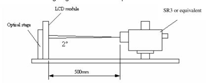
Fig.4-1 Optical measurement equipment and method
