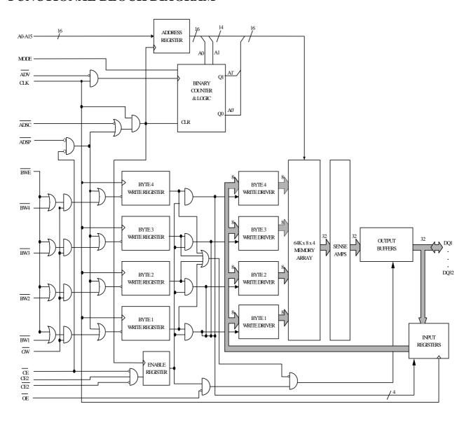
Note: The Functional Block Diagram illustrates simplified device operation. See Truth Table, pin descriptions and timing diagrams for detailed information.
