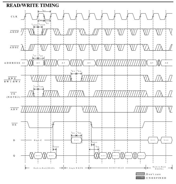
**Note:** 1. Q(A4) refers to output from address A4. Q(A4 + 1) refers to output from the next internal burst address following A4.
