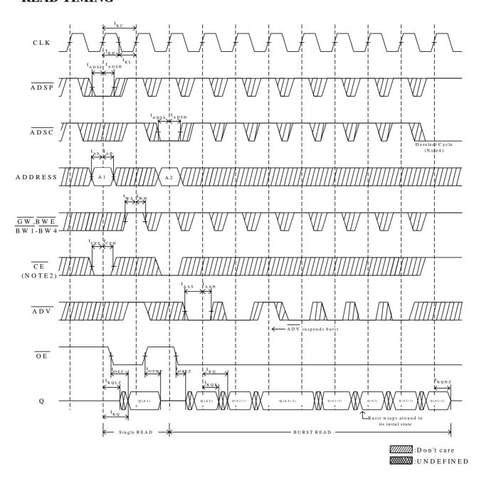
**Note:** 1. Q(A2) refers to output from address A2. Q (A2 + 1) refers to output from the next internal burst address following A2.
