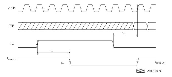
**Note:** 1. The  $\overline{CE}$  signal shown above refers to a TRUE state on all chip selects for the device.
