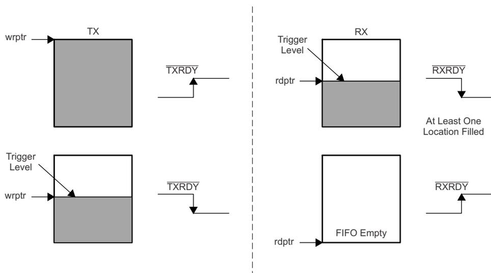
Figure 25.  $\overline{\text{TXRDY}}$  and  $\overline{\text{RXRDY}}$  in DMA Mode 1
