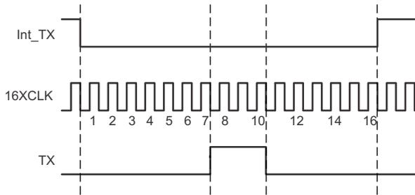
**Figure 33. IrDA-SIR Decoding Scheme – Detailed Timing Diagram**
