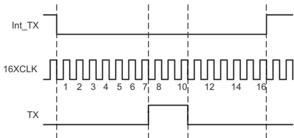
Figure 31. IrDA-SIR Encoding Scheme – Detailed Timing Diagram
