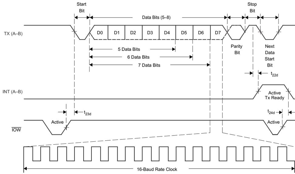
**Figure 7. Transmit Timing**
