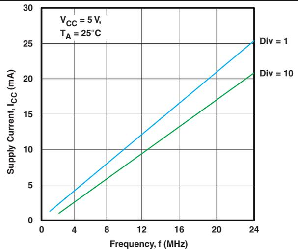
Figure 13. Supply Current vs Frequency ( $V_{CC} = 5\text{ V}$ )
