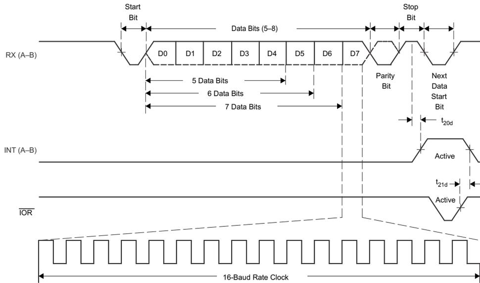
Figure 4. Receive Timing
