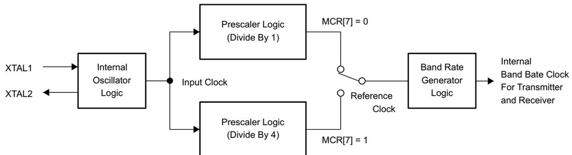
**Figure 22. Prescaler and Baud Rate Generator Block Diagram**
