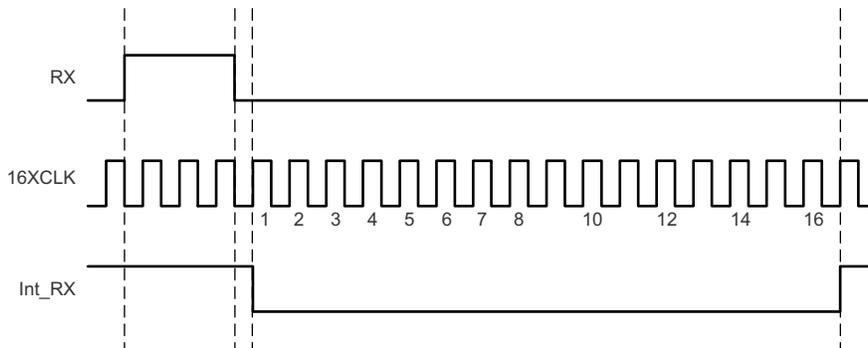
Figure 37. Positive RX Pulse Decode – Detailed View
