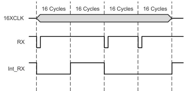
**Figure 34. IrDA-SIR Decoding Scheme – Macro View**
