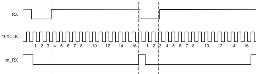
**Figure 35. Timing Causing 1-Clock-Wide Pulse Between Consecutive Ones**
