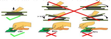
5. Precaution for soldering the LCM
