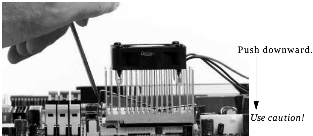
Figure 15. Pushing the Heatsink Clip Down
