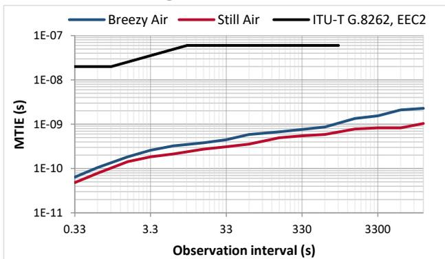
Figure 22. MTIE (0.1 Hz loop bandwidth) [15]
