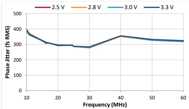
Figure 44. RMS Phase Jitter, VCTCXO (Clipped Sine)
