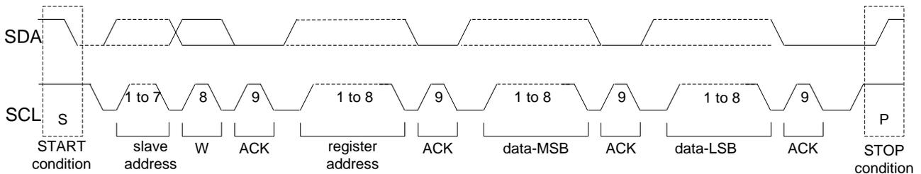
Figure 56. Parallel data byte format, write operation
