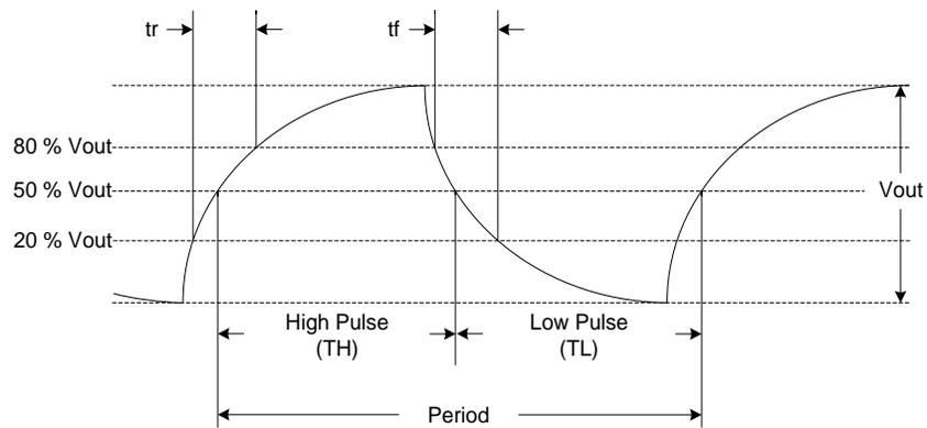
Figure 16. Clipped Sinewave Waveform Diagram<sup>[14]</sup>
