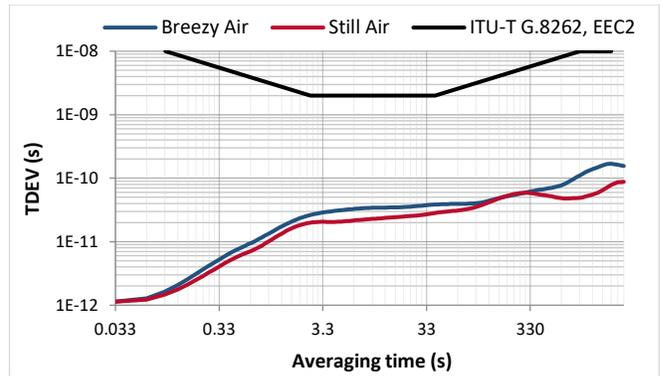
Figure 21. TDEV (0.1 Hz loop bandwidth) [15]
