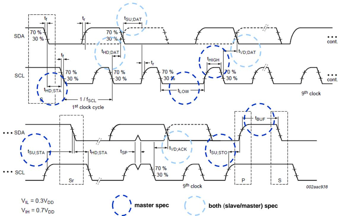
**Figure 59. I<sup>2</sup>C Timing Diagram**
