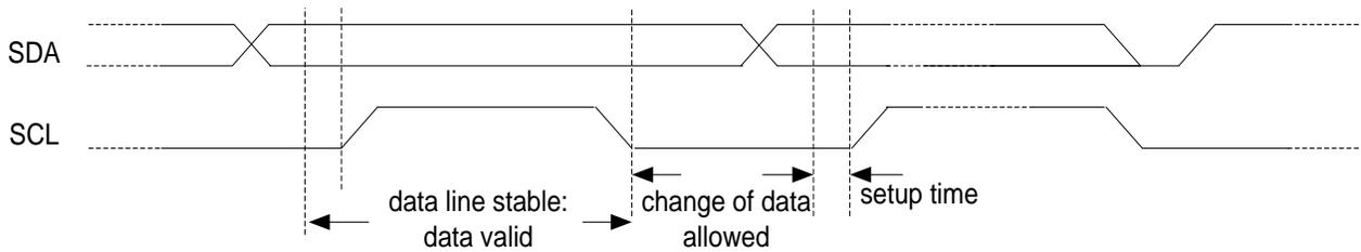
**Figure 53. Data and clock timing relation in I<sup>2</sup>C bus**
