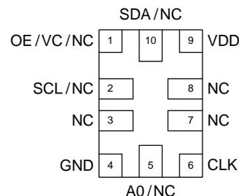
Figure 2. Pin Assignments (Top view)
