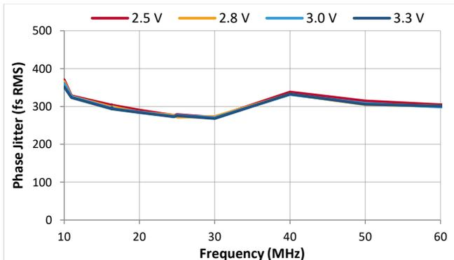
Figure 34. RMS Phase Jitter, DCTCXO, TCXO (LVCMOS)
