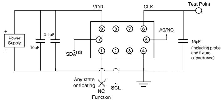
Figure 12. LVCMOS Test Circuit (I<sup>2</sup>C Control), DCTCXO mode for AC and DC Measurements
