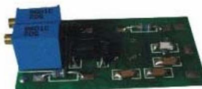
0.05F.S. There are total five points, connect to position transmitter and power supply.(size:PCB22x45mm)
