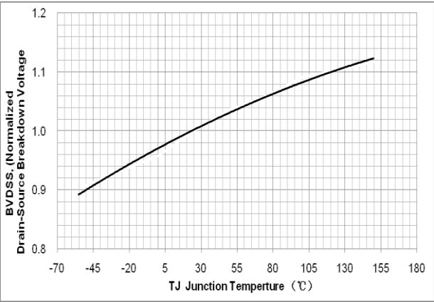
Fig 5. Breakdown Voltage Variation vs. Junction Temperature
