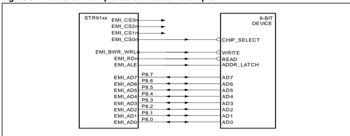
Figure 6. EMI 8-bit non-multiplexed connection example
