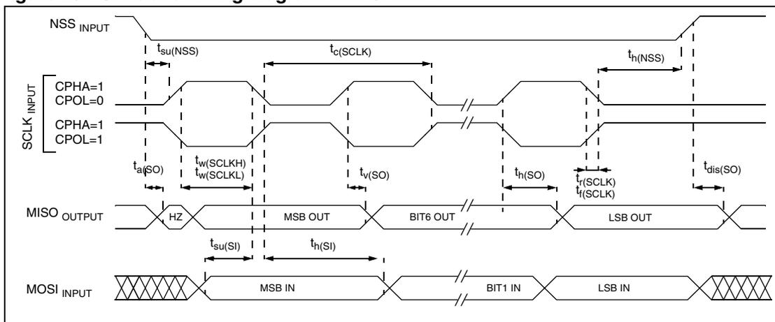
Figure 26. SPI master timing diagram
