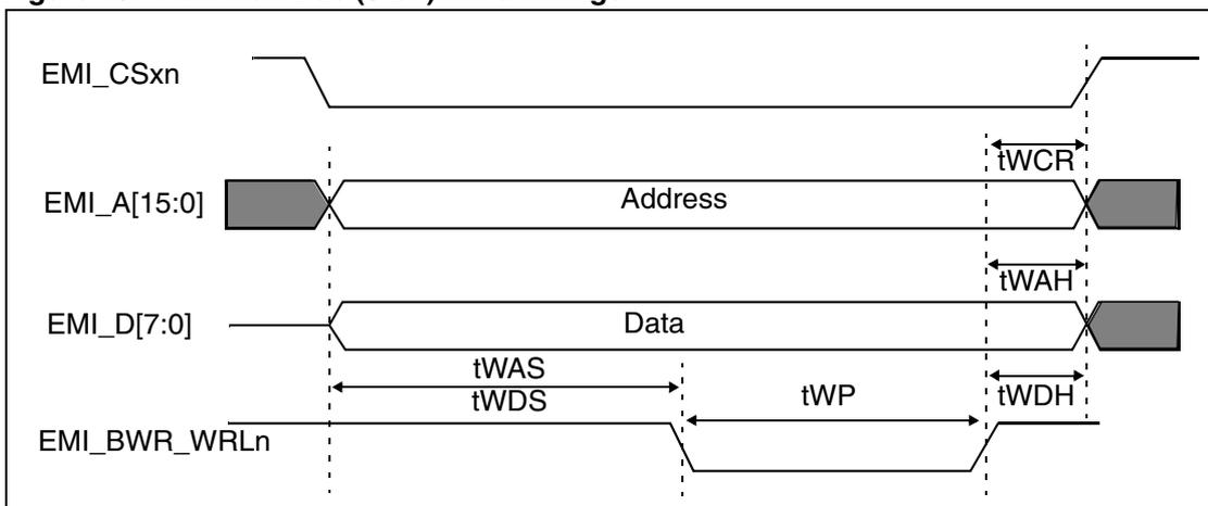
**Figure 16. Mux Bus (16-bit) Write Timings**
