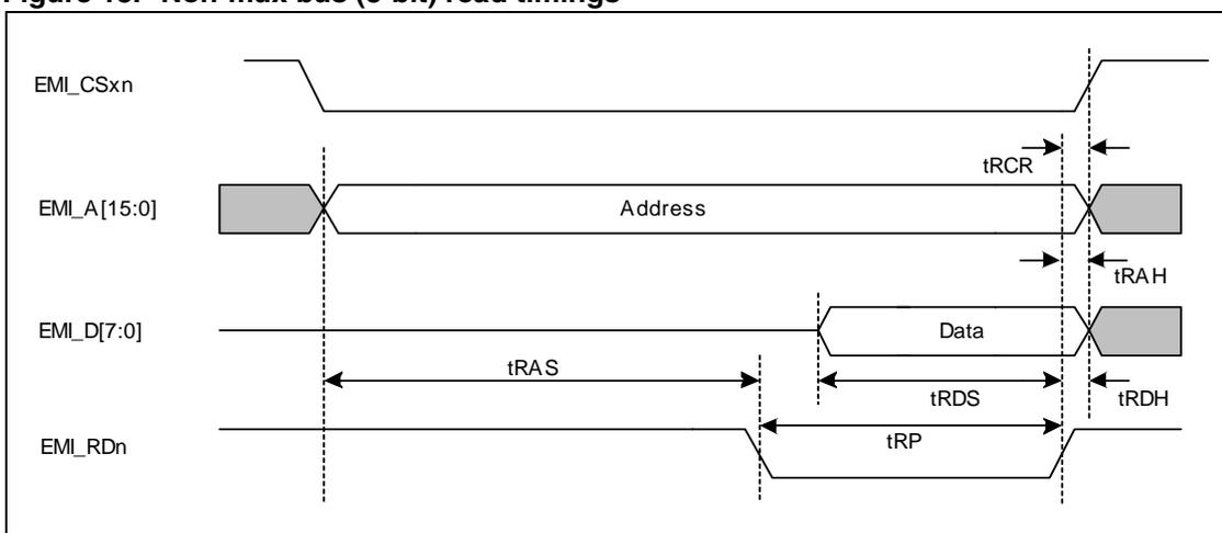
Figure 14. Mux bus (16-bit) read timings
