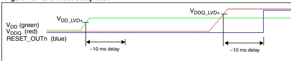
**Case 2:** When  $V_{DDQ}$  reaches the  $V_{DDQ\_LVD+}$  threshold **before** the first ~10 ms delay (introduced by the VDD rising edge), RESET\_OUTn will be released immediately at the end of the delay. No new delay is introduced in this case. See [Figure 11](#).
