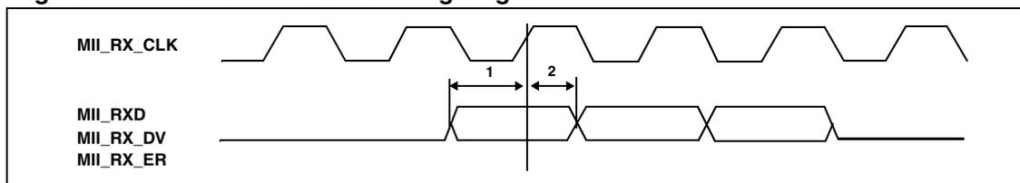
Figure 23. Ethernet MII receive timing table
