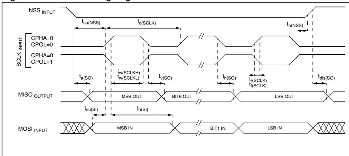
Figure 25. SPI slave timing diagram with CPHA=1
