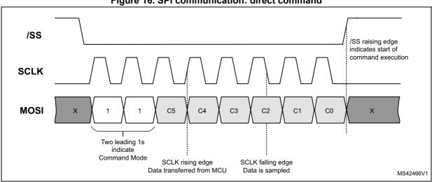
Figure 16. SPI communication: direct command
