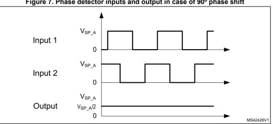
Figure 7. Phase detector inputs and output in case of 90° phase shift
