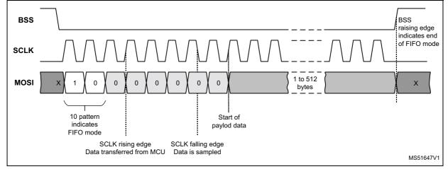
Figure 14. SPI communication: FIFO loading
