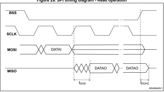
Figure 29. SPI timing diagram - Read operation
