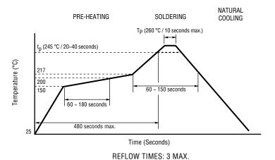
NOTE: 0.12 mm thick solder paste recommended.
