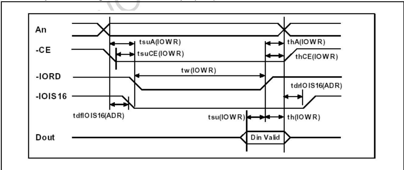
**Compact Flash Timing True IDE Mode I/O Output (Write)**
