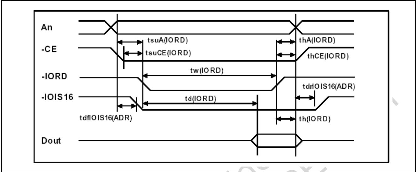
**Compact Flash Timing True IDE Mode I/O Input (Read)**
