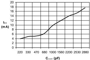
Figure 4: Supply Current vs Load Capacitor
