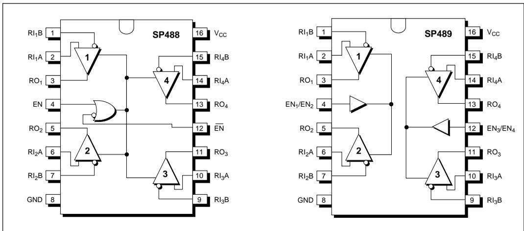
Pin 13 — RO<sub>4</sub> — Receiver 4 Output — If Receiver 4 output is enabled, if RI<sub>4A</sub> > RI<sub>4B</sub> by 200mV, Receiver 4 output is high. If Receiver 4 output is enabled, and if RI<sub>4A</sub> < RI<sub>4B</sub> by 200mV, Receiver 4 output is low.
