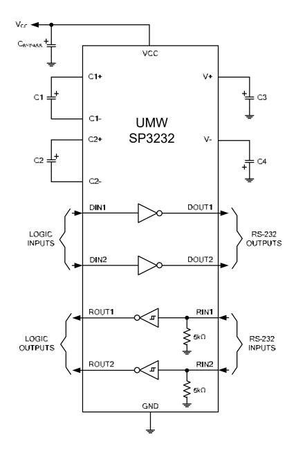
Notes: 1.C3 can be connected to  $V_{\text{CC}}$  or GND.
