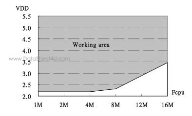
Working Voltage vs. Frequency (Noise Filter Disable · 25℃)
