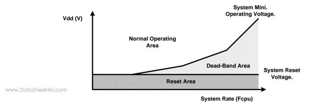
Normally the system operation voltage area is higher than the system reset voltage to VDD, and the reset voltage is decided by LVD detect level. The system minimum operating voltage rises when the system executing rate upper even higher than system reset voltage. The dead-band definition is the system minimum operating voltage above the system reset voltage.
