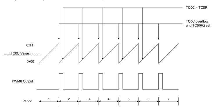
Above diagram is shown the waveform with fixed TC0R. In every TC0C overflow PWM output "High, when TC0C≧ TC0R PWM output "Low". If TC0R is changing in the program processing, the PWM waveform will became as following diagram.
