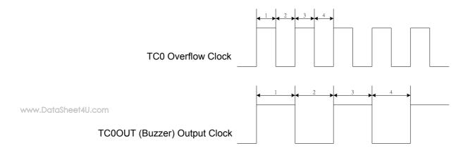
Example: Setup TC0OUT output from TC0 to TC0OUT (P5.4). The external high-speed clock is 4MHz. The TC0OUT frequency is 0.5KHz. Because the TC0OUT signal is divided by 2, set the TC0 clock to 1KHz. The TC0 clock source is from external oscillator clock. T0C rate is Fcpu/4. The TC0RATE2~TC0RATE1 = 110. TC0C = TC0R = 131.
