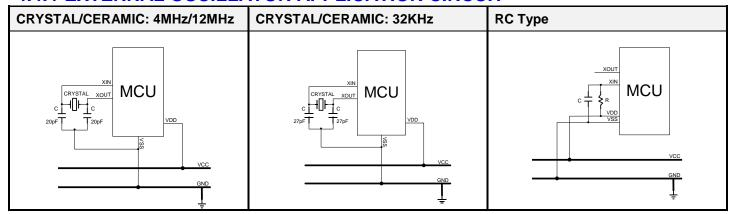
Note: Connect the Crystal/Ceramic and C as near as possible to the XIN/XOUT/VSS pins of micro-controller. Connect the R and C as near as possible to the VDD pin of micro-controller.
