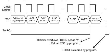
To clock source is Fcpu (instruction cycle) through Torate[2:0] pre-scaler to decide Fcpu/2~Fcpu/256. To length is 8-bit (256 steps), and the one count period is each cycle of input clock.
