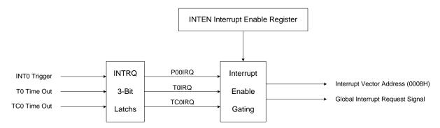
Note: The GIE bit must enable during all interrupt operation.
