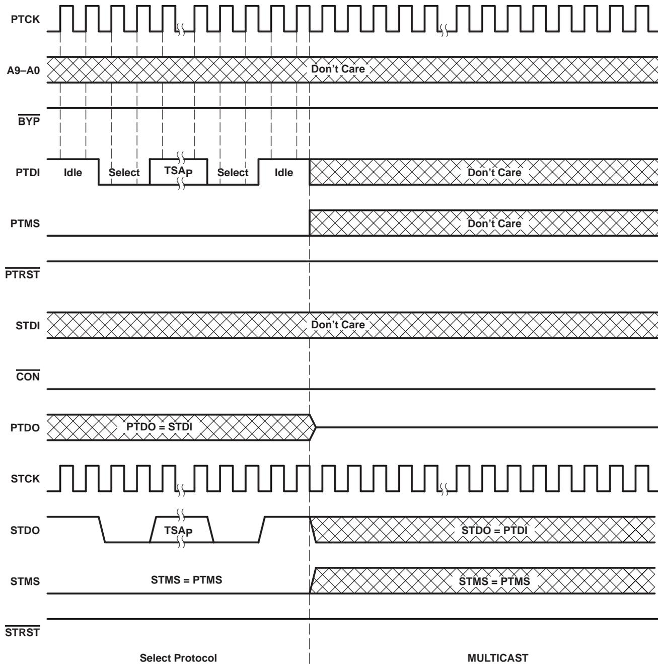
**Figure 14. Shadow-Protocol Timing,
