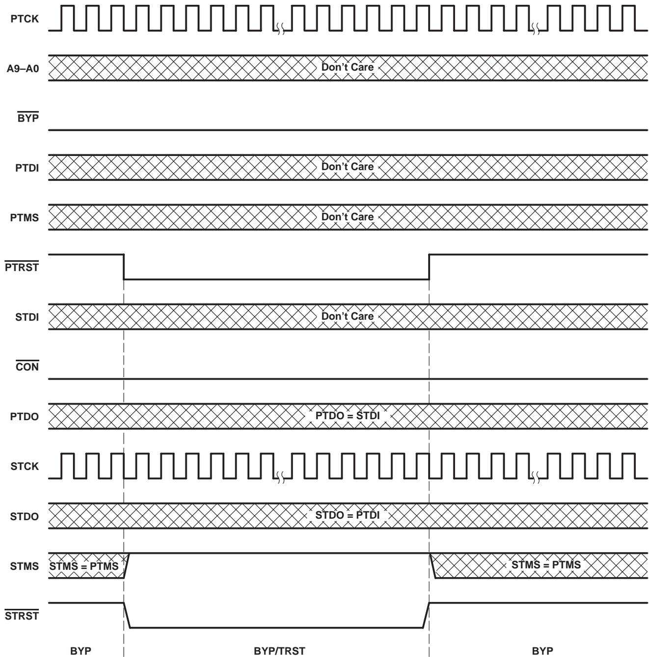
Figure 23. Asynchronous Reset Timing,  $\overline{\text{BYP}} = \text{L}$
