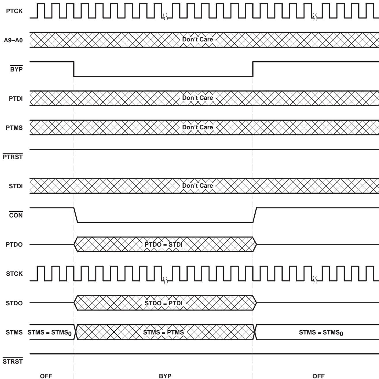
Figure 20. Protocol-Bypass Timing, Prior Connect Status = OFF
