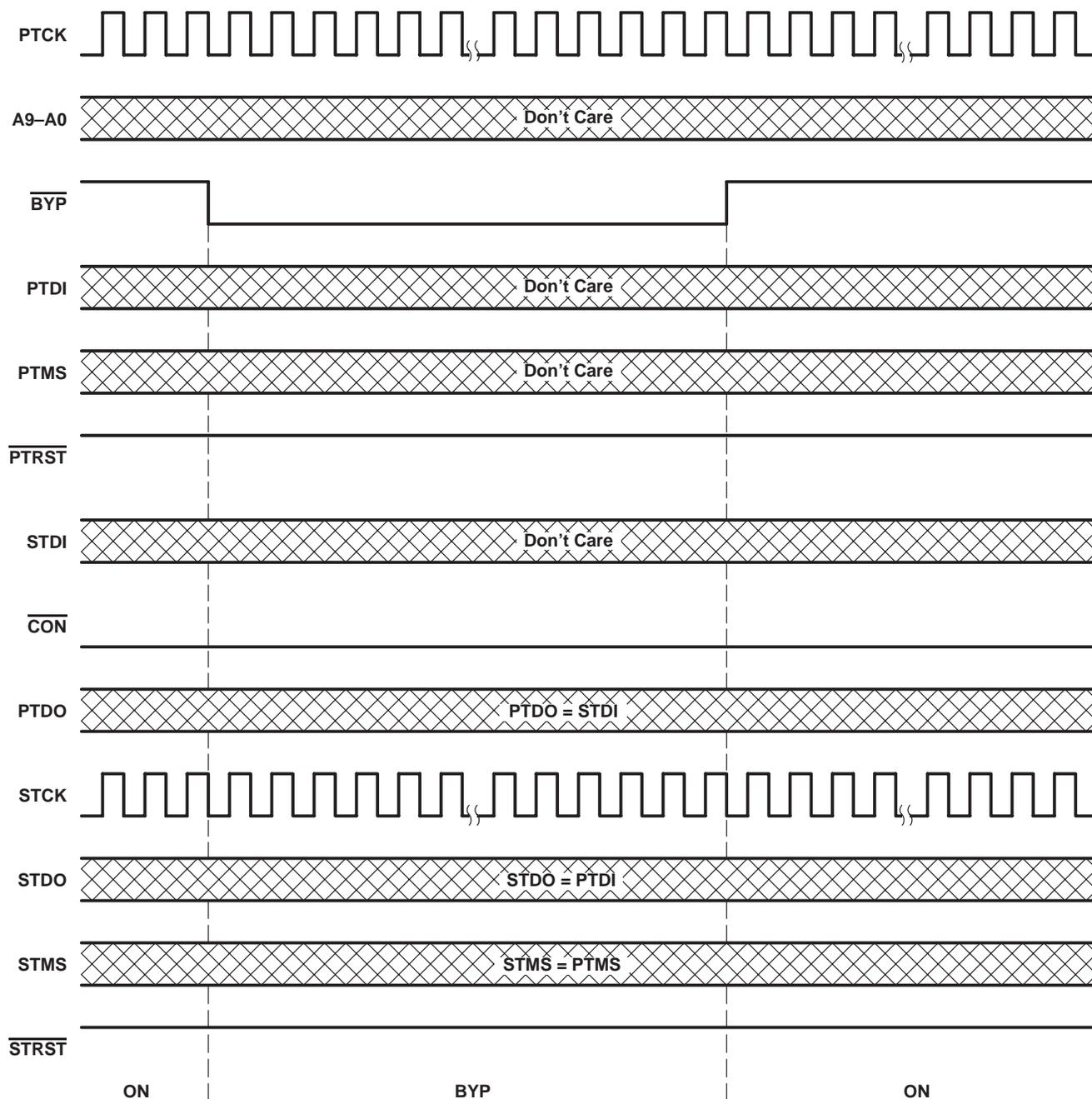
Figure 19. Protocol-Bypass Timing, Prior Connect Status = ON
