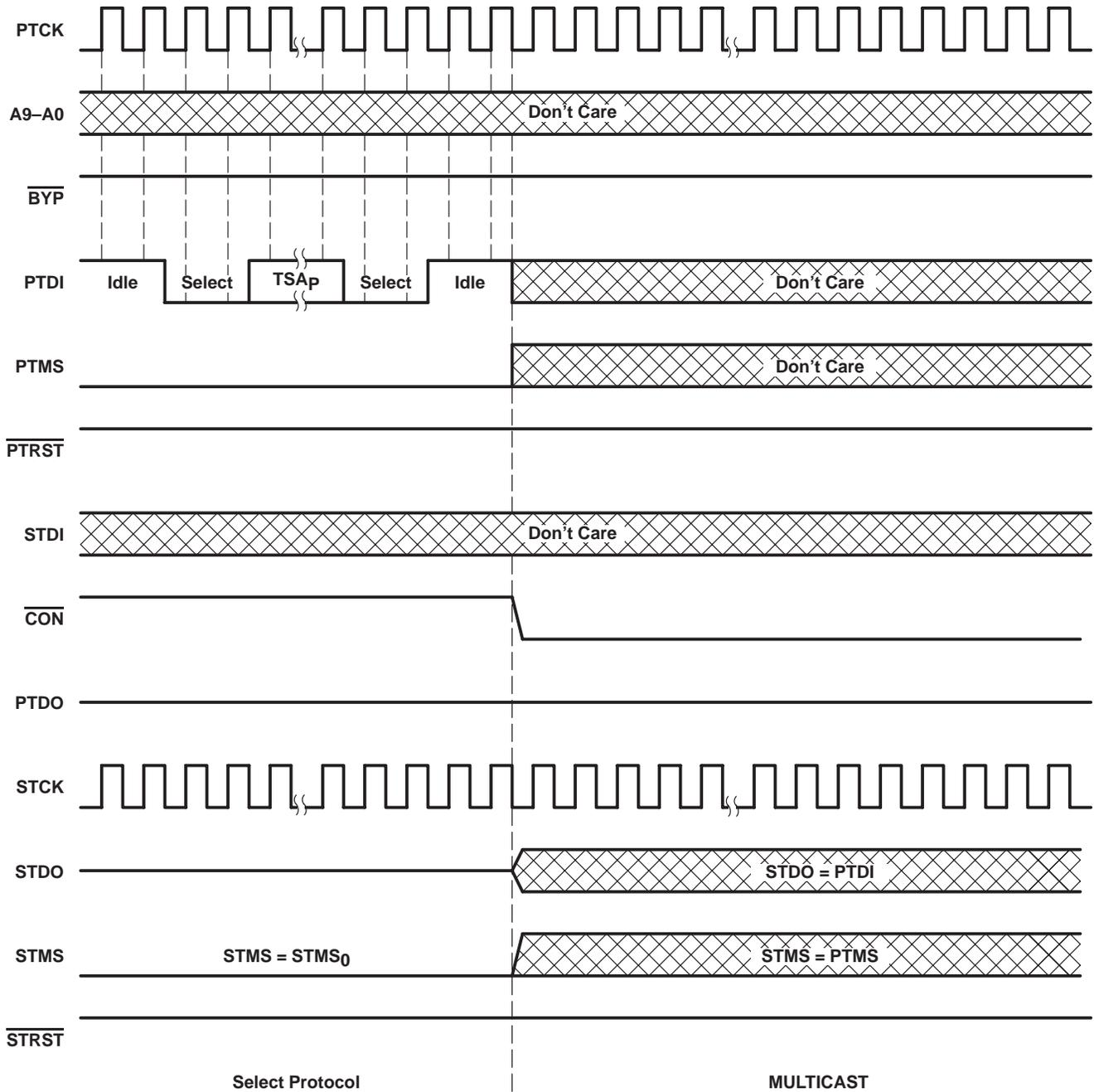
Figure 15. Shadow-Protocol Timing,
