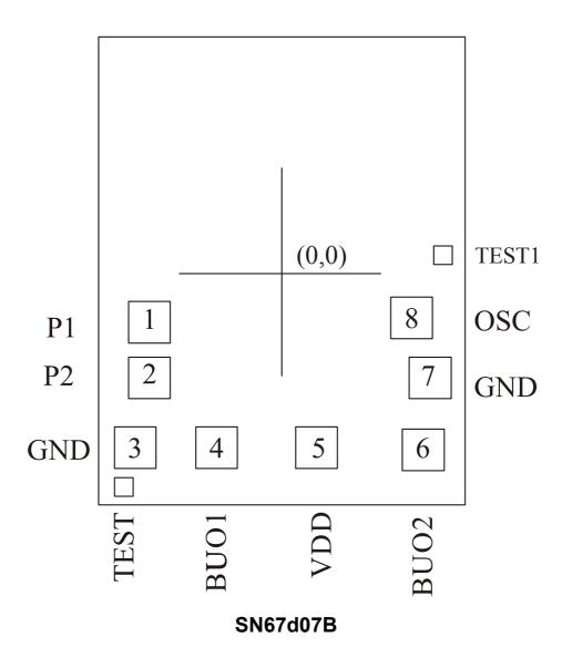
Note: The substrate MUST be connected to Vss in PCB layout.
