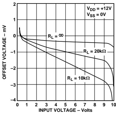
Figure 7. Offset Voltage vs. Input Voltage ( $T_A = +25^\circ\text{C}$ )
