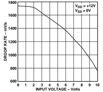
Figure 3. Droop Rate vs. Input Voltage ( $T_A = +125^\circ\text{C}$ )
