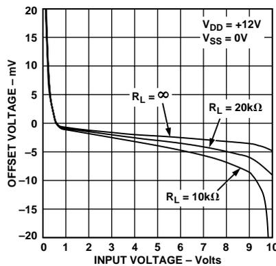
Figure 8. Offset Voltage vs. Input Voltage ( $T_A = +125^\circ\text{C}$ )
