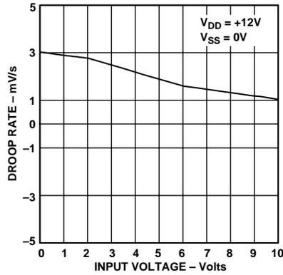
Figure 2. Droop Rate vs. Input Voltage ( $T_A = +25^\circ\text{C}$ )
