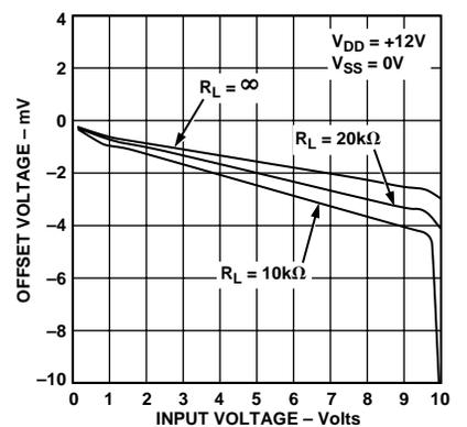
Figure 9. Offset Voltage vs. Input Voltage ( $T_A = -55^\circ\text{C}$ )
