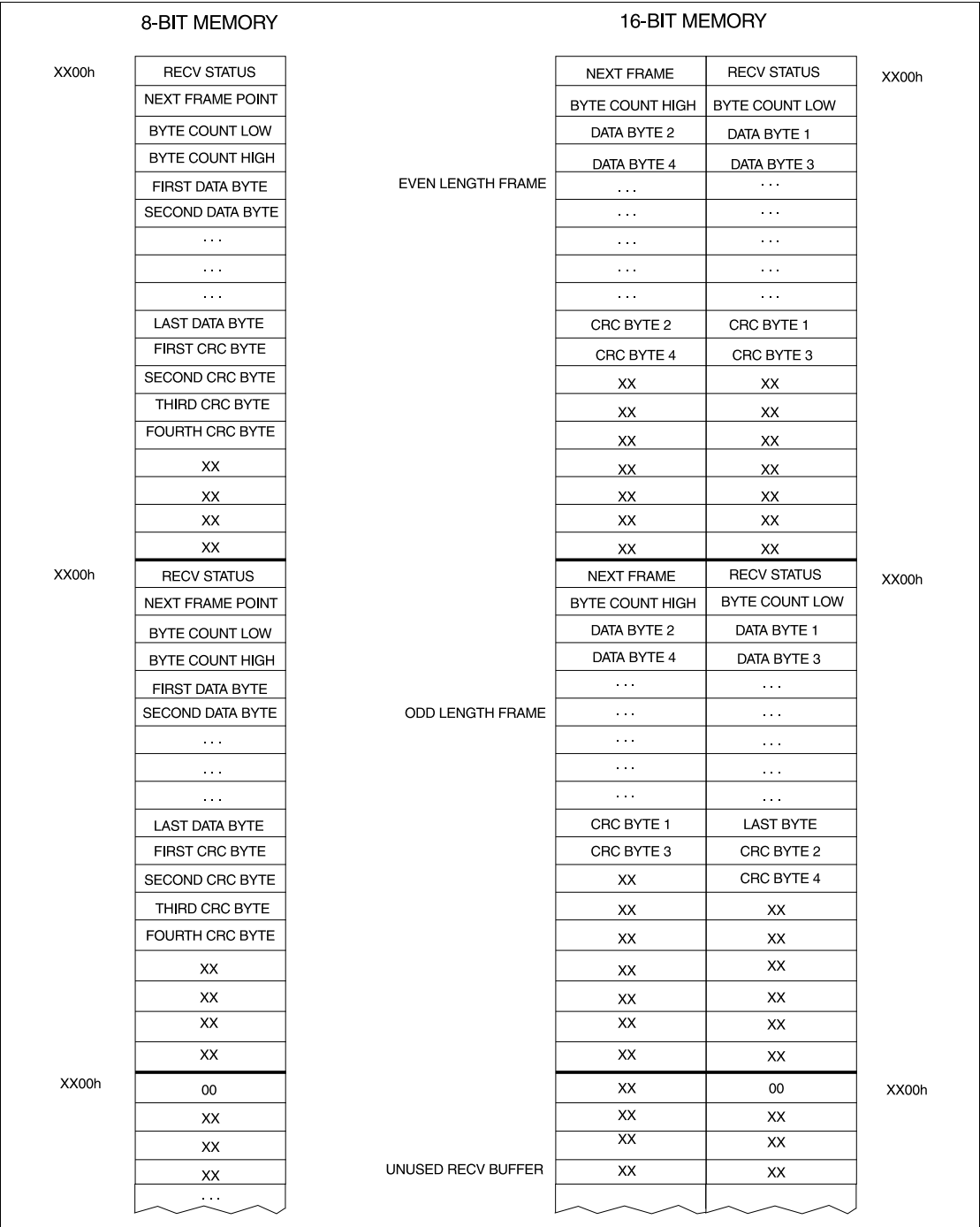
FIGURE 8-2. RECEIVER BUFFER FORMAT
