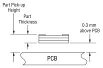
Recommended pick-up height: The bottom of the device should be 0.3 mm above the PCB.
