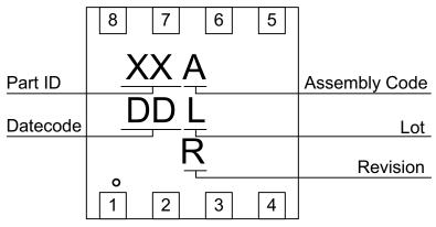
XX - Part ID Field: identifies the specific device configuration A - Assembly Code Field: Assembly Location of the device.
