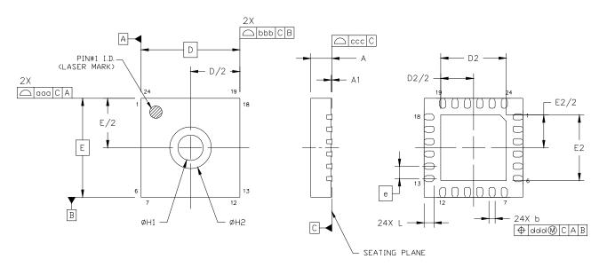
Figure 8. 24-Pin Quad Flat No Lead (QFN)
