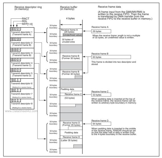
Figure 23.6 Relationship between Receive Descriptor and Receive Buffer
