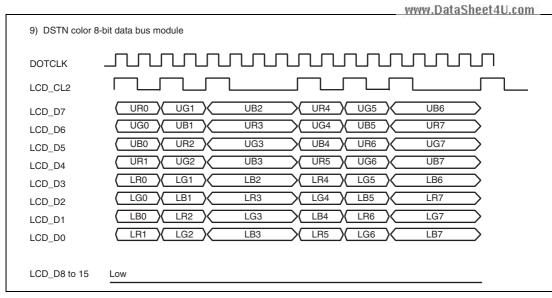
Figure 37.18 Clock and LCD Data Signal Example (DSTN Color 8-Bit Data Bus Module)
