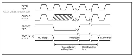
Figure 17.5 STATUS Output by Reset input during Sleep Mode
