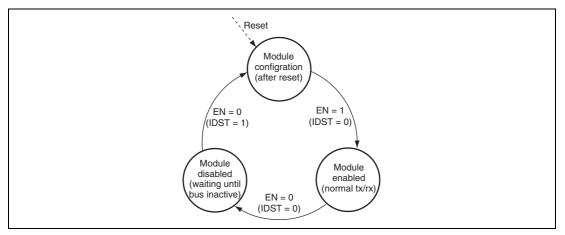
Figure 34.18 Transition Diagram between Operation Modes
