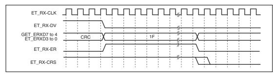
Figure 23.27 GMII/MII Fame Receive Timing (Error with Carrier Extension)
