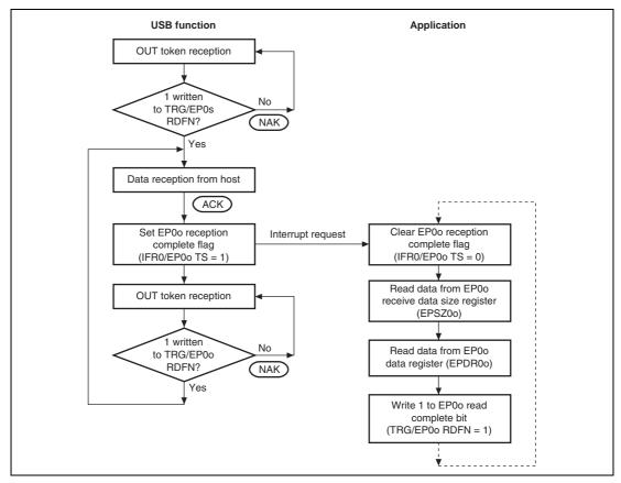
www.DataSheet4U.com Figure 36.7 Data Stage (Control-Out) Operation
