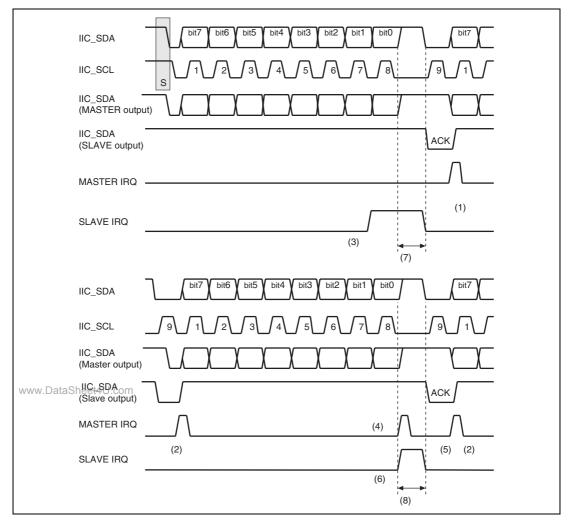
Figure 26.9 Data Transmit Mode Operation Timing
