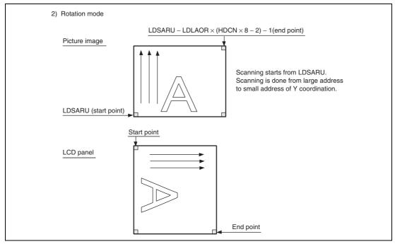
Figure 37.9 Operation for Hardware Rotation (Rotation Mode)
