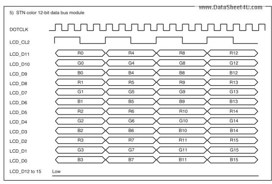
Figure 37.14 Clock and LCD Data Signal Example (STN Color 12-Bit Data Bus Module)
