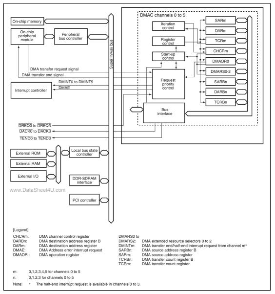
Figure 14.1 Block Diagram of DMAC
