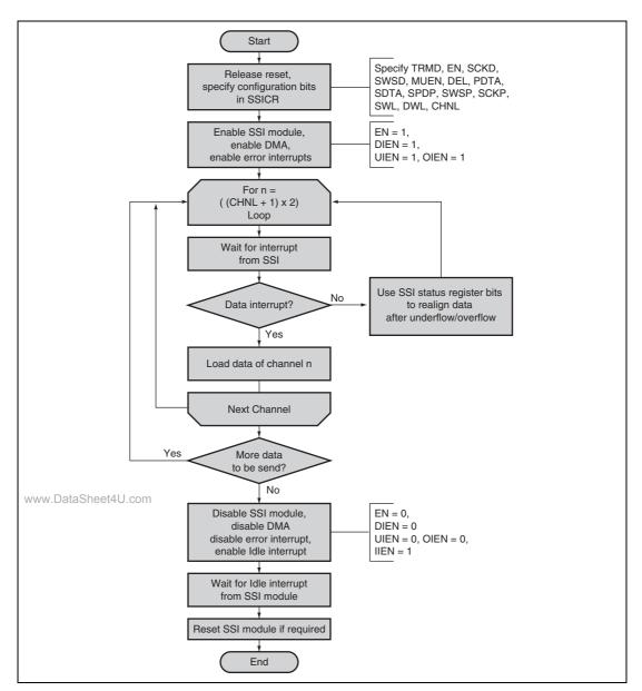
Figure 34.20 Transmission using Interrupt Data Flow Control
