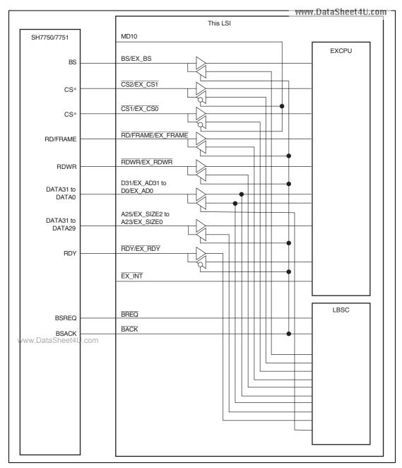
Figure 15.4 Configuration of Connection with External CPU
