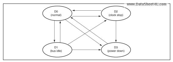
Figure 13.16 PCI Local Bus Power Down State Transition
