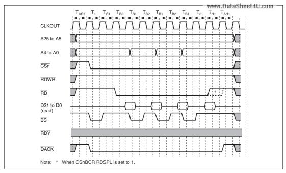
Figure 11.13 Burst ROM Wait Access Timing
