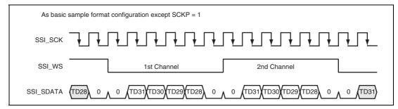
Figure 34.10 Inverted Clock
