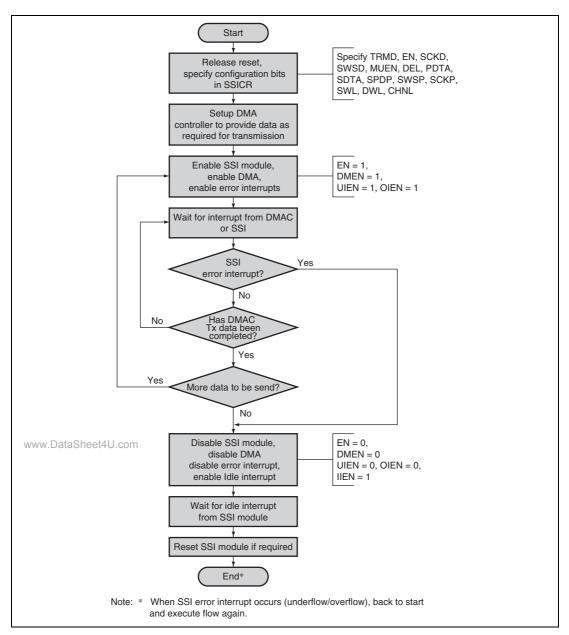
Figure 34.19 Transmission Using DMA Controller
