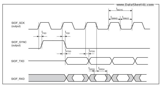
Figure 43.61 SIOF Transmission/Reception Timing (Master Mode 1, Sampling at the Falling Edge)
