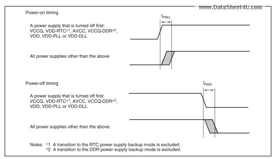
Figure 43.1 Power-On and Power-Off Timing
