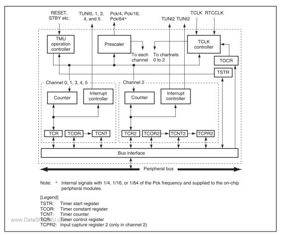
Figure 19.1 Block Diagram of TMU
