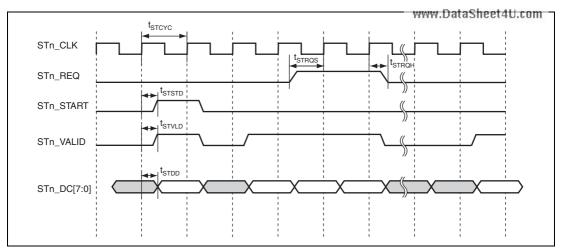
Figure 43.53 STIF Clock Valid Transmit Timing
