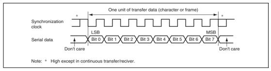
Figure 28.12 Data Format in Clocked Synchronous Communication
