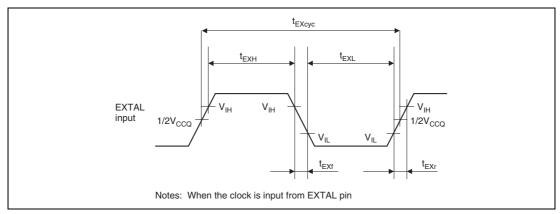
Figure 43.2 EXTAL Clock Input Timing
