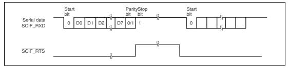
Figure 27.14 Sample Operation Using Modem Control (SCIFO\_RTS)
