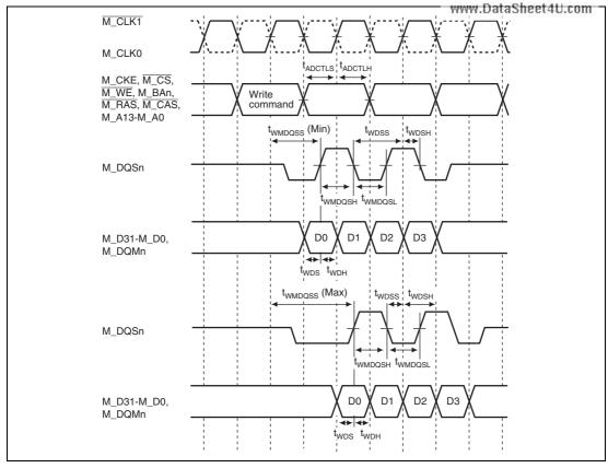
Figure 43.30 Write Timing of DDR-SDRAM (2 Burst Write)
