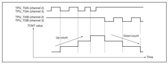
Figure 20.17 Example of Phase Counting Mode 3 Operation
