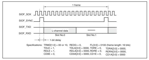
Figure 29.14 Transmit and Receive Timing (8-Bit Monaural Data (2))
