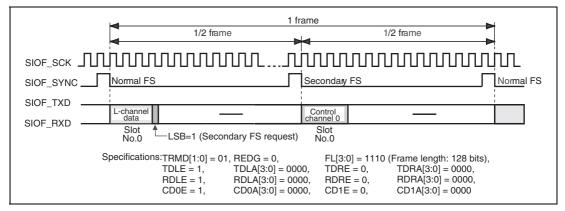
Figure 29.8 Control Data Interface (Secondary FS)
