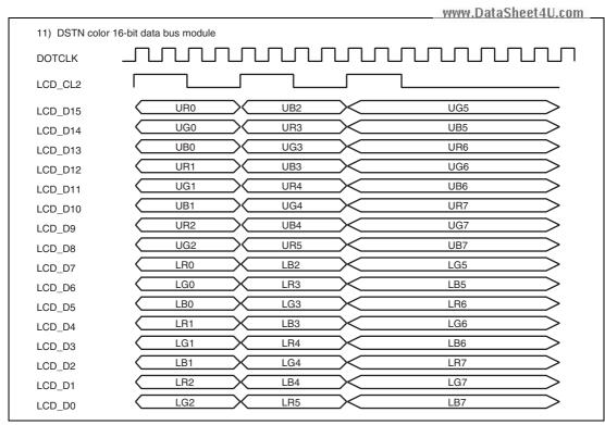
Figure 37.20 Clock and LCD Data Signal Example (DSTN Color 16-Bit Data Bus Module)
