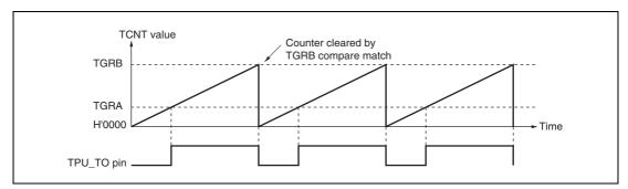
Figure 20.12 Example of PWM Mode Operation (1)
