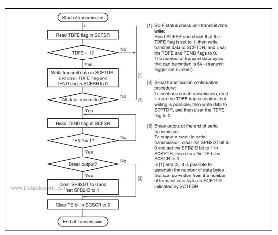
Figure 27.9 Sample Serial Transmission Flowchart
