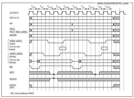
Figure 11.20 Dynamic Bus Sizing Timing for PCMCIA I/O Card Interface
