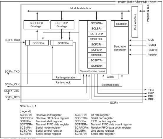
Figure 27.1 Block Diagram of SCIF
