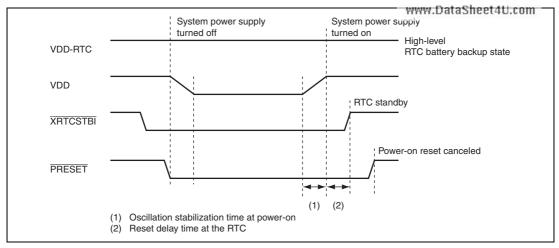
Figure 18.3 Sequence for Turning VDD Power Supply (1.2 V) On/Off
