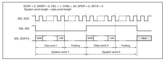
Figure 34.4 Sony Format (with Serial Data First, Followed by Padding Bits)
