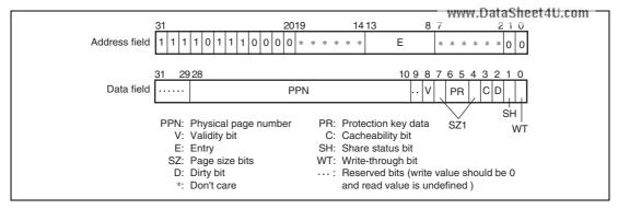
Figure 6.15 Memory-Mapped UTLB Data Array
