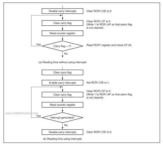
Figure 22.3 Examples of Time Reading Procedures
