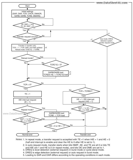
Figure 14.11 DMA Transfer Flowchart
