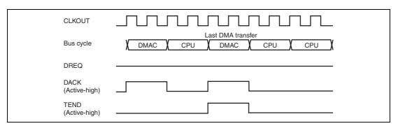
Figure 14.17 DMA Transfer End Signal (Cycle Steal Mode Level Detection)
