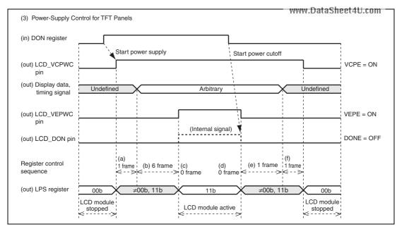
Figure 37.6 Power-Supply Control Sequence and States of the LCD Module
