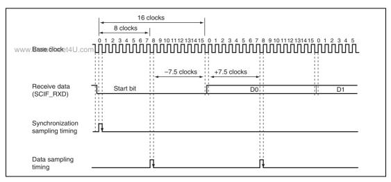
Figure 27.22 Receive Data Sampling Timing in Asynchronous Mode
