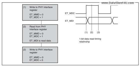
Figure 23.35 1-Bit Data Read Flowchart
