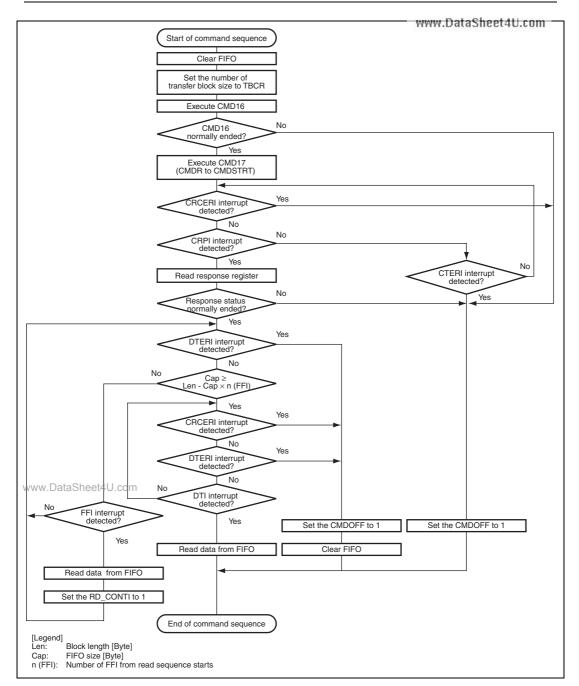
Figure 31.10 Example of Operational Flow for Commands with Read Data (Single Block Transfer)
