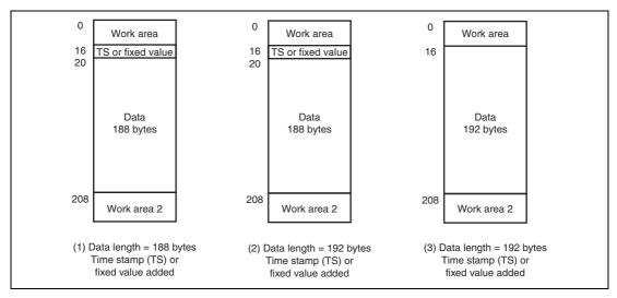
Figure 25.2 Transmit/Receive Data Structure in External Memory (with 16-Byte Work www.DataSheet4U.com Area)
