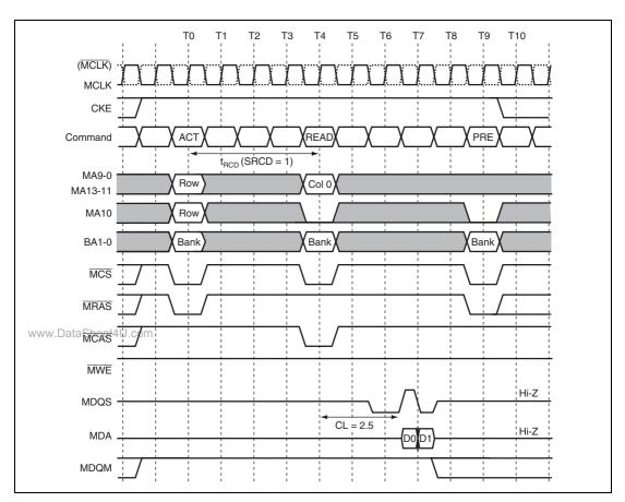
Figure 12.5 Basic DDRIF Timing (1 Burst Read: 1, 2, 4, or 8 Bytes; Without Auto-Precharge)
