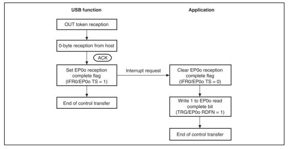
Figure 36.8 Status Stage (Control-In) Operation
