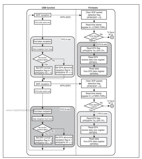
Figure 36.13 EP4 Isochronous-Out Transfer Operation (SOF is Normal)
