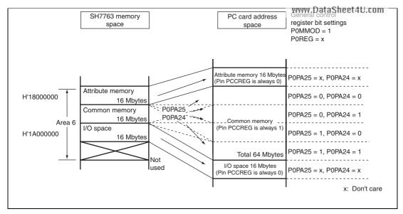
Figure 32.3 Continuous 16-Mbyte Area Mode (Area 6)
