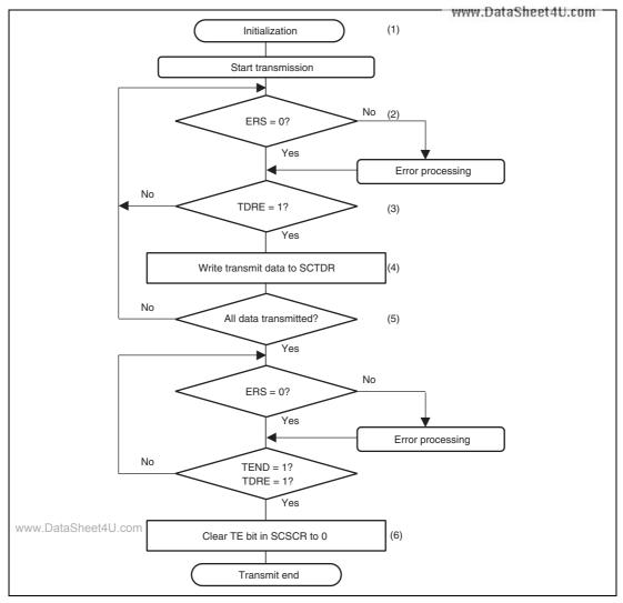
Figure 30.5 Example of Transmit Processing
