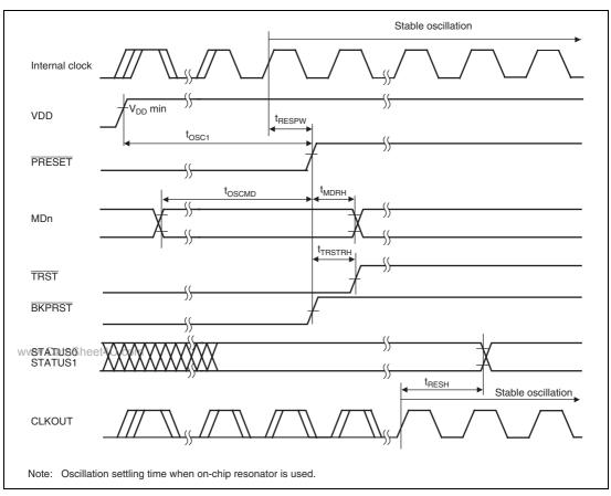
Figure 43.5 Power-On Oscillation Settling Time
