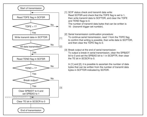
Figure 28.7 Sample Serial Transmission Flowchart
