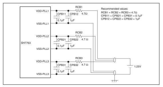
Figure 16.3 Notes on Using PLL or DLL Oscillator Circuit
