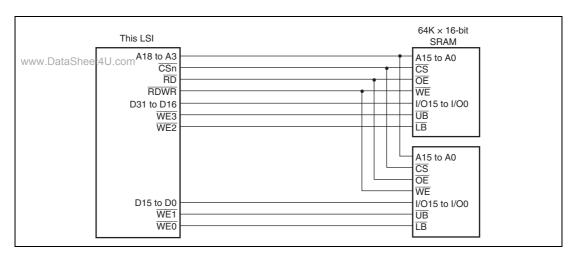
Figure 11.34 Example of 32-Bit Data-Width Byte-Control SRAM
