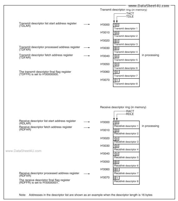
Figure 23.7 Relationship between Transmit/Receive Descriptor and Descriptor Pointing Registers
