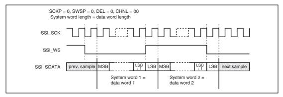
Figure 34.2 Philips Format (with no Padding)
