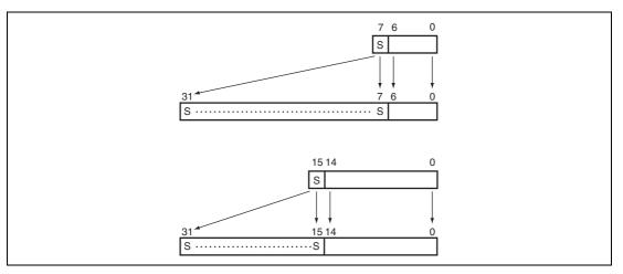
Figure 2.6 Formats of Byte Data and Word Data in Register
