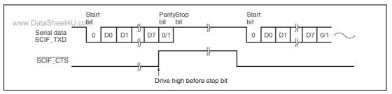
Figure 27.11 Sample Operation Using Modem Control (SCIF\_CTS)
