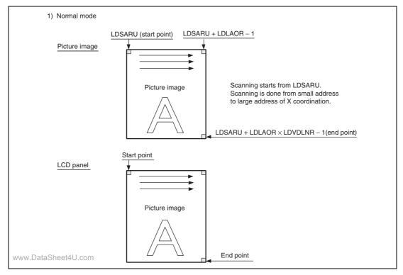
Figure 37.8 Operation for Hardware Rotation (Normal Mode)
