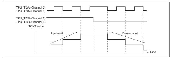
Figure 20.16 Example of Phase Counting Mode 2 Operation
