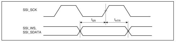
Figure 43.76 SSI Receive Timing (1)
