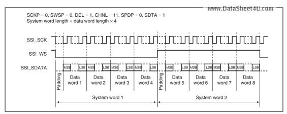
Figure 34.8 Multichannel Format (4 Channels, with Padding Bits First, Followed by Serial Data, with Padding)
