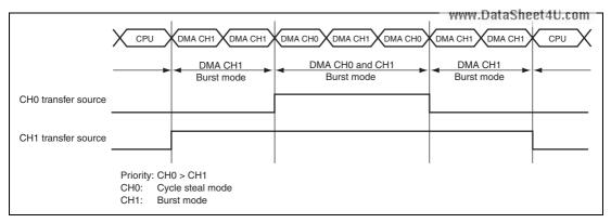
Figure 14.10 Bus State when Multiple Channels are Operating
