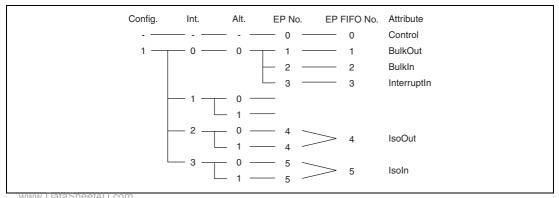
Figure 36.2 Example of Endpoint Configuration
