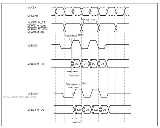
Figure 43.29 Read Timing of DDR-SDRAM (2 Burst Read)
