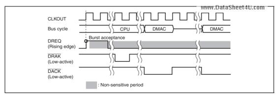
Figure 14.15 Example of DREQ Input Detection in Burst Mode Edge Detection
