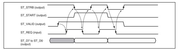
Figure 25.6 Strobe Transmission Timing
