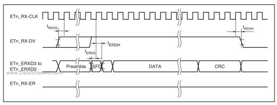
Figure 43.42 MII Receive Timing (normal operation)
