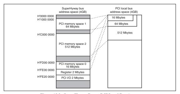
Figure 13.2 SuperHyway Bus to PCI Local Bus Access
