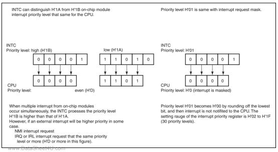
Figure 9.3 On-chip Module Interrupt Priority
