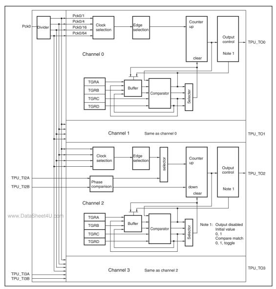
Figure 20.1 Block Diagram of TPU
