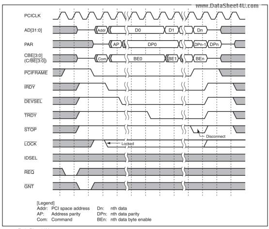
www.Data Figure 13.24 Target Memory Write Cycle in Host Bus Bridge Mode (Burst)
