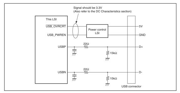
Figure 35.2 Connection Example of External Circuit
