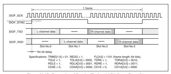
Figure 29.17 Transmit and Receive Timing (16-Bit Stereo Data (2))
