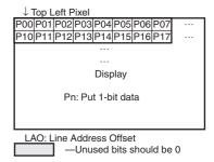
2. Packed 2bpp (Pixel Alignment in Byte is Big Endian) [Windows CE Recommended Format]
