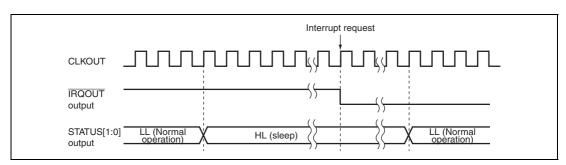
Figure 18.4 STATUS Output when an Interrupt Occurs in Sleep Mode
