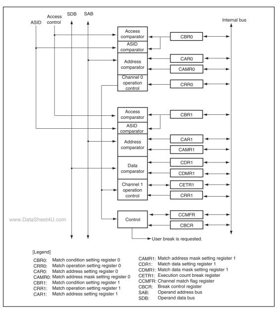
Figure 41.1 Block Diagram of UBC
