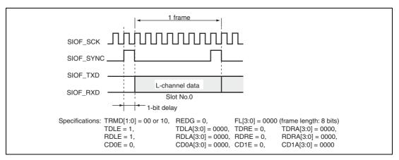
Figure 29.13 Transmit and Receive Timing (8-Bit Monaural Data (1))
