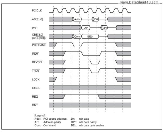
$Figure\ 13.18\ Master\ Read\ Cycle\ in\ Host\ Bus\ Bridge\ Mode\ (Single)$
