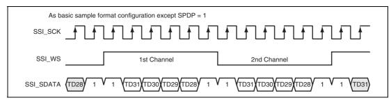
Figure 34.12 Inverted Padding Polarity
