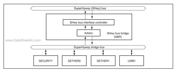
Figure 10.1 SBR Block Diagram
