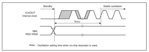
Figure 43.7 Oscillation Settling Time on Return from Standby NMI or IRQ
