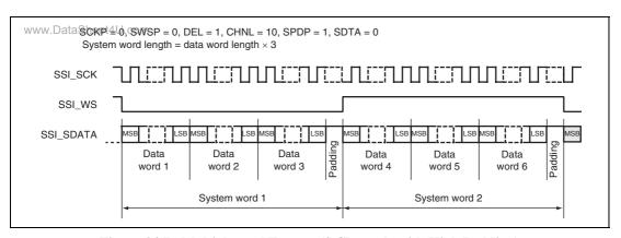
Figure 34.7 Multichannel Format (3 Channels with High Padding)
