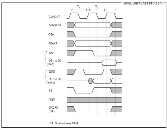
Figure 11.4 Basic Timing of SRAM Interface
