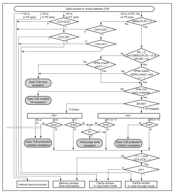
Figure 6.9 Flowchart of Memory Access Using UTLB
