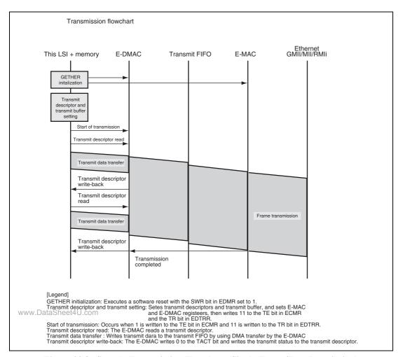
Figure 23.8 Sample Transmission Flowchart (Single-Frame/Two-Description)
