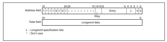
Figure 7.8 Memory-Mapped OC Data Array
