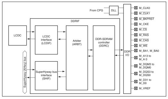
Figure 12.1 DDRIF Block Diagram
