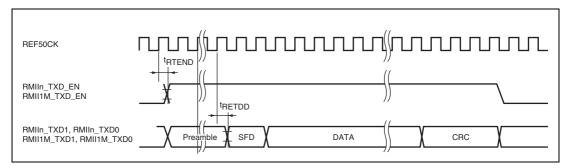
Figure 43.49 RMII Transmit Timing
