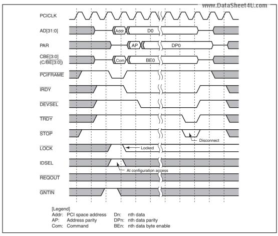
www.DataSheet4U.cFigure 13.22 Target Write Cycle in Normal Mode (Single)
