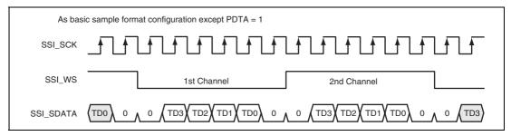
Figure 34.16 Parallel Right Aligned with Delay
