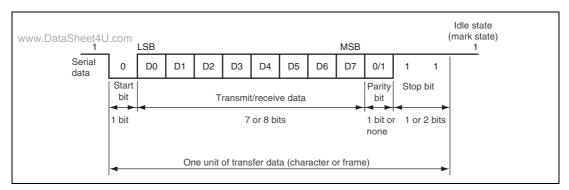
Figure 28.5 Data Format in Asynchronous Communication (Example with 8-Bit Data, Parity, and Two Stop Bits)
