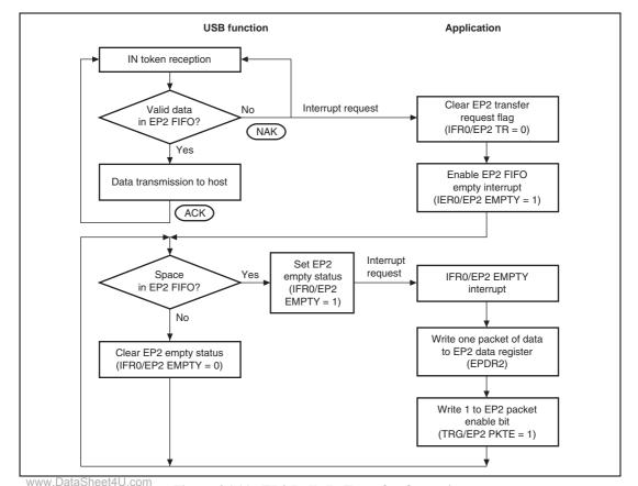
Figure 36.11 EP2 Bulk-In Transfer Operation
