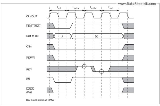
Figure 11.25 MPX Interface Timing 4 (Single Write Cycle, IW = 1, One External Wait Inserted)
