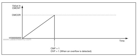
Figure 21.2 Counter Operation (One-Shot Operation)
