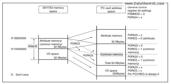
Figure 32.2 Continuous 32-Mbyte Area Mode
