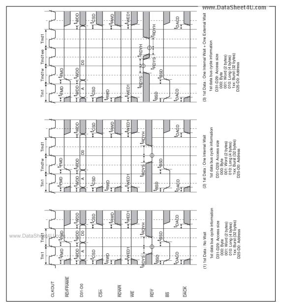
Figure 43.23 MPX Basic Bus Cycle: Write
