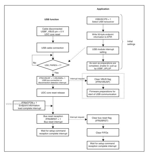
Figure 36.3 Cable Connection Operation
