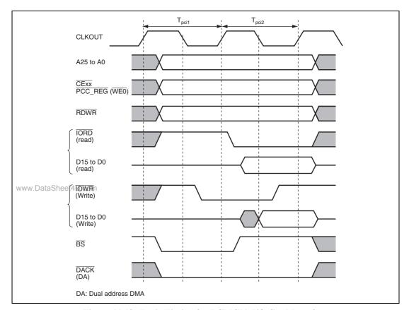
Figure 11.18 Basic Timing for PCMCIA I/O Card Interface
