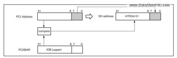
Figure 13.11 PCI Local Bus to SuperHyway Bus Address Translation (PCIC I/O Space)
