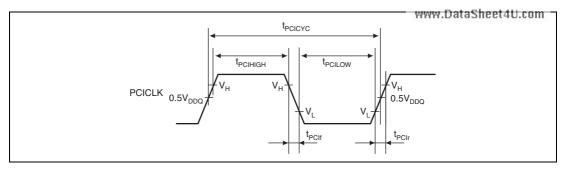
Figure 43.34 PCI Clock Input Timing
