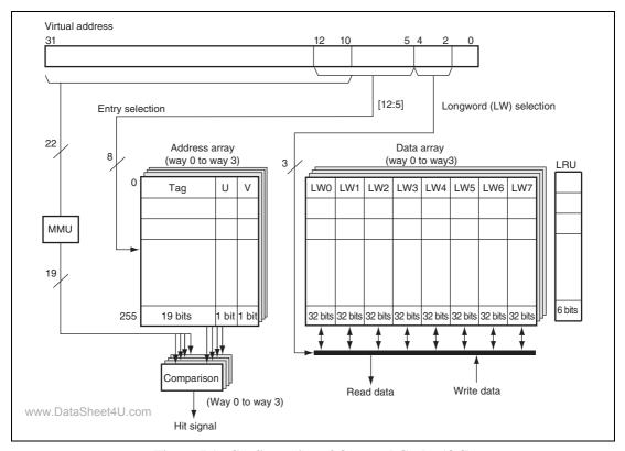
Figure 7.1 Configuration of Operand Cache (OC)
