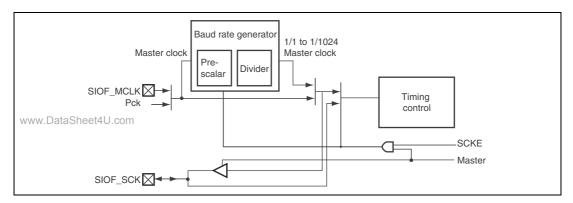
Figure 29.2 Serial Clock Supply
