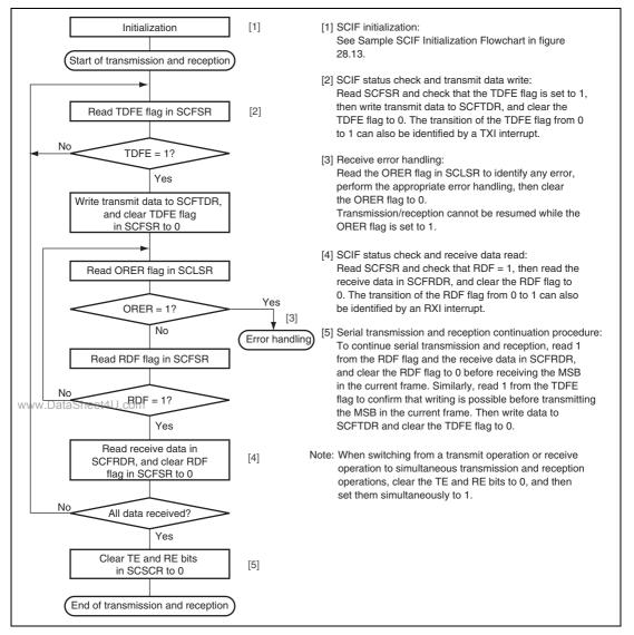
Figure 28.19 Sample Simultaneous Serial Transmission and Reception Flowchart
