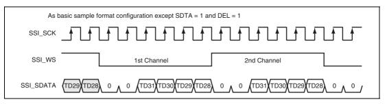
Figure 34.14 Padding Bits First, Followed by Serial Data, without Delay
