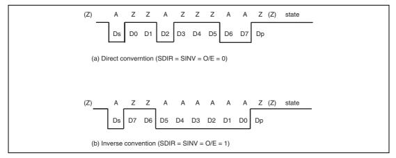
Figure 30.3 Examples of Start Character Waveforms
