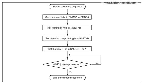
Figure 31.3 Example of Operational Flow for Commands
