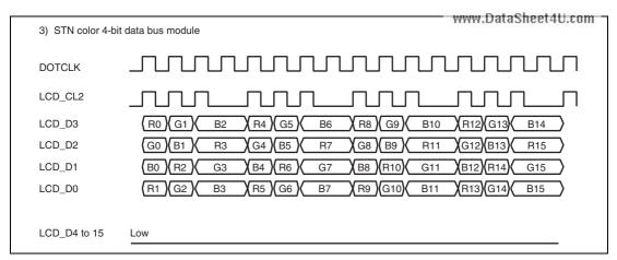
Figure 37.12 Clock and LCD Data Signal Example (STN Color 4-Bit Data Bus Module)
