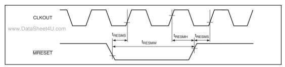
Figure 43.8 Reset Input Timing
