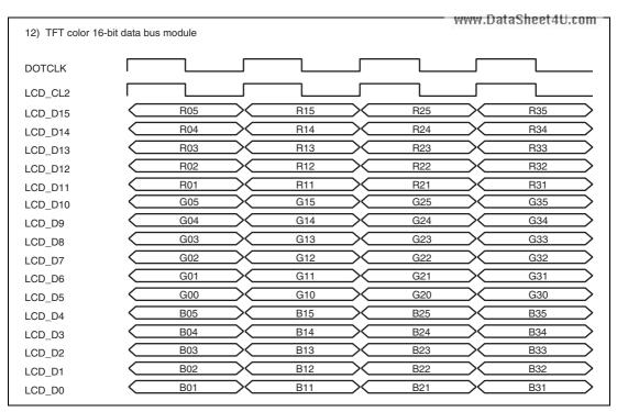
Figure 37.21 Clock and LCD Data Signal Example (TFT Color 16-Bit Data Bus Module)
