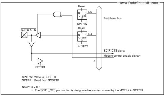
Figure 27.3  $\overline{SCIFn}$  Pin (n = 0, 1)
