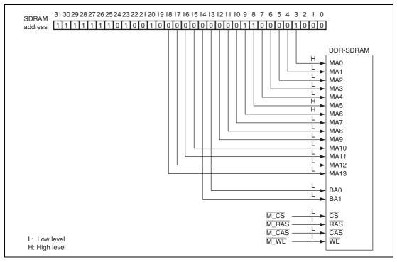
Figure 12.3 Relationship between Write Values in SDMR and Output Signals to Memory Pins
