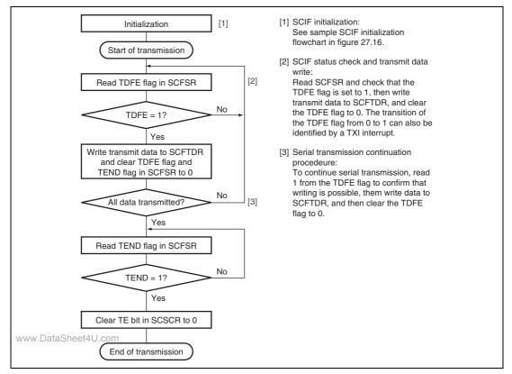
Figure 27.17 Sample Serial Transmission Flowchart
