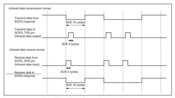
Figure 28.21 Infrared Communication Data Format
