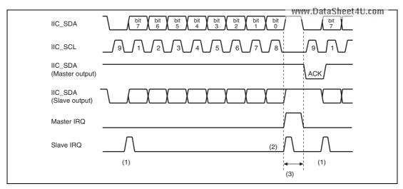
Figure 26.10 Data Receive Mode Operation Timing
