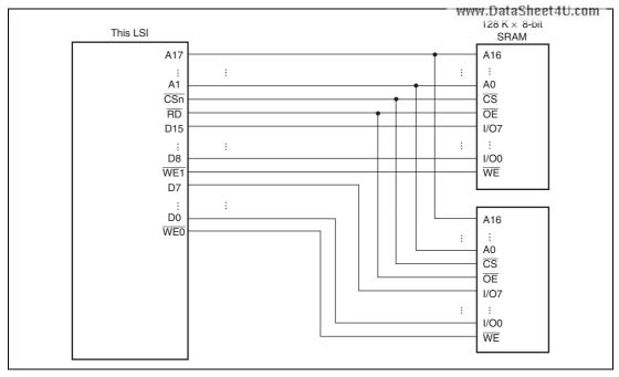
Figure 11.6 Example of 16-Bit Data-Width SRAM Connection
