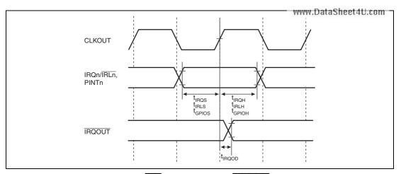
Figure 43.32 IRQ/IRL, PINT Input and IRQOUT Output Timing
