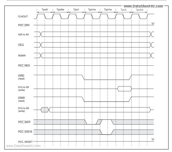
Figure 32.8 PCMCIA I/O Card Interface Wait Timing
