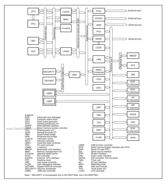
Figure 1.1 SH7763 Block Diagram
