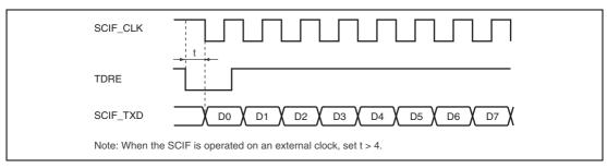
Figure 27.23 Example of Synchronization Clock Transfer by DMAC
