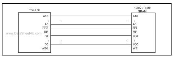
Figure 11.7 Example of 8-Bit Data-Width SRAM Connection
