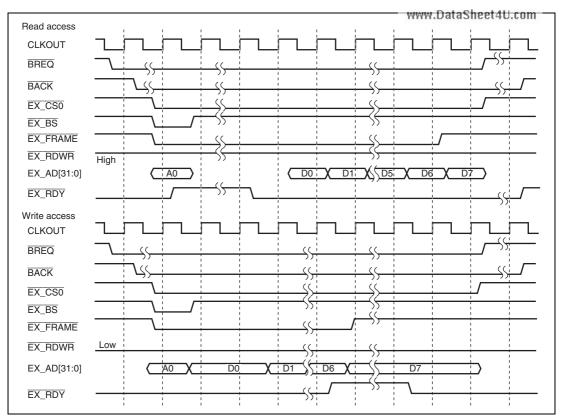
Figure 15.3 External CPU Access (Burst Access)
