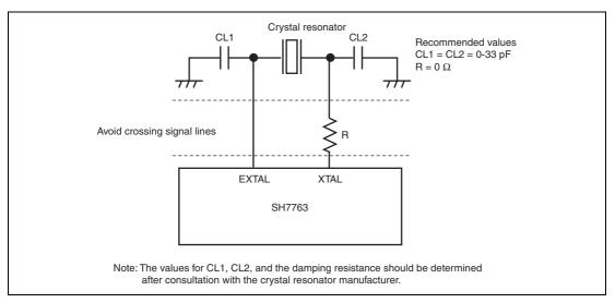
Figure 16.2 Notes on Using Crystal Resonator
