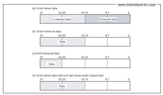
Figure 29.5 Transmit/Receive Data Bit Alignment
