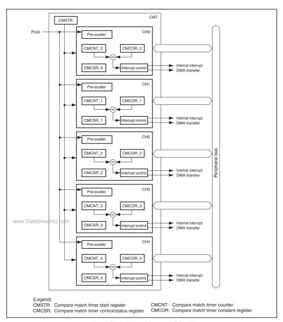
Figure 21.1 Block Diagram of CMT
