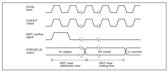
Figure 17.9 STATUS Output by Watchdog timer overflow Manual Reset during Sleep Mode
