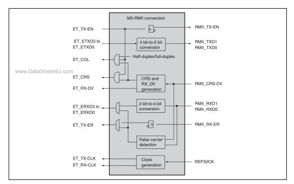
Figure 23.37 MII-RMll Conversion Circuit
