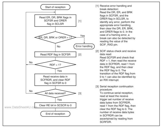
Figure 27.12 Sample Serial Reception Flowchart (1)
