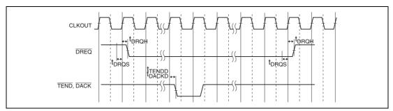
Figure 43.37 DREQ, TEND, and DACK Timing
