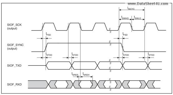
Figure 43.63 SIOF Transmission/Reception Timing (Master Mode 2, Sampling at the Falling Edge)
