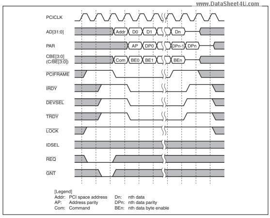
Figure 13.19 Master Write Cycle in Normal Mode (Burst)
