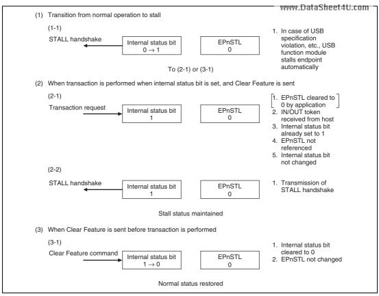
Figure 36.18 Automatic Stall by USB Function Controller
