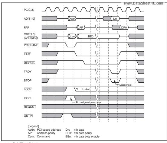
www.DataSheet4U.Figure 13.21 Target Read Cycle in Normal Mode (Single)
