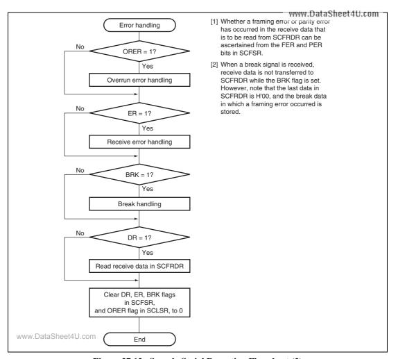
Figure 27.12 Sample Serial Reception Flowchart (2)
