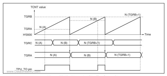
Figure 20.10 Example of Buffer Operation
