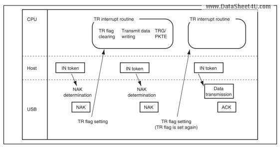
Figure 36.20 Set Timing of TR Interrupt Flag
