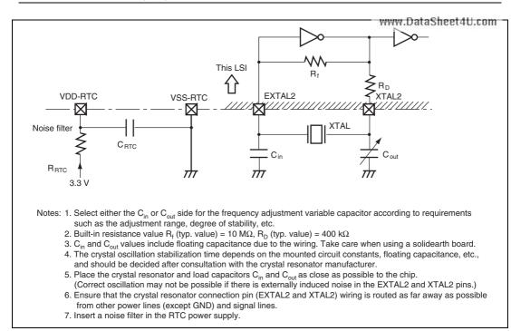
Figure 22.5 Example of Crystal Oscillator Circuit Connection
