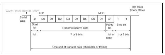
Figure 27.7 Data Format in Asynchronous Communication (Example with 8-Bit Data, Parity, and Two Stop Bits)
