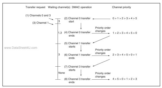
Figure 14.3 Changes in Channel Priority in Round-Robin Mode
