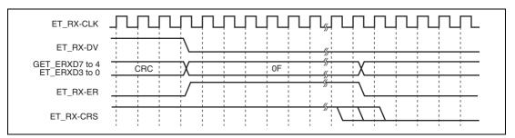
Figure 23.24 GMII/MII Fame Receive Timing (with Carrier Extension)
