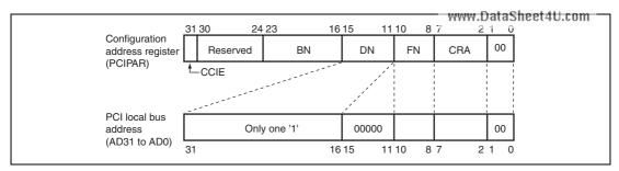
Figure 13.15 Address Generation for Type 0 Configuration Access
