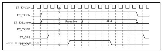
Figure 23.18 MII Frame Transmit Timing (Collision)
