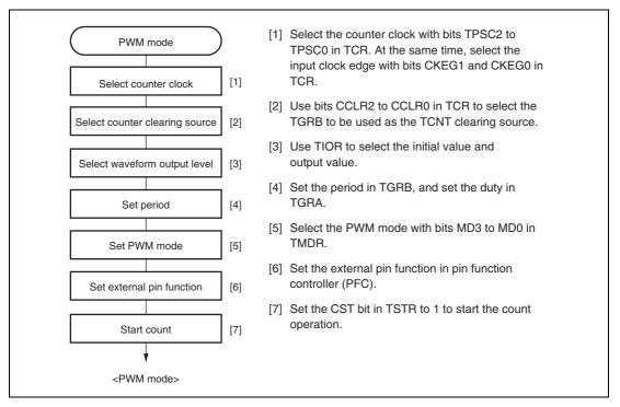
Figure 20.11 Example of PWM Mode Setting Procedure
