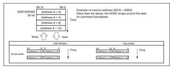
Figure 12.2 Data Alignment in DDR-SDRAM and DDRIF
