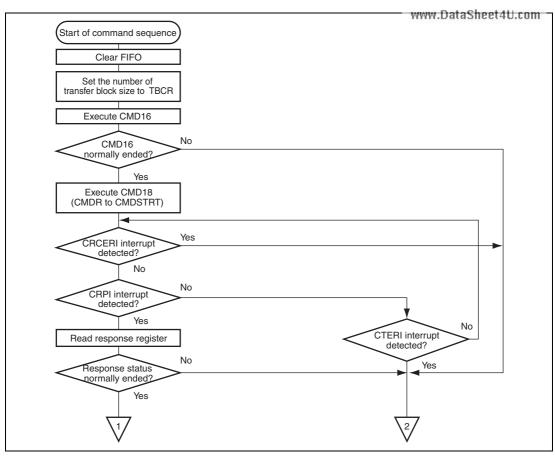
Figure 31.11 (1) Example of Operational Flow for Commands with Read Data www.DataSheet4U.com (Open-ended Multiblock Transfer)
