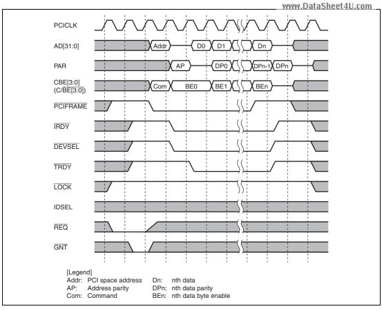
Figure 13.20 Master Read Cycle in Normal Mode (Burst)
