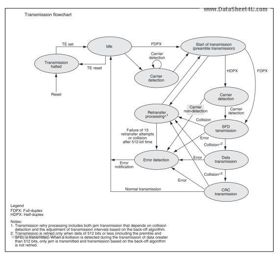
Figure 23.9 E-MAC Transmitter State Transitions
