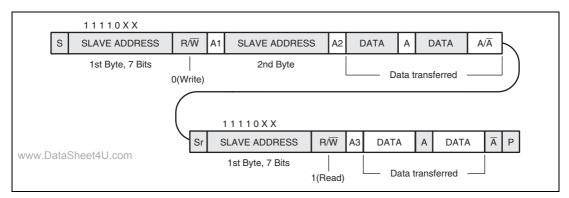
Figure 26.8 10-Bit Address Transmit/Receive Combined Format
