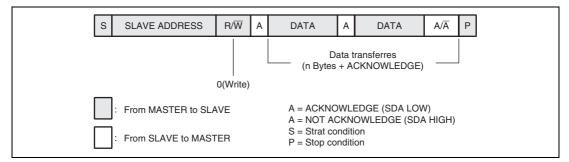
Figure 26.3 Master Data Transmit Format
