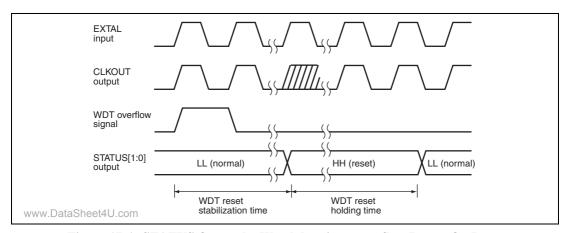
Figure 17.6 STATUS Output by Watchdog timer overflow Power-On Reset during Normal Operation
