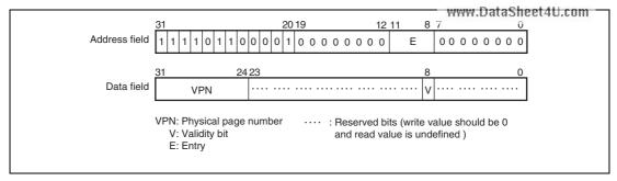
Figure 6.18 Memory-Mapped PMB Address Array
