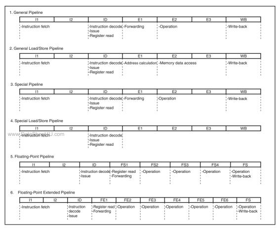
Figure 4.1 Basic Pipelines
