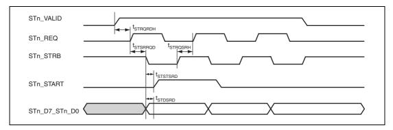
Figure 43.55 STIF Strobe Transmit Timing
