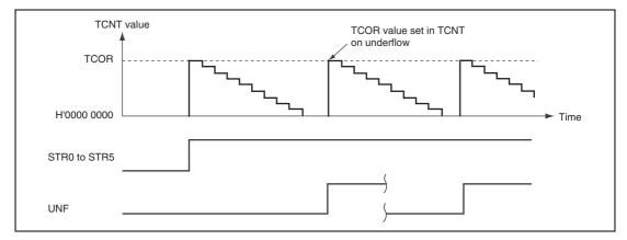
Figure 19.3 TCNT Auto-Reload Operation
