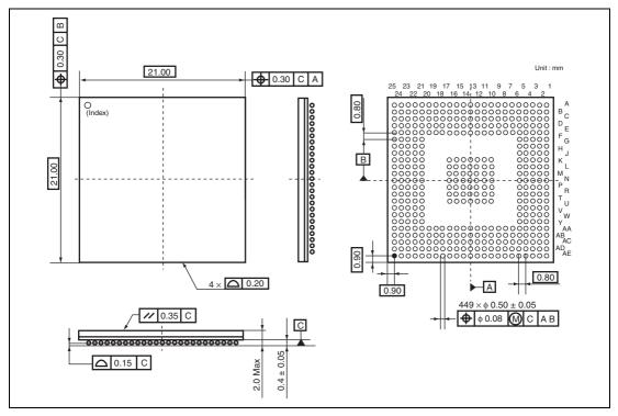
Figure F.1 Package Dimensions (449-Pin)
