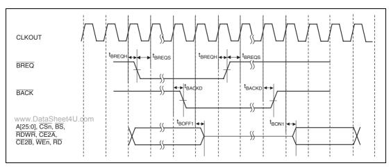
Figure 43.9 Control Signal Timing
