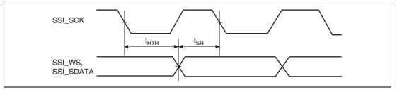
Figure 43.77 SSI Receive Timing (2)
