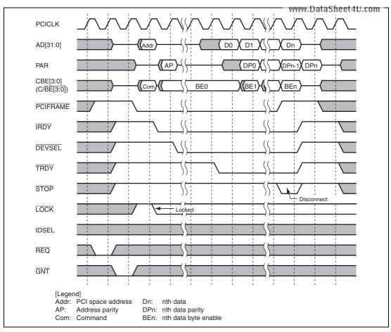
www.DatFiguré 13:23 Target Memory Read Cycle in Host Bus Bridge Mode (Burst)
