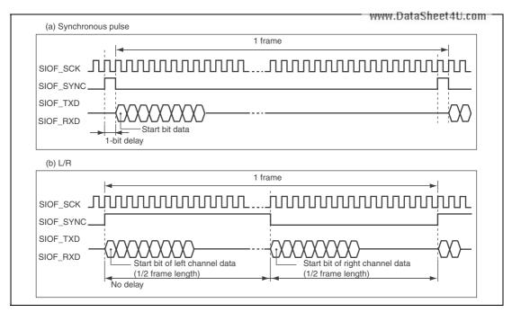
Figure 29.3 Serial Data Synchronization Timing
