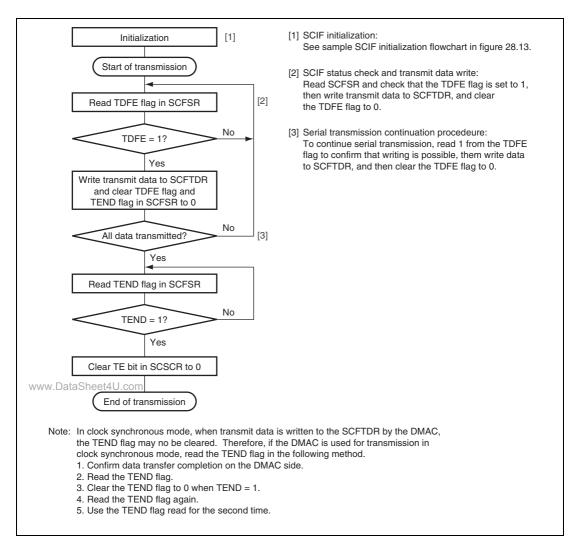
Figure 28.14 Sample Serial Transmission Flowchart
