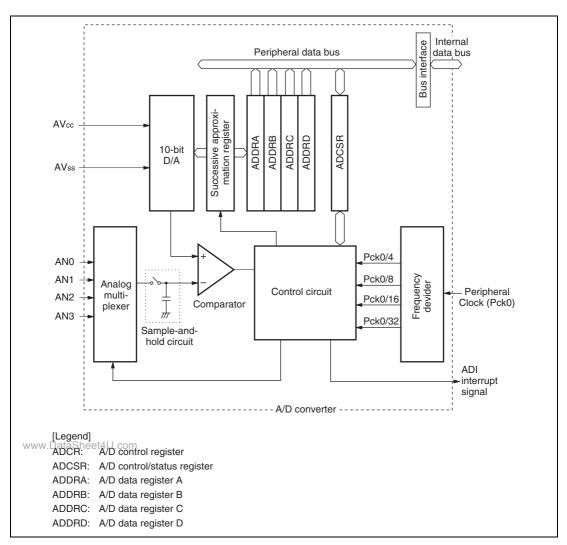
Figure 38.1 Block Diagram of A/D Converter
