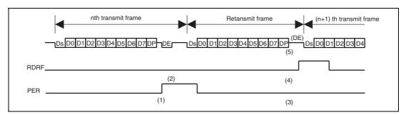
Figure 30.8 Retransmission when Smart Card Interface is in Receive Mode
