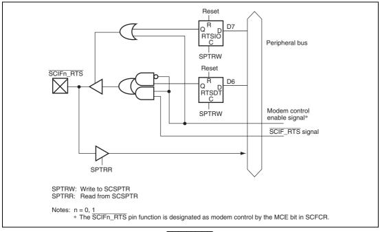
Figure 27.2  $\overline{SCIFn}_{RTS}$  Pin (n = 0, 1)
