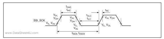
Figure 43.73 SSI Clock Input/Output Timing
