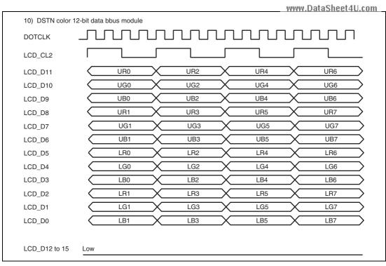
Figure 37.19 Clock and LCD Data Signal Example (DSTN Color 12-Bit Data Bus Module)
