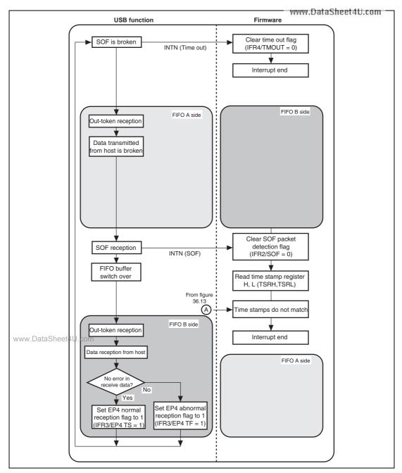
Figure 36.14 EP4 Isochronous-Out Transfer Operation (SOF is Broken)
