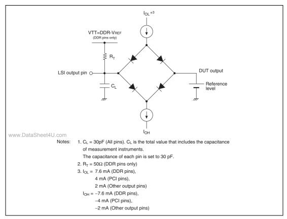
Figure 43.85 Output Load Circuit
