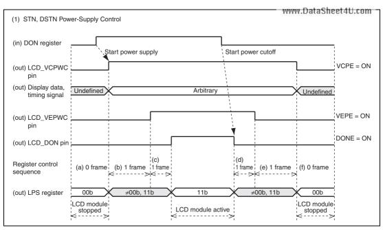
Figure 37.4 Power-Supply Control Sequence and States of the LCD Module
