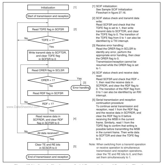
Figure 27.21 Sample Simultaneous Serial Transmission and Reception Flowchart
