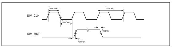
Figure 43.66 SIM Module Signal Timing
