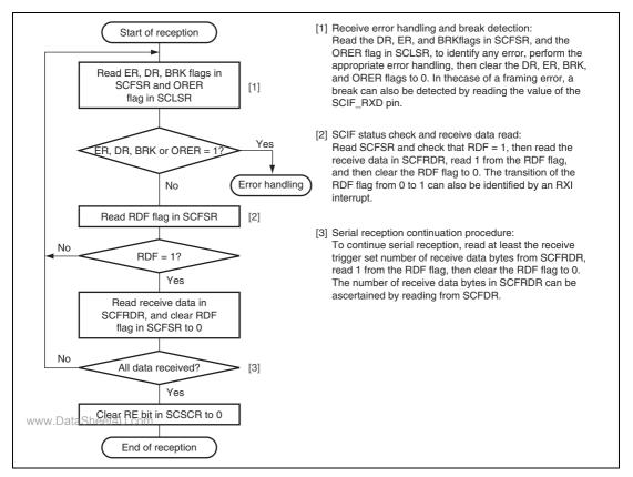
Figure 28.9 Sample Serial Reception Flowchart (1)
