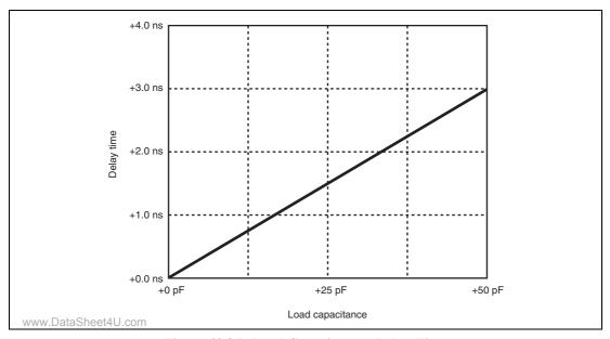
Figure 43.86 Load Capacitance - Delay Time
