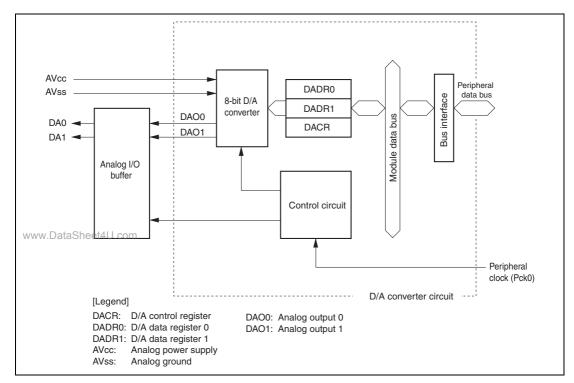
Figure 39.1 Block Diagram of D/A Converter
