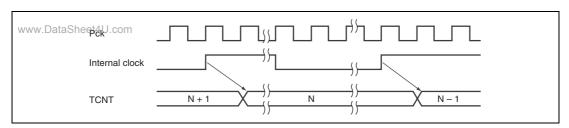
Figure 19.4 Count Timing when Operating on Internal Clock
