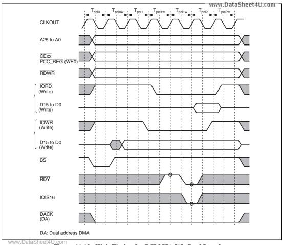
Figure 11.19 Wait Timing for PCMCIA I/O Card Interface
