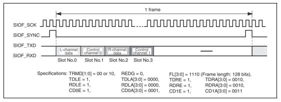
Figure 29.7 Control Data Interface (Slot Position)
