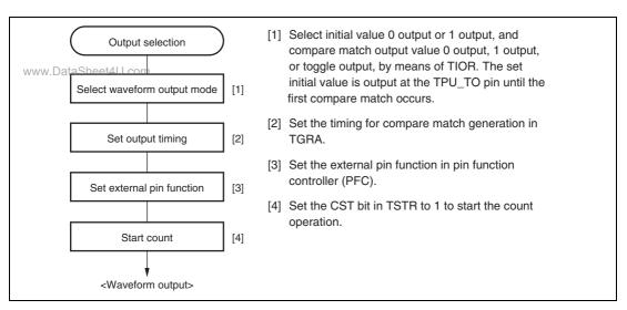
Figure 20.5 Example of Setting Procedure for Waveform Output by Compare Match
