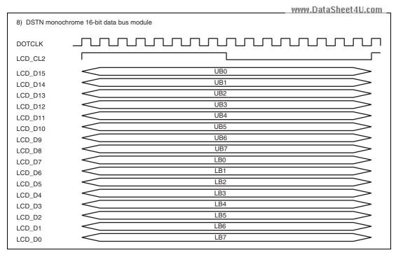
Figure 37.17 Clock and LCD Data Signal Example (DSTN Monochrome 16-Bit Data Bus Module)
