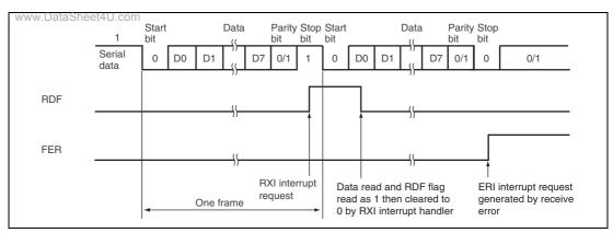
Figure 27.13 Sample SCIF Receive Operation (Example with 8-Bit Data, Parity, One Stop Bit)
