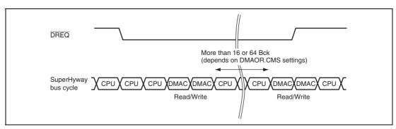
Figure 14.8 Example of DMA Transfer Timing in Cycle Steal Intermittent Mode (DREQ Low Level Detection)
