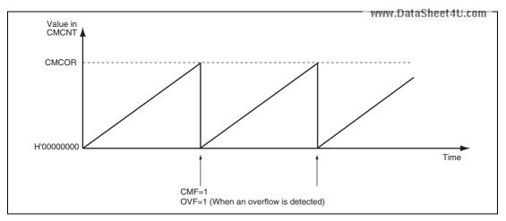
**Figure 21.3 Counter Operation (Free-Running Operation)**
