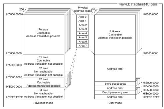
Figure 6.3 Virtual Address Space (AT in MMUCR = 1)
