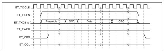
Figure 23.17 MII Frame Transmit Timing (Normal Transmission)
