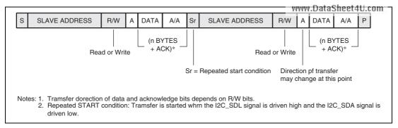
Figure 26.5 Combination Transfer Format of Master Transfer
