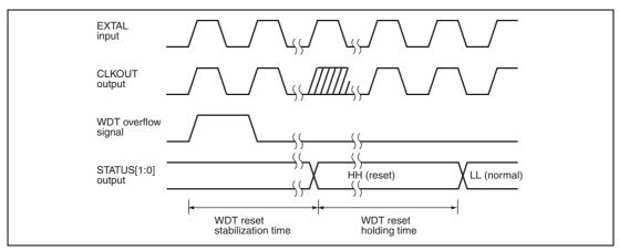
Figure 17.7 STATUS Output by Watchdog timer overflow Power-On Reset during Sleep Mode
