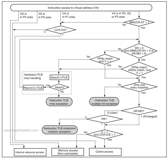
Figure 6.10 Flowchart of Memory Access Using ITLB
