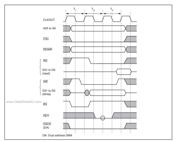
Figure 11.8 SRAM Interface Wait Timing (Software Wait Only)
