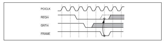
Figure 13.27 Timing Example of Device ( $\overline{REQm}$ ) Not Executing  $\overline{REQ}$  Negation and  $\overline{FRAME}$  Assertion Simultaneously
