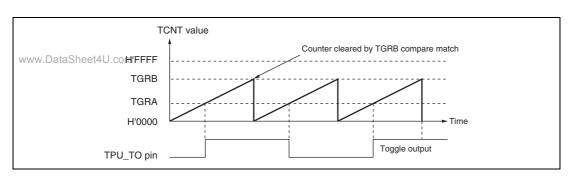
Figure 20.7 Example of Toggle Output Operation
