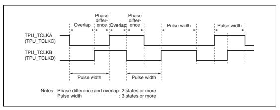
Figure 20.19 Phase Difference, Overlap, and Pulse Width in Phase Counting Mode www.DataSheet4U.com
