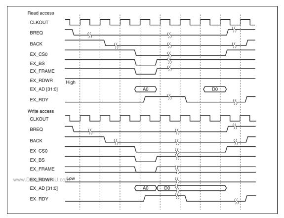
Figure 15.2 External CPU Access (Single Access)
