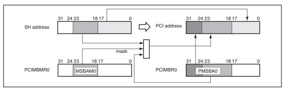
Figure 13.3 SuperHyway Bus to PCI Local Bus Address Translation
