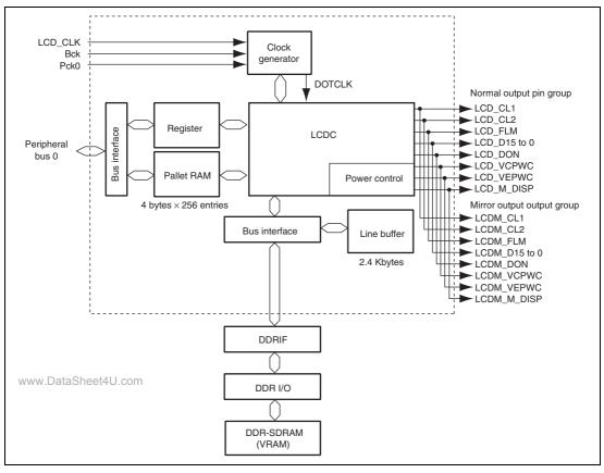
Figure 37.1 LCDC Block Diagram
