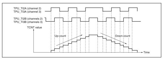
Figure 20.15 Example of Phase Counting Mode 1 Operation
