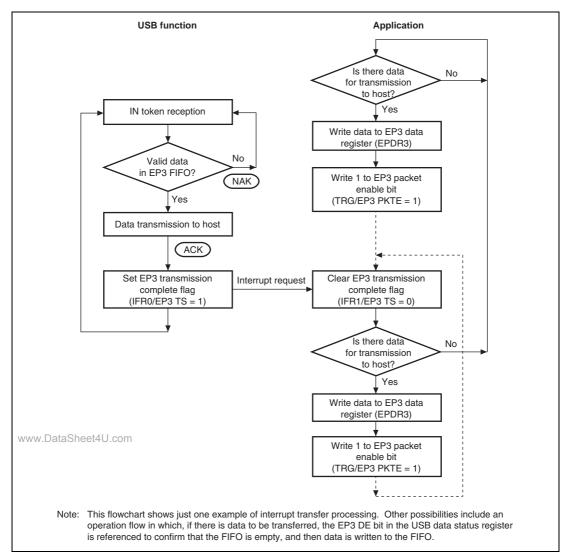
Figure 36.12 EP3 Interrupt-In Transfer Operation
