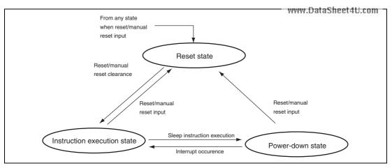
Figure 2.8 Processing State Transitions
