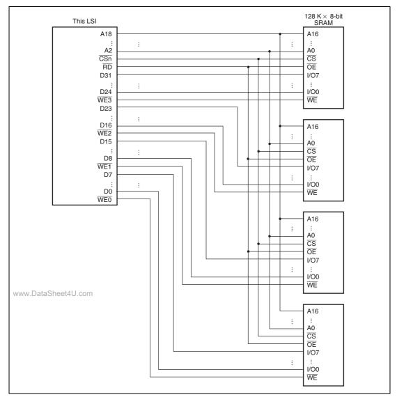
Figure 11.5 Example of 32-Bit Data-Width SRAM Connection
