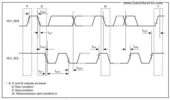
Figure 43.56 I<sup>2</sup>C Bus Interface Input/Output Timing
