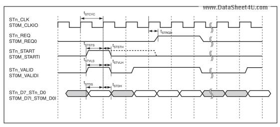
Figure 43.52 STIF Clock Valid Receive Timing
