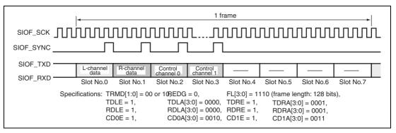
Figure 29.20 Transmit and Receive Timing (16-Bit Stereo Data)
