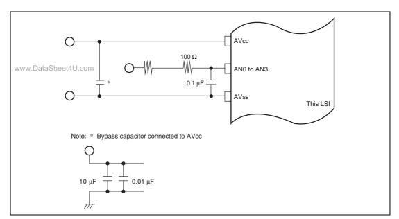
Figure 38.6 Example of Analog Input Pin Protection Circuit
