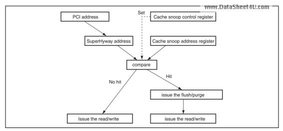
Figure 13.14 Cache Flush/Purge Execution Flow for PCI local Bus to SuperHyway Bus
