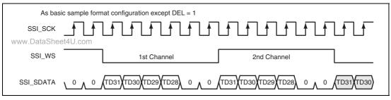
Figure 34.15 Serial Data First, Followed by Padding Bits, without Delay
