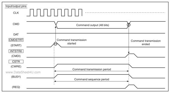
Figure 31.2 Example of Command Sequence for Commands
