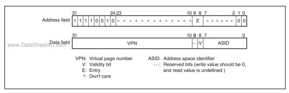
Figure 6.12 Memory-Mapped ITLB Address Array
