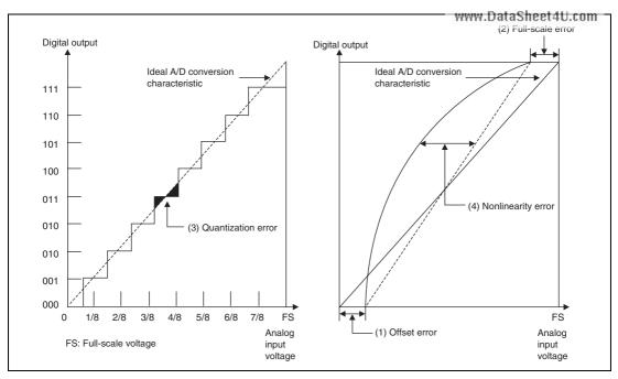
Figure 38.5 Definitions of A/D Conversion Accuracy
