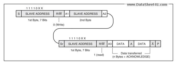
Figure 26.7 10-Bit Address Data Receive Format
