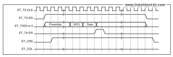
**Figure 23.19 MII Frame Transmit Timing (Transmit Error)**
