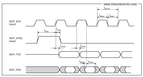
Figure 43.65 SIOF Transmission/Reception Timing (Slave Mode 1, Slave Mode 2)
