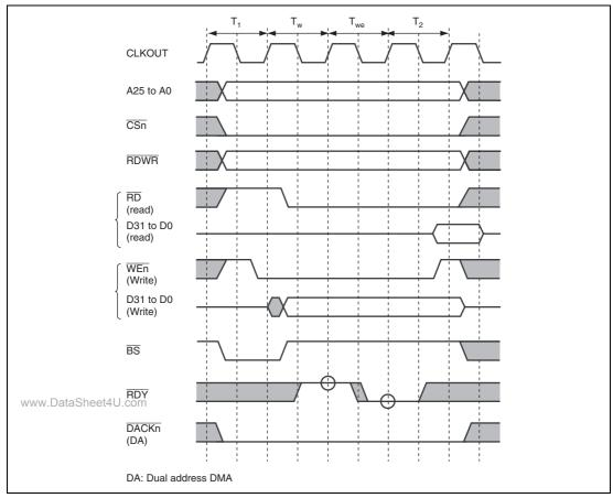
Figure 11.9 SRAM Interface Wait Cycle Timing (Wait Cycle Insertion by RDY Signal)
