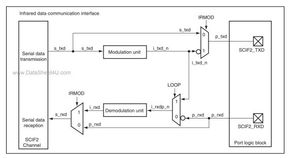
Figure 28.22 Block Diagram of Infrared Data Communication Interface
