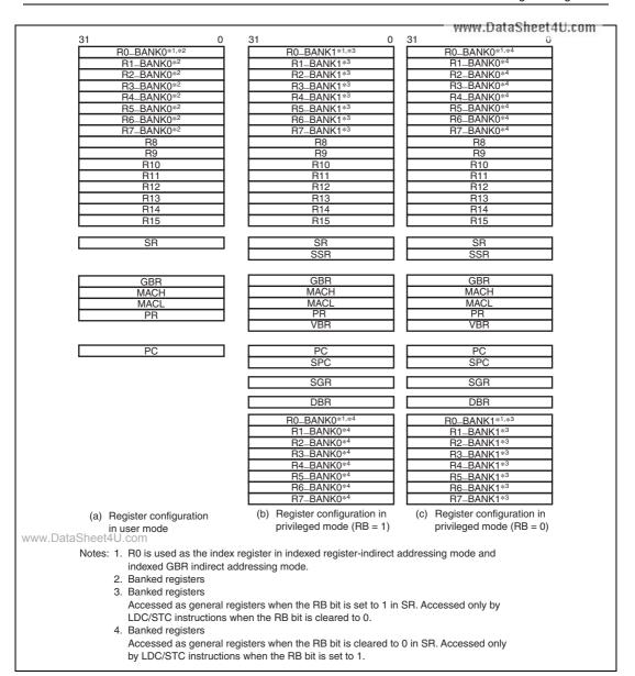
Figure 2.2 CPU Register Configuration in Each Processing Mode
