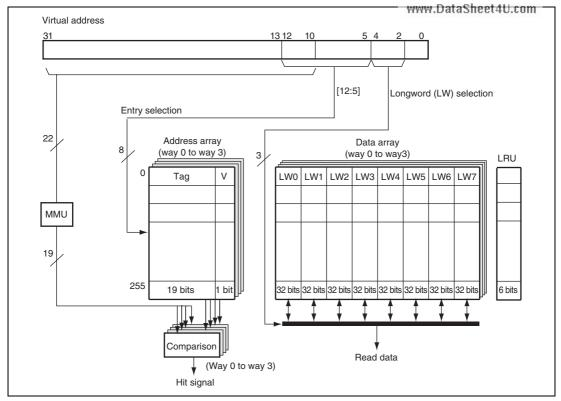
Figure 7.2 Configuration of Instruction Cache (IC)
