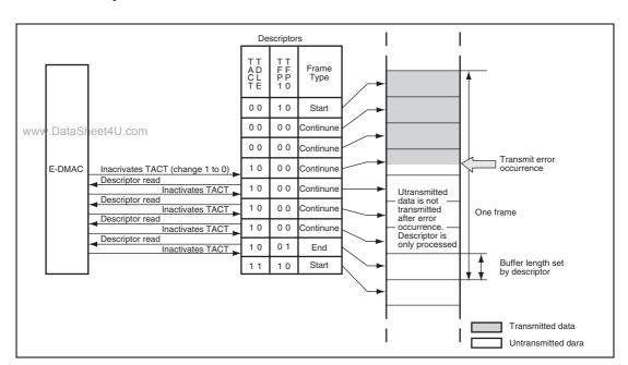
Figure 23.12 E-DMAC Operation after Transmit Error
