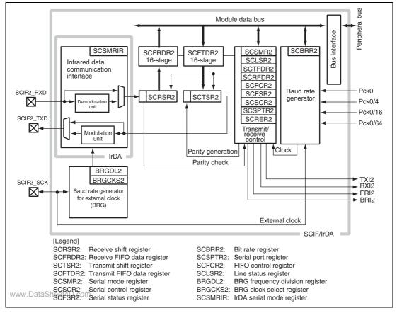
Figure 28.1 Block Diagram of SCIF/IrDA
