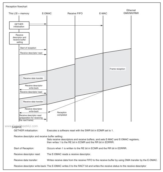
Figure 23.11 Sample Reception Flowchart (Single-Frame/Two-Descriptor)
