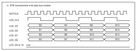
Figure 37.10 Clock and LCD Data Signal Example
