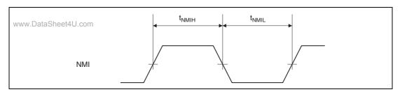
Figure 43.31 NMI Input Timing
