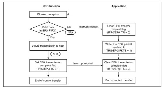
Figure 36.9 Status Stage (Control-Out) Operation
