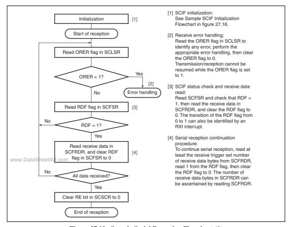
Figure 27.19 Sample Serial Reception Flowchart (1)
