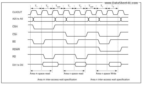
Figure 11.38 Wait Cycles between Access Cycles
