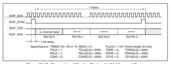
Figure 29.15 Transmit and Receive Timing (16-Bit Monaural Data)
