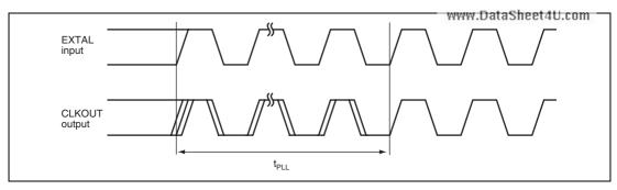
Figure 43.6 PLL Synchronization Settling Time
