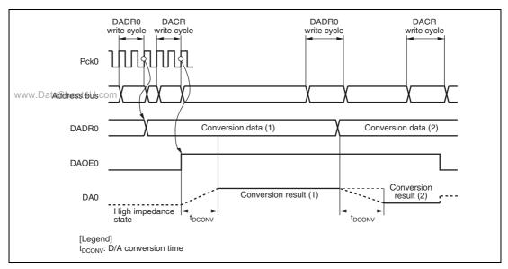
Figure 39.2 D/A Converter Operation Example
