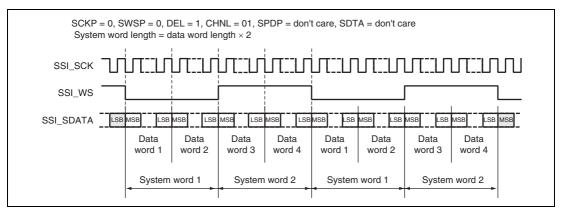
Figure 34.6 Multichannel Format (2 Channels, No Padding)
