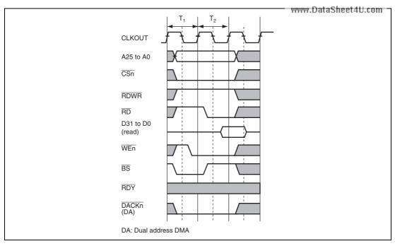
Figure 11.35 Byte-Control SRAM Basic Read Cycle (No Wait)
