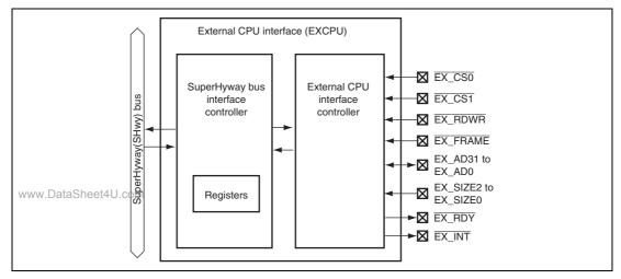
Figure 15.1 EXCPU Block Diagram
