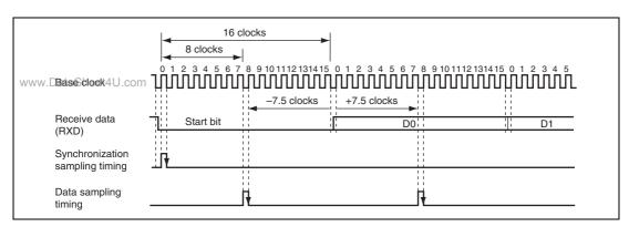
Figure 28.20 Receive Data Sampling Timing in Asynchronous Mode
