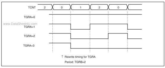
Figure 20.13 Examples of PWM Mode Operation (2)
