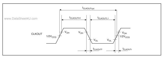
Figure 43.3 CLKOUT Clock Output Timing (1)
