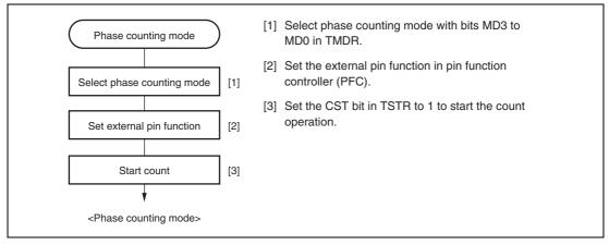
Figure 20.14 Example of Phase Counting Mode Setting Procedure
