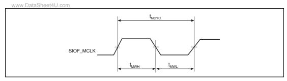
Figure 43.60 SIOF\_MCLK Input Timing
