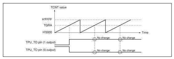
Figure 20.6 Example of 0 Output/1 Output Operation
