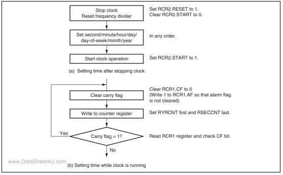
Figure 22.2 Examples of Time Setting Procedures
