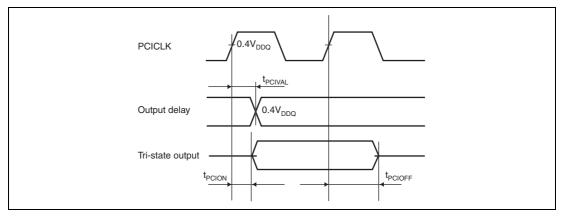
Figure 46.35 Output Signal Timing
