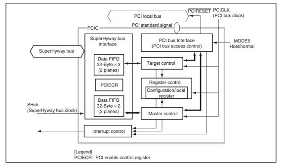
Figure 13.1 PCIC Block Diagram
