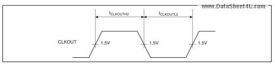
Figure 43.4 CLKOUT Clock Output Timing (2)
