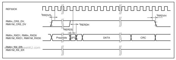
Figure 43.50 RMII Receive Timing (normal operation)
