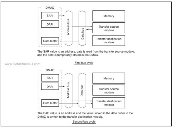
Figure 14.4 Data Flow of Dual Address Mode
