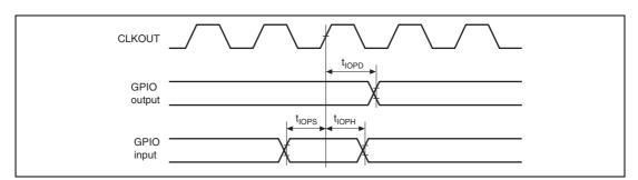
Figure 43.80 GPIO Timing
