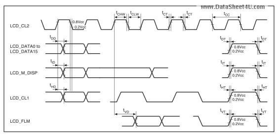
Figure 43.79 LCDC Module Signal Timing
