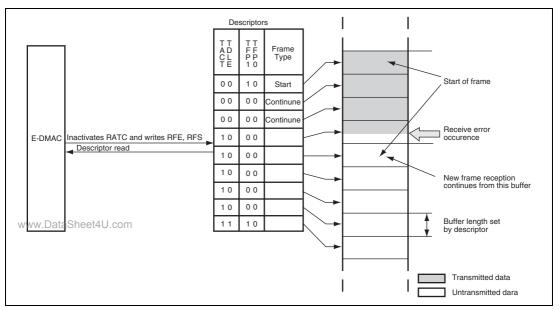
Figure 23.13 E-DMAC Operation after Receive Error
