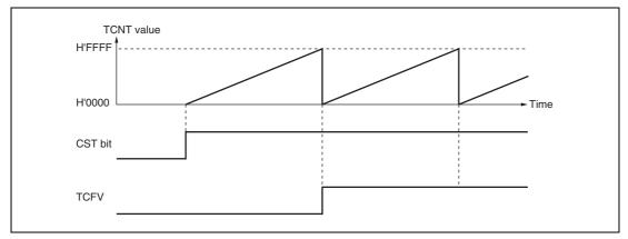
Figure 20.3 Free-Running Counter Operation
