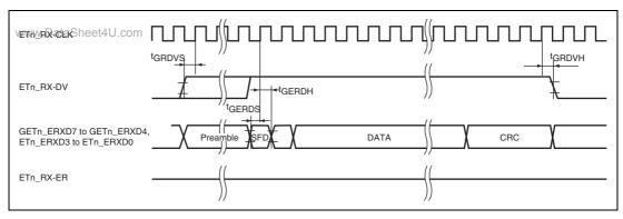
Figure 43.46 GMII Receive Timing (normal operation)
