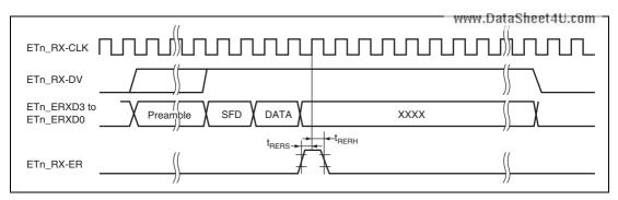
Figure 43.43 MII Receive Timing (When an Error is Detected)
