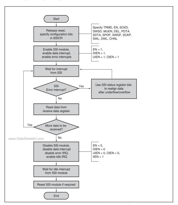
Figure 34.22 Reception using Interrupt Data Flow Control
