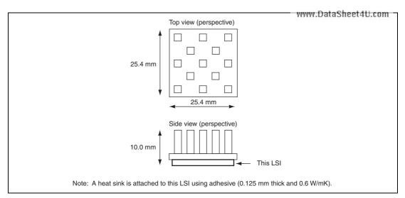
Figure J.2 Heat Sink Model
