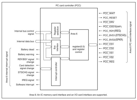
Figure 32.1 PC Card Controller Block Diagram
