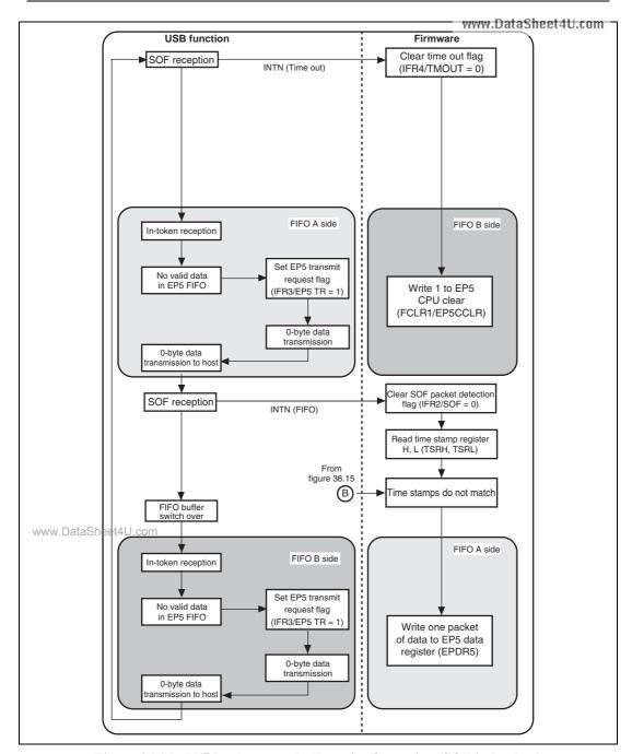
Figure 36.16 EP5 Isochronous-In Transfer Operation (SOF in Broken)
