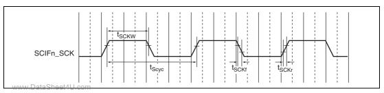
Figure 43.58 SCIFn\_SCK Input Clock Timing
