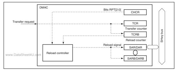
Figure 14.12 Reload Mode Transfer
