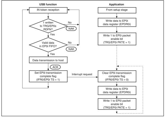
Figure 36.6 Data Stage (Control-In) Operation
