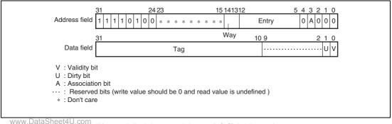
Figure 7.7 Memory-Mapped OC Address Array
