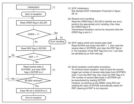
Figure 28.16 Sample Serial Reception Flowchart (1)
