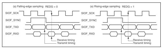
Figure 29.4 SIOF Transmit/Receive Timing
