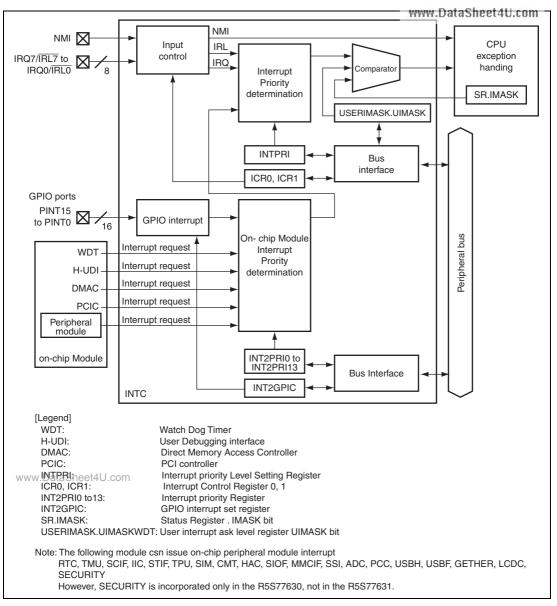
Figure 9.1 Block Diagram of INTC
