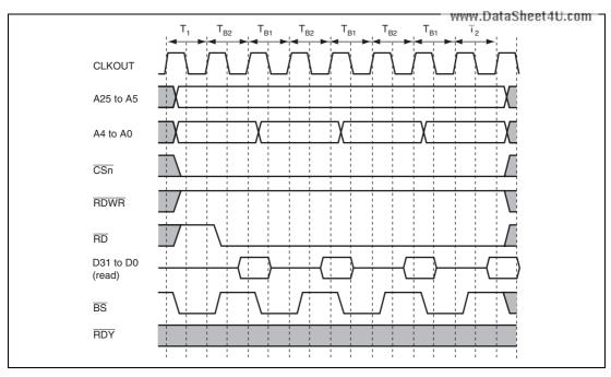
Figure 11.11 Burst ROM Basic Access Timing
