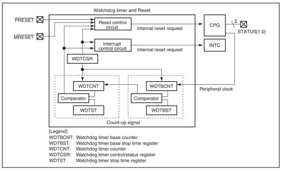
Figure 17.1 System Block Diagram
