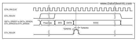
Figure 43.47 GMII Receive Timing (When an Error is Detected)
