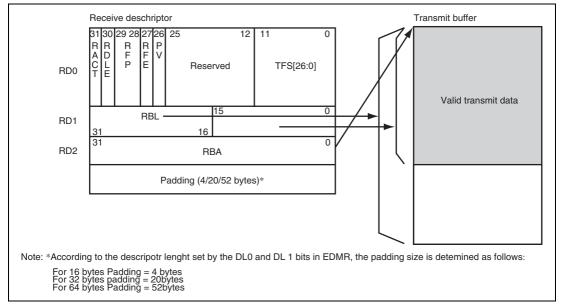
Figure 23.4 Relationship between Receive Descriptor and Receive Buffer
