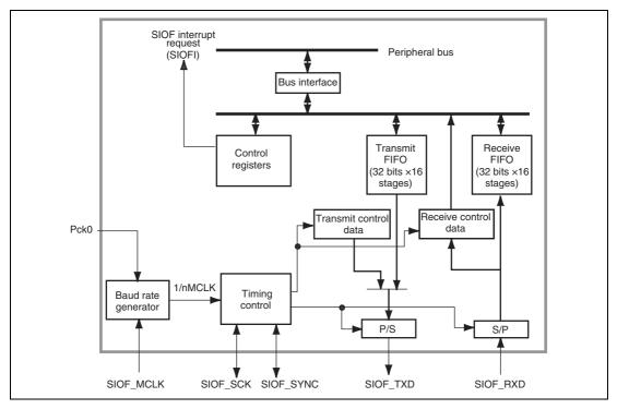
Figure 29.1 Block Diagram of SIOF
