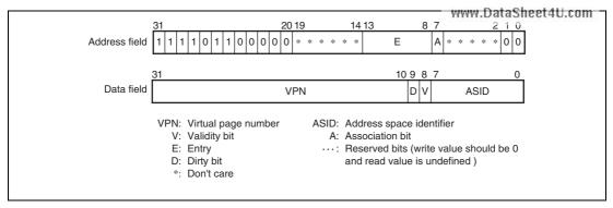
Figure 6.14 Memory-Mapped UTLB Address Array
