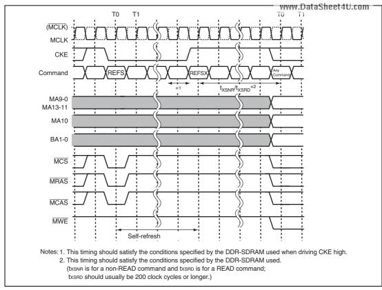
Figure 12.14 Basic DDRIF Timing (Self-Refresh Entry from IDLE (REFS)/Self-Refresh Exit (REFSX) to Any Command Input)
