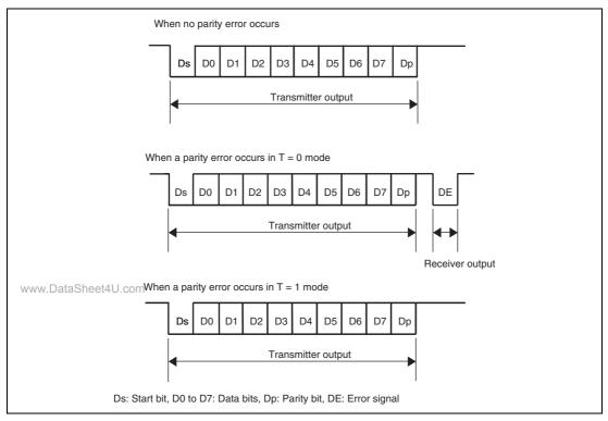
Figure 30.2 Data Format Used by Smart Card Interface
