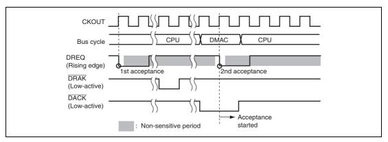
Figure 14.13 Example of DREQ Input Detection in Cycle Steal Mode Edge Detection
