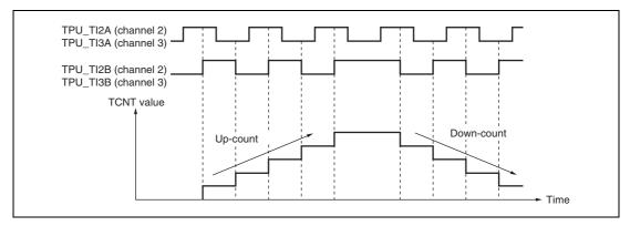
Figure 20.18 Example of Phase Counting Mode 4 Operation
