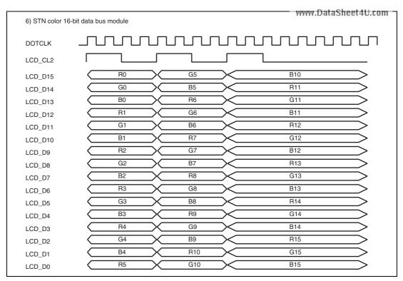
Figure 37.15 Clock and LCD Data Signal Example (STN Color 16-Bit Data Bus Module)
