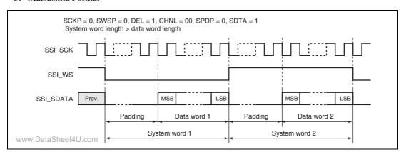
Figure 34.5 Matsushita Format (with Padding Bits First, Followed by Serial Data)
