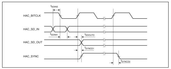
Figure 43.72 HAC Interface Module Signal Timing
