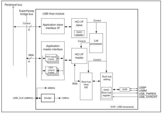
Figure 35.1 Block Diagram of USBH
