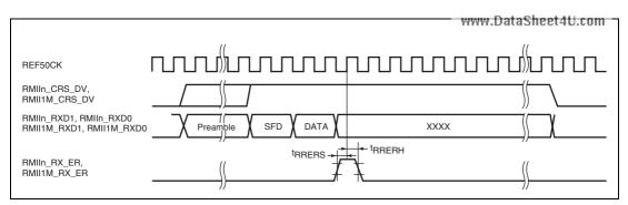
Figure 43.51 RMII Receive Timing (When an Error is Detected)
