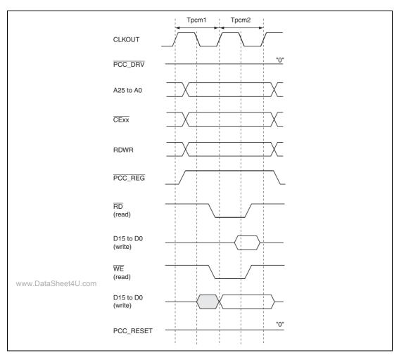
Figure 32.5 PCMCIA Memory Card Interface Basic Timing
