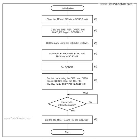
Figure 30.4 Example of Initialization Flow
