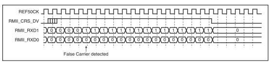
Figure 23.30 RMII Fame Receive Timing (100-Mbps Reception with Illegal Carrier Detected)
