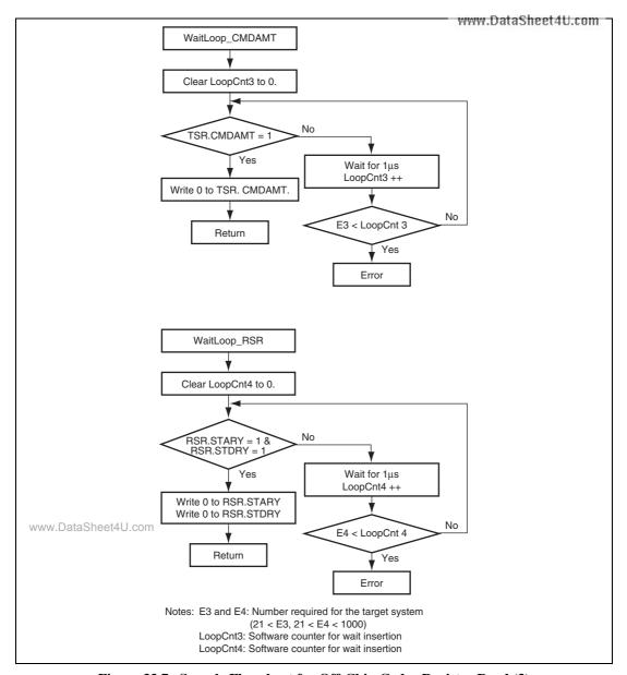
Figure 33.7 Sample Flowchart for Off-Chip Codec Register Read (3)
