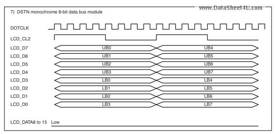
Figure 37.16 Clock and LCD Data Signal Example (DSTN Monochrome 8-Bit Data Bus Module)
