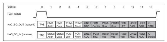
Figure 33.2 AC97 Frame Slot Structure
