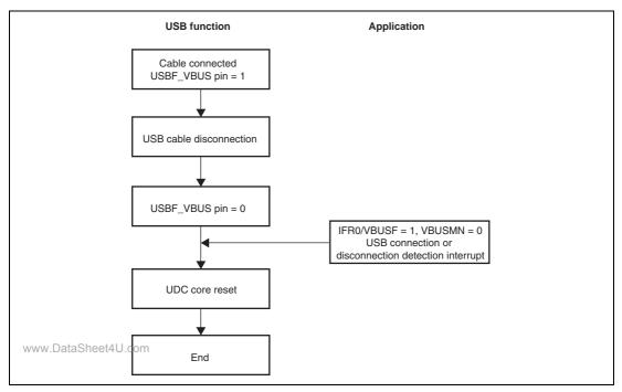
Figure 36.4 Cable Disconnection Operation
