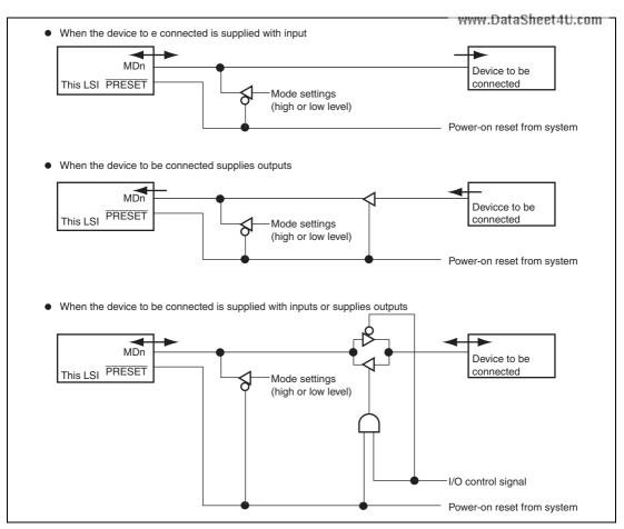
www.DataSheet4U.conFigure D.1 Schematic Diagram of External Circuits
