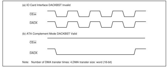
Figure 11.14 CExx and DACK Output of ATA Complete Mode in DMA Transfer
