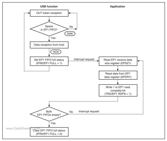
Figure 36.10 EP1 Bulk-Out Transfer Operation
