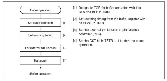
Figure 20.9 Example of Buffer Operation Setting Procedure
