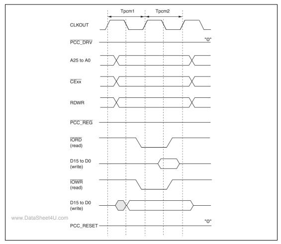
Figure 32.7 PCMCIA I/O Card Interface Basic Timing
