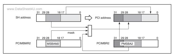
Figure 13.5 SuperHyway Bus to PCI Local Bus Address Translation (PCI Memory Space 2)
