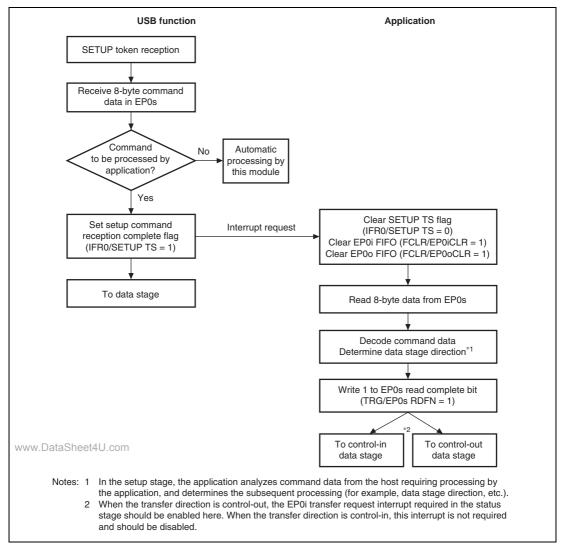
Figure 36.5 Setup Stage Operation
