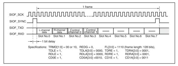
Figure 29.18 Transmit and Receive Timing (16-Bit Stereo Data (3))
