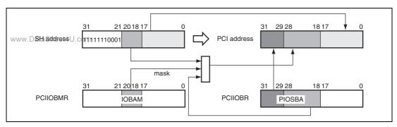
Figure 13.6 SuperHyway Bus to PCI Local Bus Address Translation (PCI I/O)
