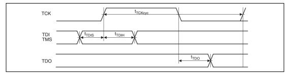
Figure 43.83 H-UDI Data Transfer Timing
