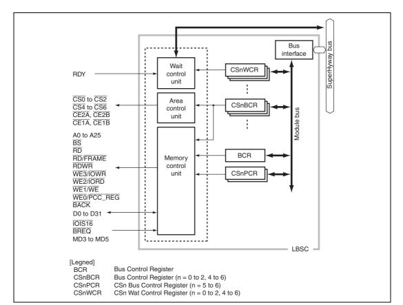
Figure 11.1 LBSC Block Diagram
