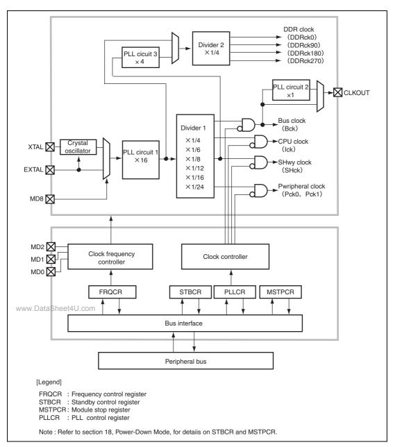
Figure 16.1 Block Diagram of CPG
