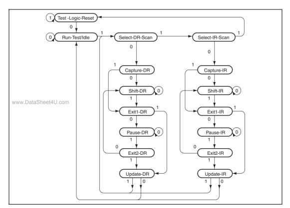
Figure 42.3 TAP Controller State Transitions
