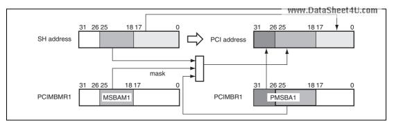
Figure 13.4 SuperHyway Bus to PCI Local Bus Address Translation (PCI Memory Space 1)
