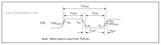
Figure 43.81 TCK Input Timing
