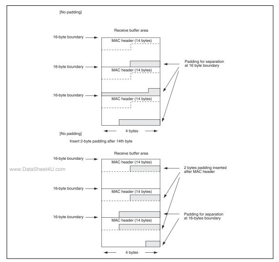
Figure 23.14 Padding Insertion in Receive Data
