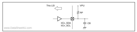
Figure 43.57 AC Characteristic Load Condition
