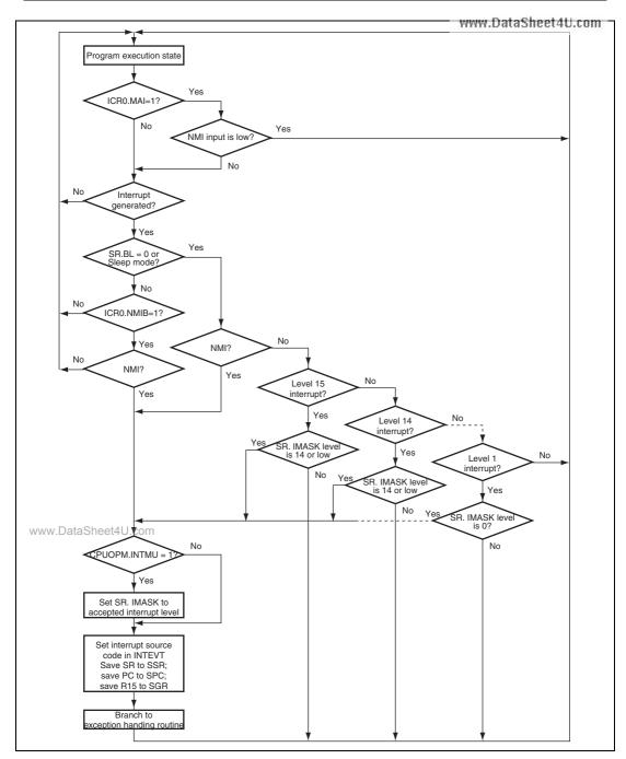
Figure 9.4 Interrupt Operation Flowchart
