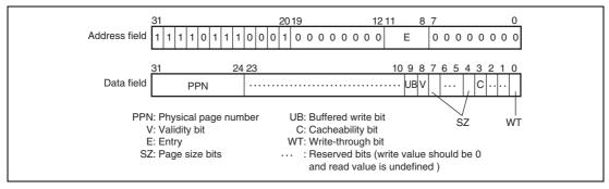
Figure 6.19 Memory-Mapped PMB Data Array
