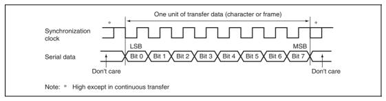
Figure 27.15 Data Format in Clocked Synchronous Communication
