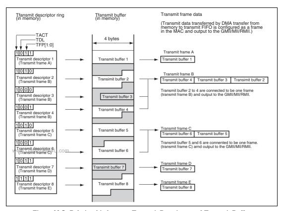
Figure 23.5 Relationship between Transmit Descriptor and Transmit Buffer
