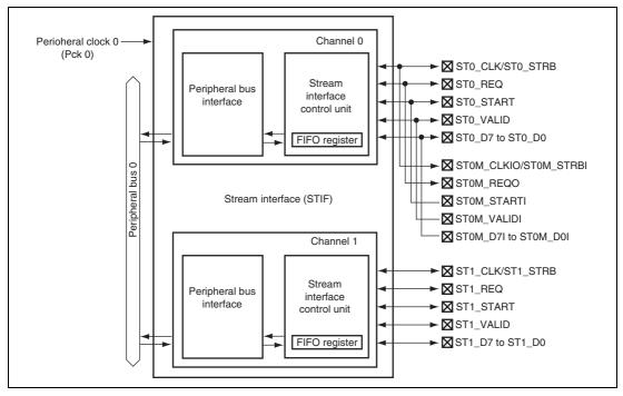
Figure 25.1 Block Diagram of STIF
