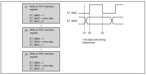
Figure 23.33 1-Bit Data Write Flowchart
