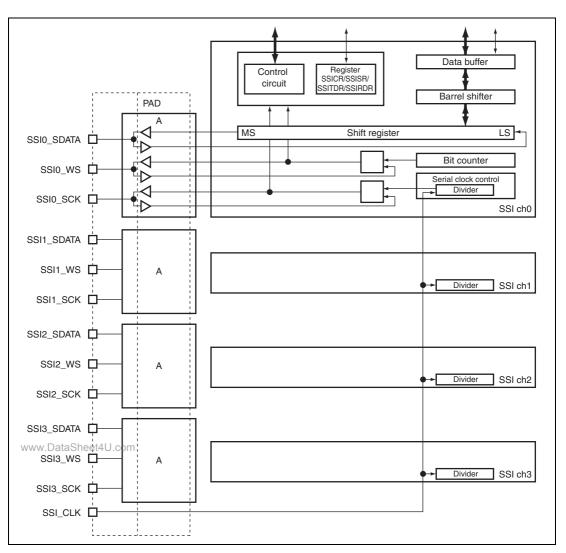
Figure 34.1 Block Diagram of SSI Module
