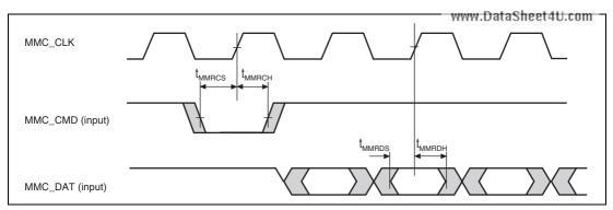
Figure 43.68 MMCIF Receive Timing (Sampling at the Rising Edge)
