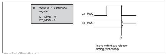
Figure 23.36 Independent Bus Release Flowchart (IDLE in Write in Figure 23.33)
