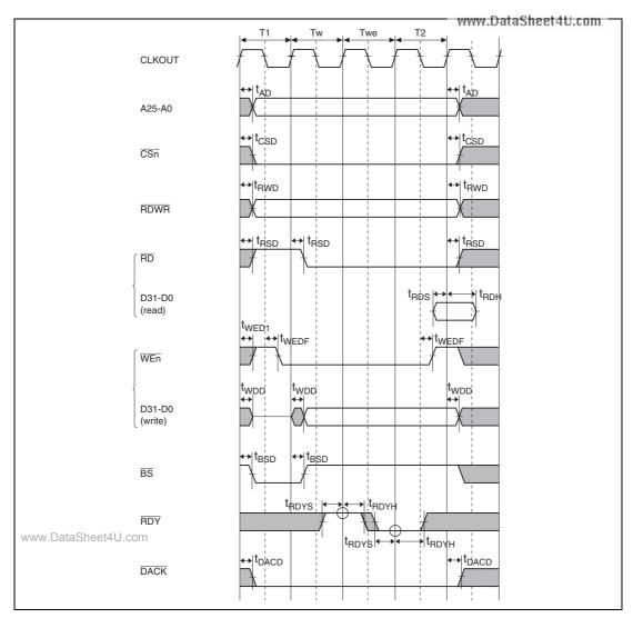
Figure 43.13 SRAM Bus Cycle: Basic Bus Cycle (One Wait by Software + One Wait by RDY, RDY Signal is Synchronous Input)
