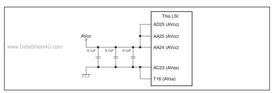
Figure E.1 Connection Example of Bypass Capacitors for Analog Power Supply
