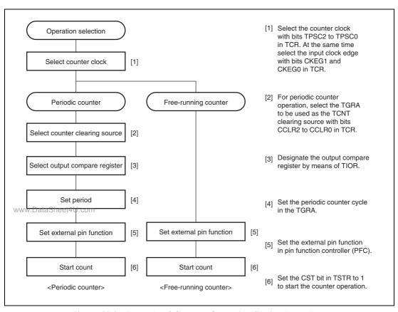
Figure 20.2 Example of Counter Operation Setting Procedure
