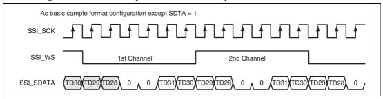
Figure 34.13 Padding Bits First, Followed by Serial Data, with Delay
