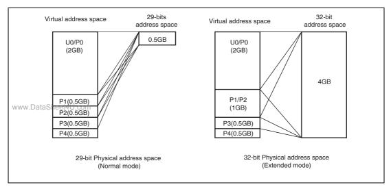
Figure 6.16 Physical Address Space (32-Bit Address Extended Mode)
