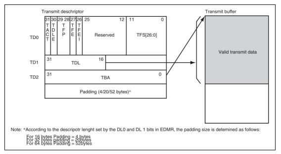
Figure 23.3 Relationship between Transmit Descriptor and Transmit Buffer
