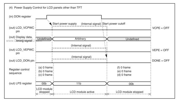
Figure 37.7 Power-Supply Control Sequence and States of the LCD Module
