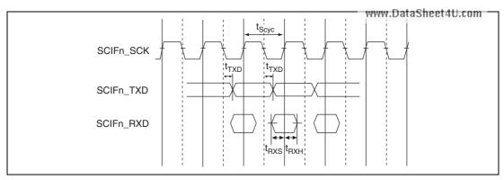
Figure 43.59 SCIFn I/O Synchronous Mode Clock Timing
