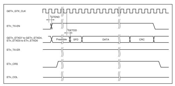
Figure 43.45 GMII Transmit Timing (normal operation)
