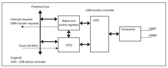
Figure 36.1 Block Diagram of USBF
