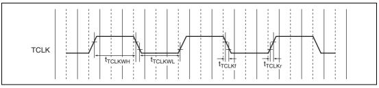
Figure 43.38 TCLK Input Timing
