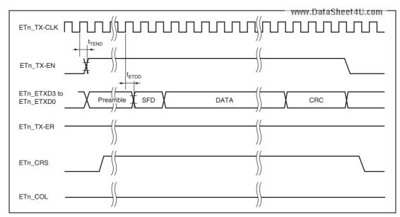
Figure 43.41 MII Transmit Timing (normal operation)
