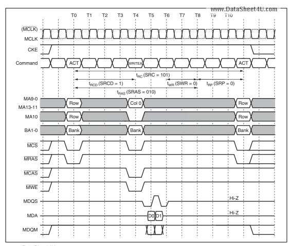
Figure 12.8 Basic DDRIF Timing (1 Burst Write: 1, 2, 4, or 8 Bytes; With Auto-Precharge)
