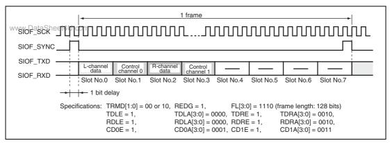
Figure 29.19 Transmit and Receive Timing (16-Bit Stereo Data (4))
