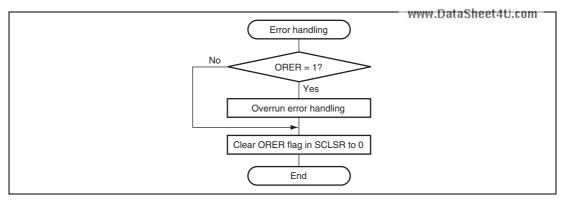
Figure 28.17 Sample Serial Reception Flowchart (2)
