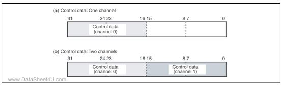
Figure 29.6 Control Data Bit Alignment
