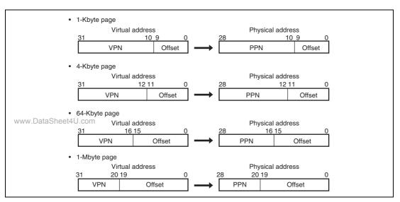
Figure 6.7 Relationship between Page Size and Address Format
