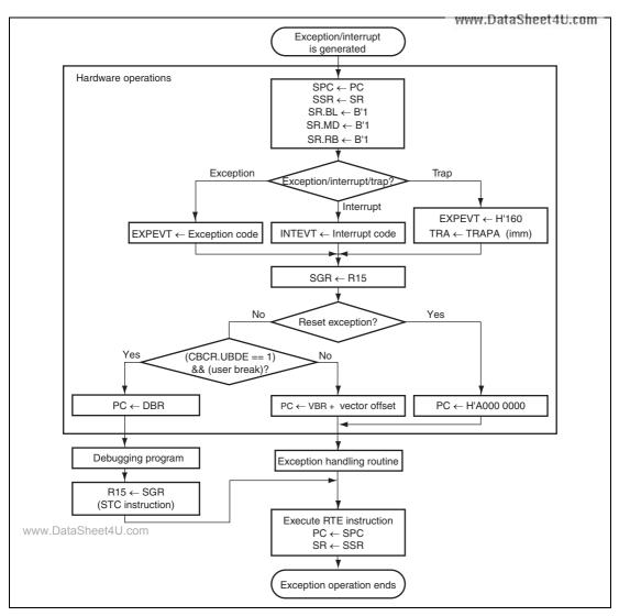
Figure 41.2 Flowchart of User Break Debugging Support Function
