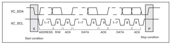
Figure 26.2 I<sup>2</sup>C Bus Timing
