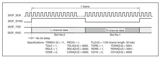
Figure 29.16 Transmit and Receive Timing (16-Bit Stereo Data (1))
