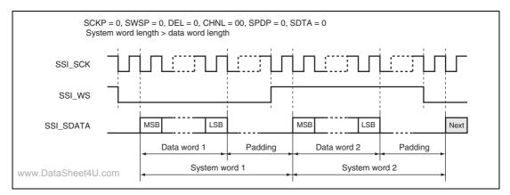
Figure 34.3 Philips Format (with Padding)
