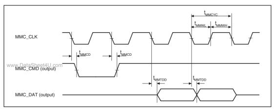
Figure 43.67 MMCIF Transmit Timing
