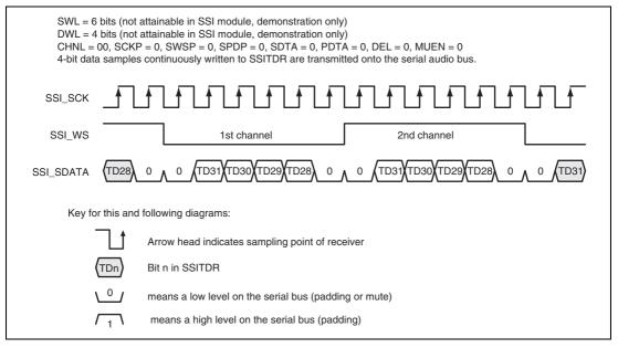
Figure 34.9 Basic Sample Format www.DataSheet4U.(Fransmit Mode with Example System/Data Word Length)
