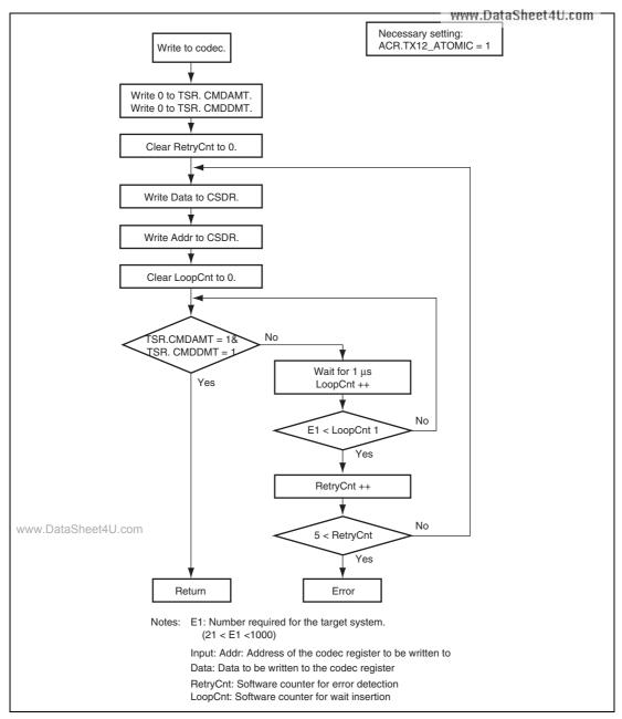
Figure 33.4 Sample Flowchart for Off-Chip Codec Register Write
