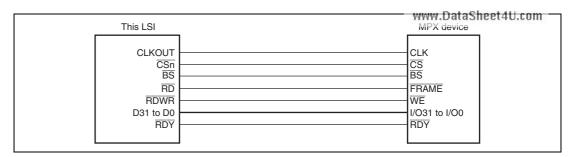
Figure 11.21 Example of 32-Bit Data Width MPX Connection
