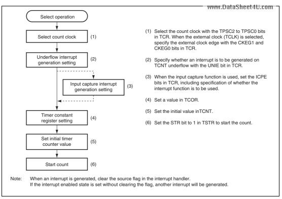
Figure 19.2 Example of Count Operation Setting Procedure
