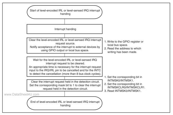
Figure 9.5 Example of Interrupt Handling Routine
