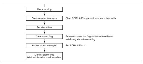
Figure 22.4 Example of Use of Alarm Function
