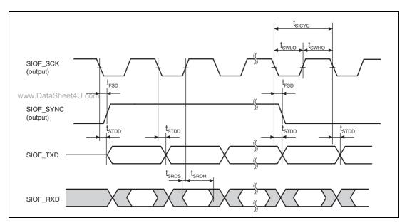
Figure 43.64 SIOF Transmission/Reception Timing (Master Mode 2, Sampling at the Rising Edge)
