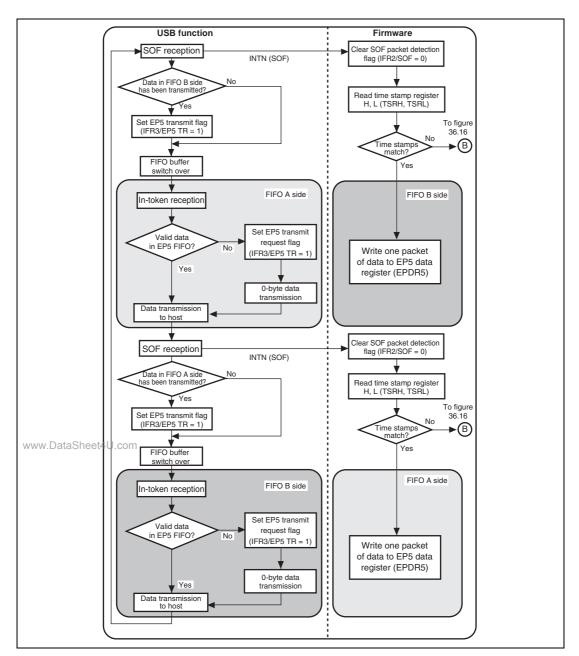
Figure 36.15 EP5 Isochronous-In Transfer Operation (SOF is Normal)
