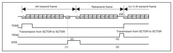
Figure 30.9 Retransmit Standby Mode (Clock Stopped) when Smart Card Interface is in Transmit Mode
