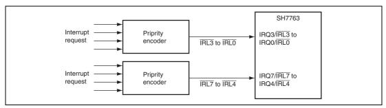
Figure 9.2 Example of IRL Interrupt Connection
