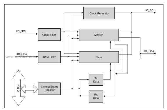
Figure 26.1 Block Diagram for I<sup>2</sup>C Bus Interface
