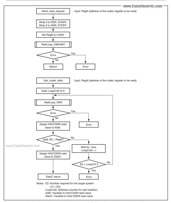
Figure 33.6 Sample Flowchart for Off-Chip Codec Register Read (2)
