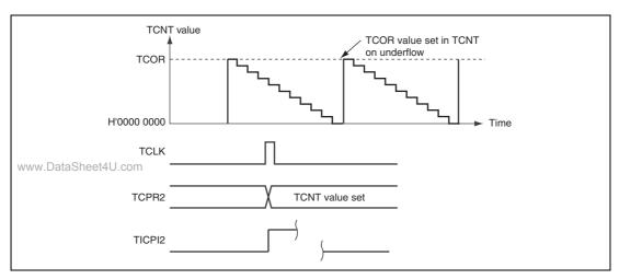
Figure 19.7 Operation Timing when Using Input Capture Function
