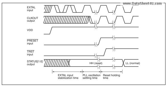
Figure 17.3 STATUS Output during Power-on
