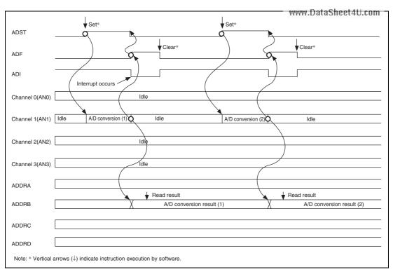
Figure 38.2 Example of A/D Converter Operation (Single Mode, Channel 1 Selected)
