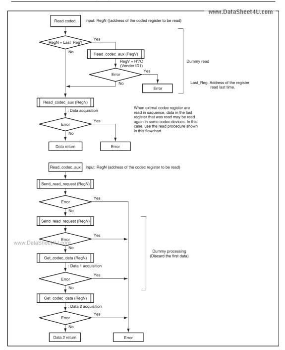
Figure 33.5 Sample Flowchart for Off-Chip Codec Register Read (1)
