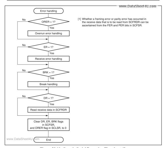
Figure 28.10 Sample Serial Reception Flowchart (2)
