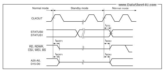
Figure 43.10 Pin Drive Timing in Standby Mode
