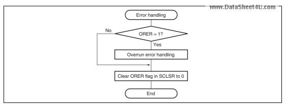
Figure 27.19 Sample Serial Reception Flowchart (2)
