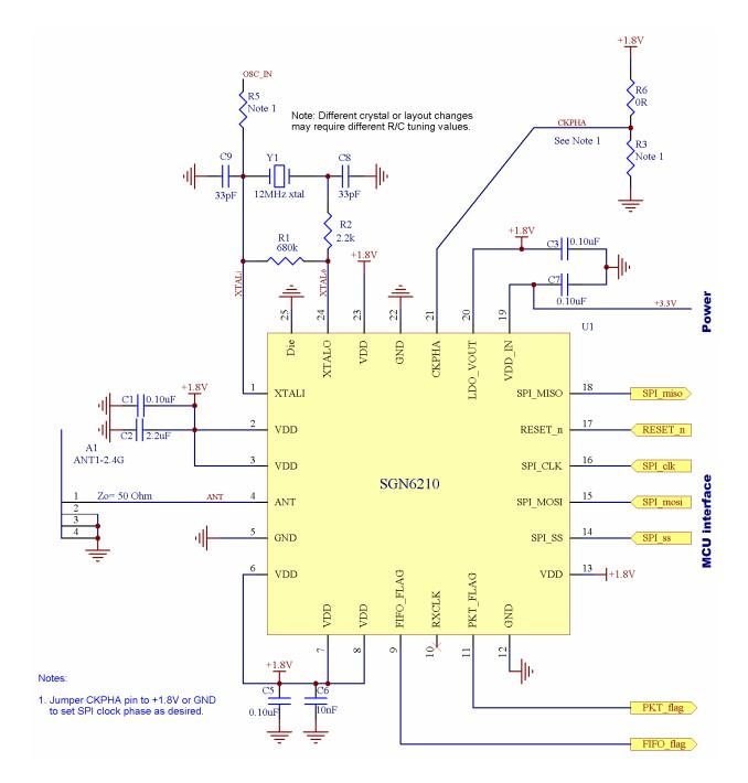
Simple, low-power (0 dBm) 2.4 GHz RF Transceiver with Framing and data buffers
