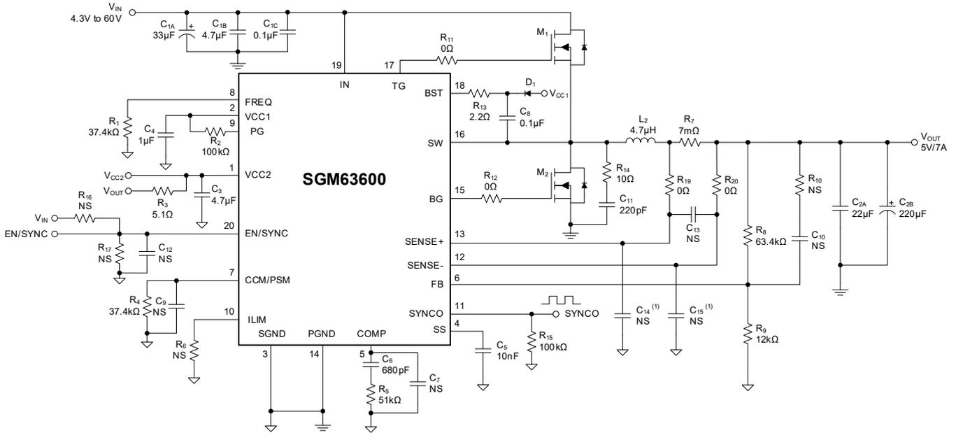
NOTE: 1. The recommended values for C14 and C15 are 10nF in TSSOP package.
