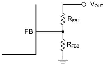
Figure 5. Output Voltage (V<sub>OUT</sub>) Setting
