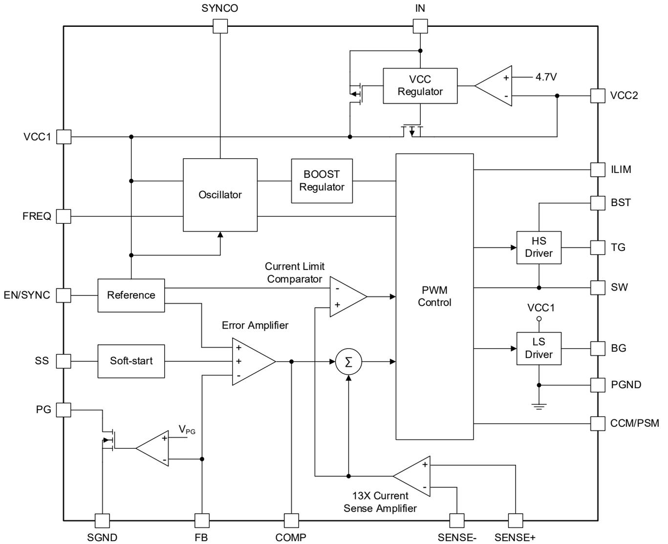
Figure 2. Block Diagram
