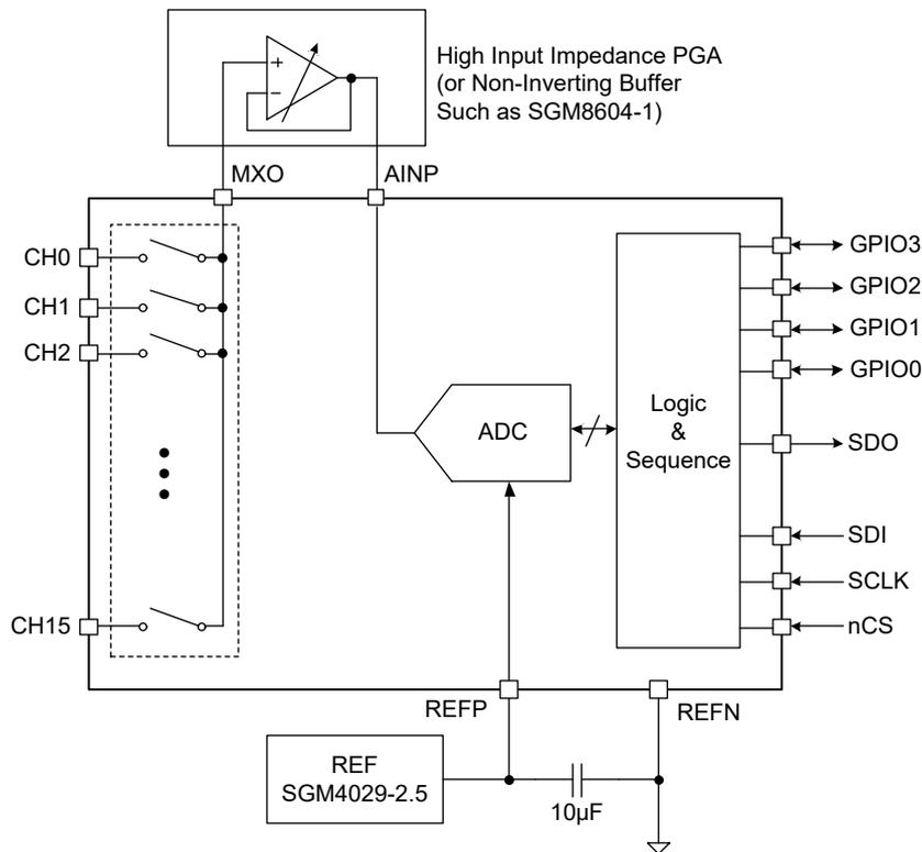
Figure 4. Typical Application Circuit
