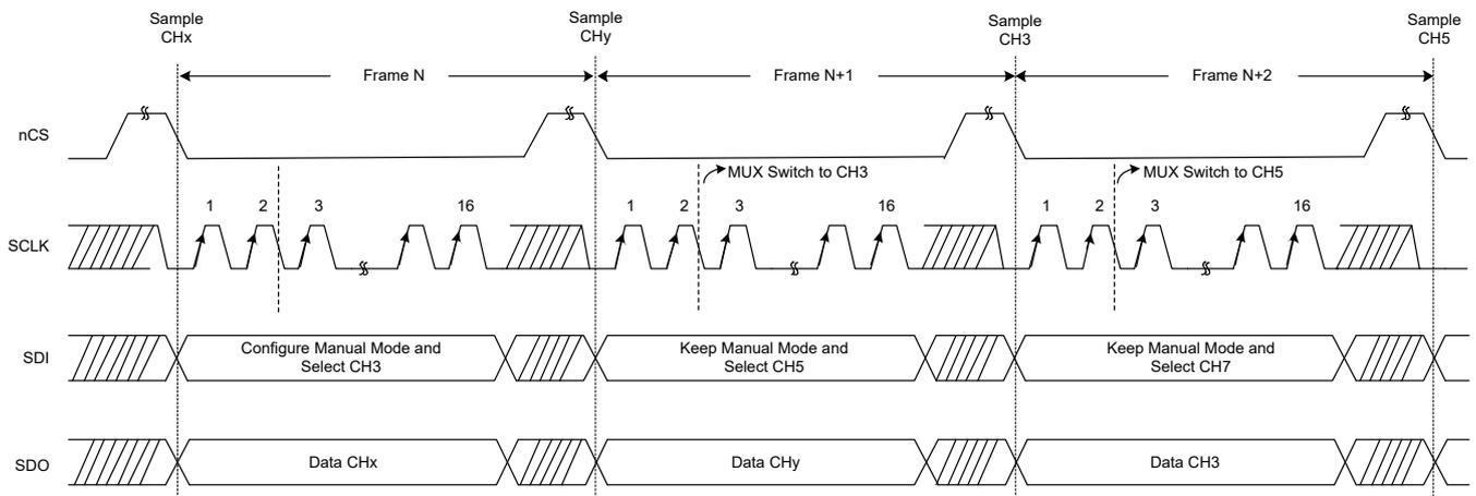
Figure 5. Example for Manual Mode Timing Diagram
