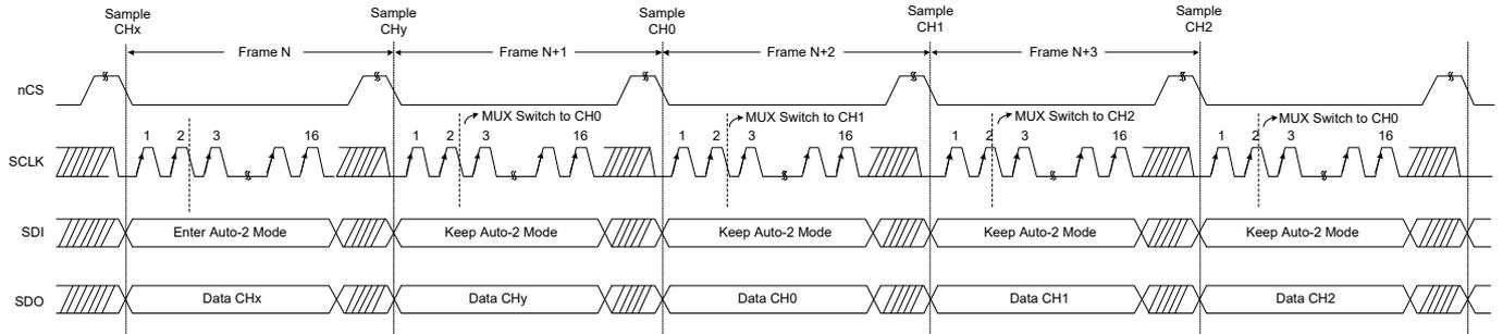
Figure 8. Example for Auto-2 Mode Timing Diagram
