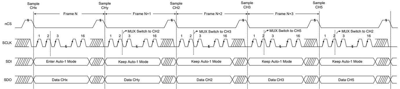
Figure 6. Example for Auto-1 Mode Timing Diagram
