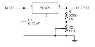
FIGURE 2 - ADJUSTABLE OUTPUT REGULATOR
