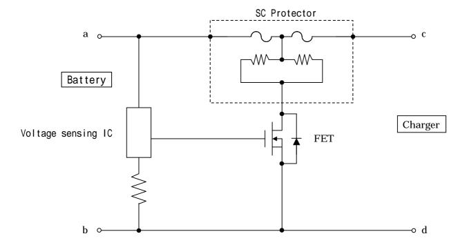
When the voltage between a and b exceeds the pre-set limit value, the output of the voltage detector IC becomes high and the FET is switched on. As a result, current flow through the heater of the protector, the fuses melt, and the battery stops to be charged any longer.
