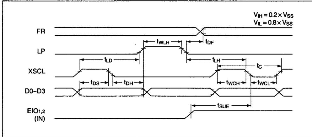
$V_{SS} = -5.0V \pm 0.5V$ ,  $T_a = -40$  to  $85^\circ C$
