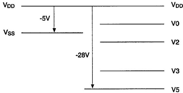
Note 4. When logic power becomes floating state or if V<sub>SS</sub> = -2.6 or beyond while the LCD driver power source is being applied, the LSI may be permanently damaged and avoid such circumstances.
