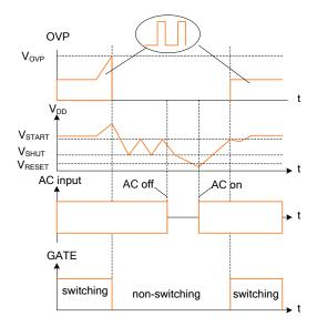
The output over-voltage protection waveform (Auto-restart) of SD4872R is shown below.
