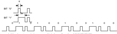
One word of the above transmission command is in the configuration of (010100100100).
