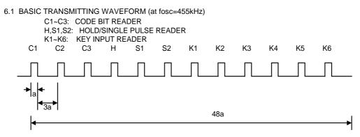
Basic transmitting waveform is 12-bits serial data in configuration as shown above.
