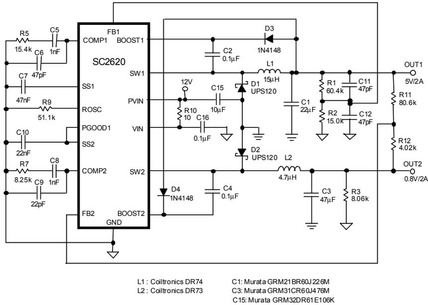
Figure 17(a). 500kHz 12V to 5V and 0.8V step-down converter. Notice that  $V_{OUT2}$  is lower than the nominal FB voltage.  $R_{11}$  and  $R_{12}$  constitute the feedback voltage divider for Channel 2.
