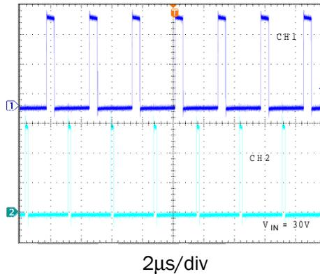
Figure 18(b). Switching Waveforms.  $I_{OUT1} = I_{OUT2} = 1A$ .
