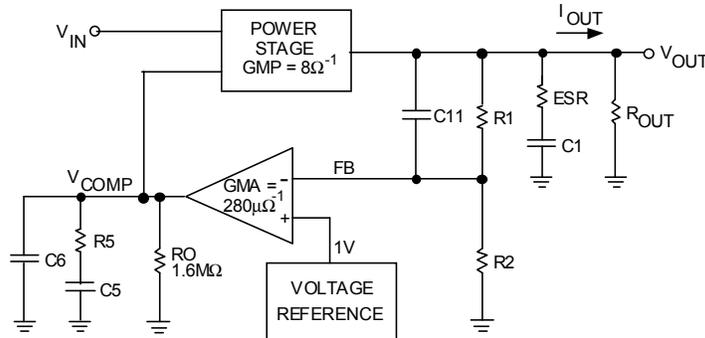
Figure 11. Simplified Control Loop Equivalent Circuit
