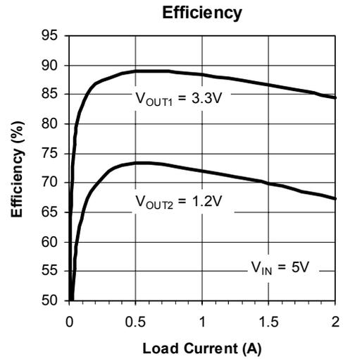
Figure 16(a). 1.2MHz 5V to 3.3V and 1.2V xDSL Power Supply. Channel 2 does not start until Channel 1 output voltage becomes regulated.
