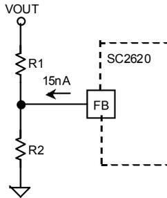
Figure 4.  $V_{OUT}$  is set with a Resistive Divider
