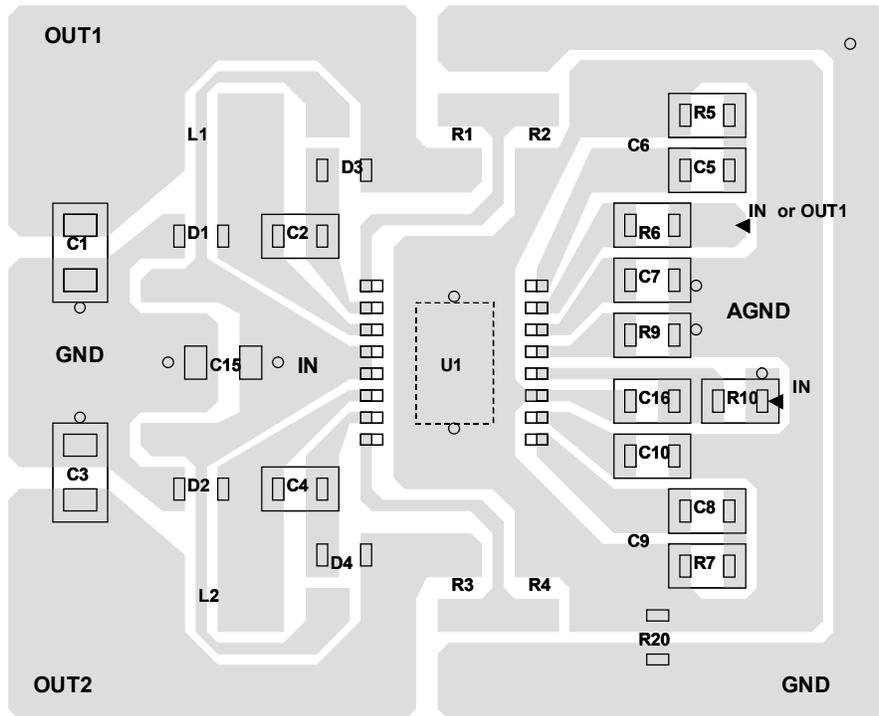
Figure 15. Suggested PCB Layout for the SC2620.
