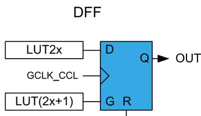
When the even LUT is disabled (LUTCTRL2x.ENABLE=0), the flip-flop is asynchronously cleared. The reset command (R) is kept enabled for one APB clock cycle. In all other cases, the flip-flop output (OUT) is refreshed on rising edge of the GCLK\_CCL, as shown in [Table 40-2](#).
