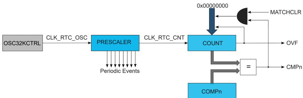
Figure 25-2. RTC Block Diagram (Mode 1 — 16-Bit Counter)
