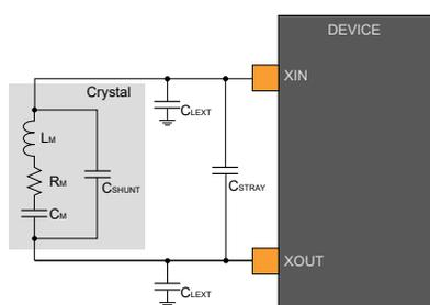
The user must choose a crystal oscillator where the crystal load capacitance  $C_L$  is within the range given in the table. The exact value of  $C_L$  can be found in the crystal data sheet. The capacitance of the external capacitors ( $C_{LEXT}$ ) can then be computed as follows:
