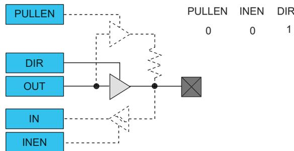
**Figure 29-7.** I/O Configuration - Totem-Pole Output with Enabled Input
