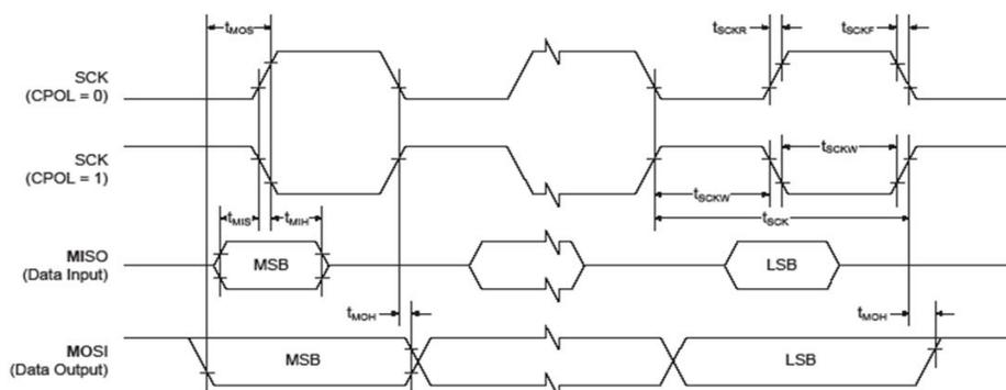
Figure 46-8. SPI Timing Requirements in Client Mode
