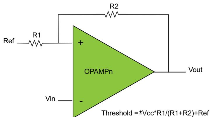
To configure an OPAMP as a non-inverting comparator with programmable hysteresis, the OPAMPCTRLx register can be configured as follows:
