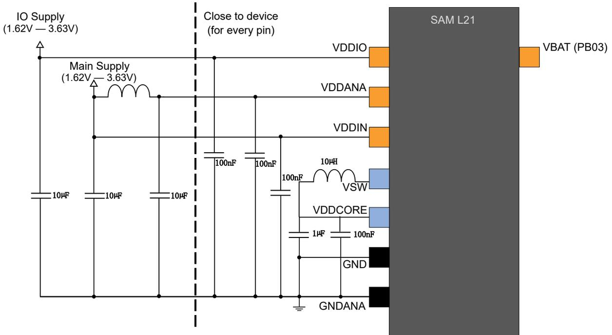
Figure 51-2. Power Supply Connection for Linear Mode Only
