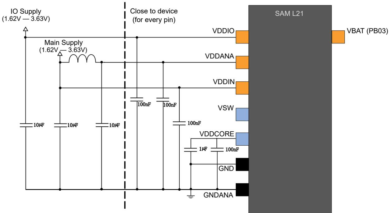
**Figure 51-3.** Power Supply Connection for Battery Backup
