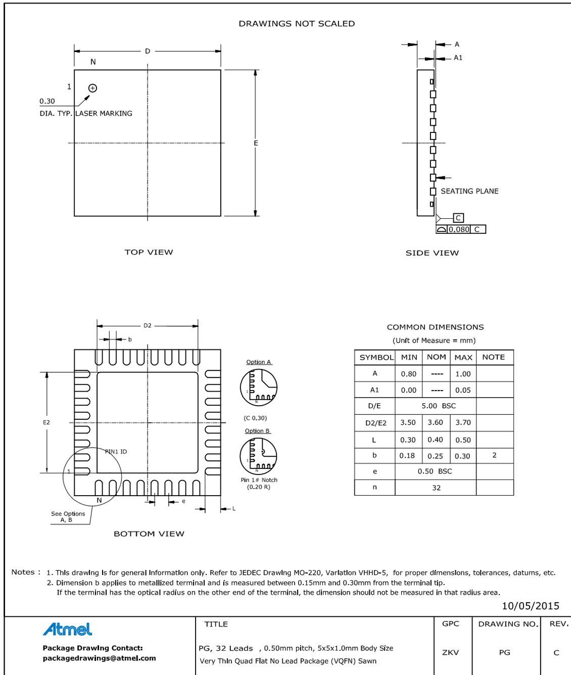
**Note:** The exposed die attach pad is connected inside the device to GND and GNDANA.
