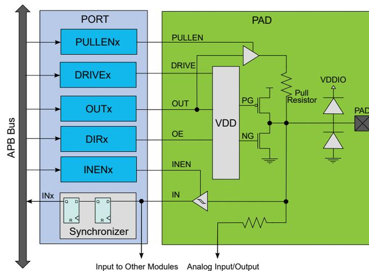
**Note:** The ESD diode connected to VDDIO is not plugged for the Back-up I/Os. For these specific pins, only the ESD diode connected to ground is implemented.
