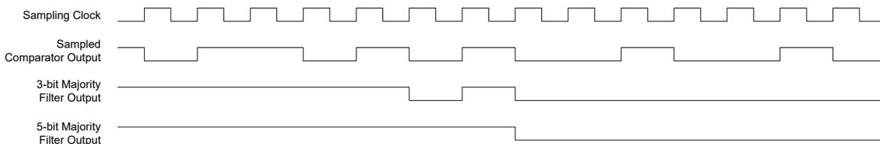
**Figure 43-7. Single-Shot Filtering**
