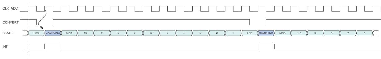
**Figure 42-7.** ADC Timing for Free Running in 8-bit Resolution
