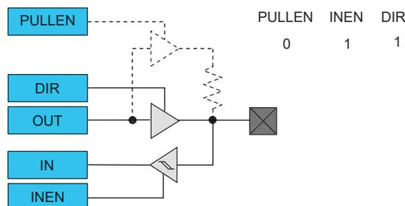
**Figure 29-8.** I/O Configuration - Output with Pull
