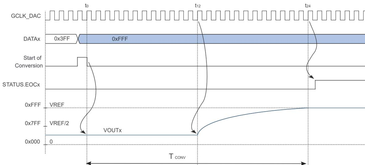
Since the DAC conversion is implemented as pipelined procedure, a new conversion can be started after only 12 GCLK\_DAC periods. Therefore if DATAx is written while a conversion is ongoing, start of conversion is postponed until DACx is ready to start next conversion.
