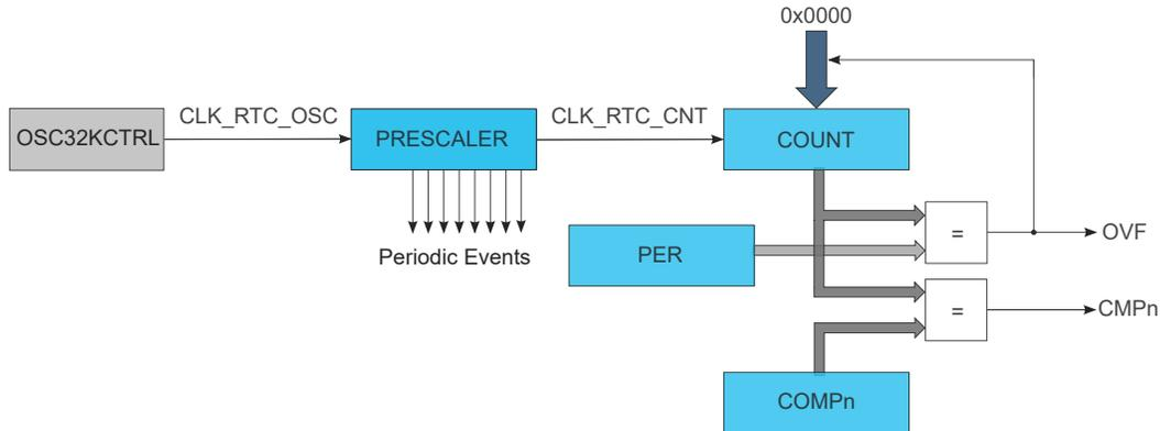
Figure 25-3. RTC Block Diagram (Mode 2 — Clock/Calendar)
