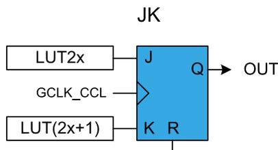
When the even LUT is disabled ( $LUTCTRL2x.ENABLE=0$ ), the flip-flop is asynchronously cleared. The reset command (R) is kept enabled for one APB clock cycle. In all other cases, the flip-flop output (OUT) is refreshed on rising edge of the GCLK\_CCL, as shown in [Table 40-3](#).
