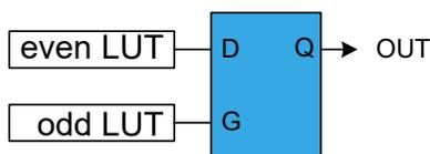
When the even LUT is disabled ( $LUTCTRL2x.ENABLE=0$ ), the latch output will be cleared. The G-input is forced enabled for one more APB clock cycle, and the D-input to zero. In all other cases, the latch output (OUT) is refreshed as shown in [Table 40-4](#).
