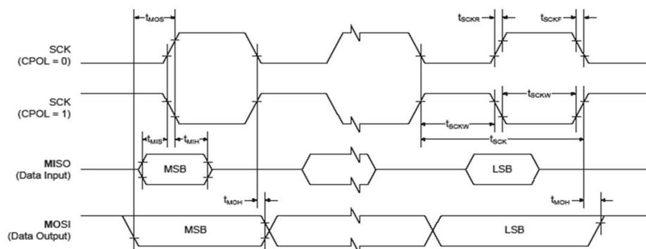
Figure 46-6. SPI Timing Requirements in Client Mode
