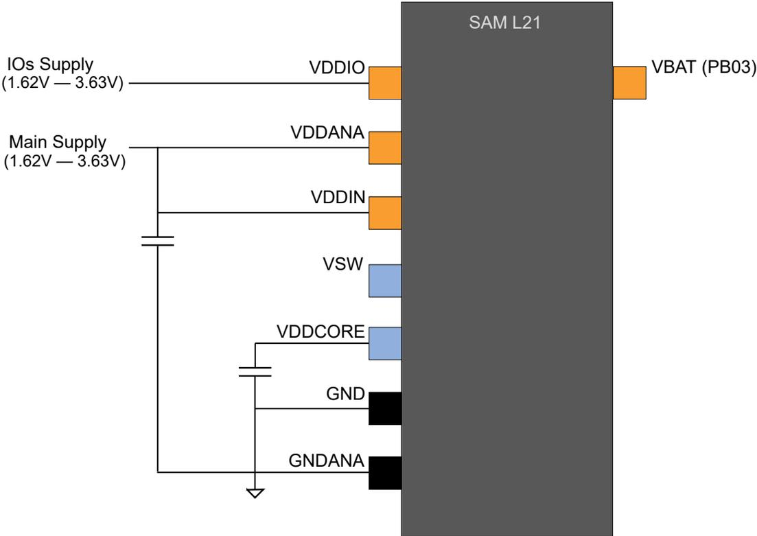
Figure 9-2. Power Supply Connection for Switching/Linear Mode
