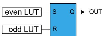
When the even LUT is disabled (LUTCTRL2x.ENABLE=0), the latch output will be cleared. The R-input is forced enabled for one more APB clock cycle and S-input to zero. In all other cases, the latch output (OUT) is refreshed as shown in [Table 40-5](#).
