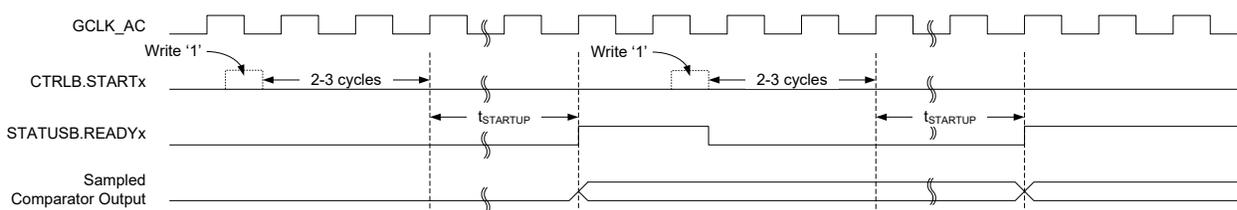
For low-power operation, event-triggered measurements can be performed during sleep modes. When the event occurs, the Power Manager will start GCLK\_AC. The comparator is enabled, and after the startup time has passed, a comparison is done and appropriate peripheral events and interrupts are also generated. The comparator and GCLK\_AC are then disabled again automatically, unless configured to wake up the system from sleep.
