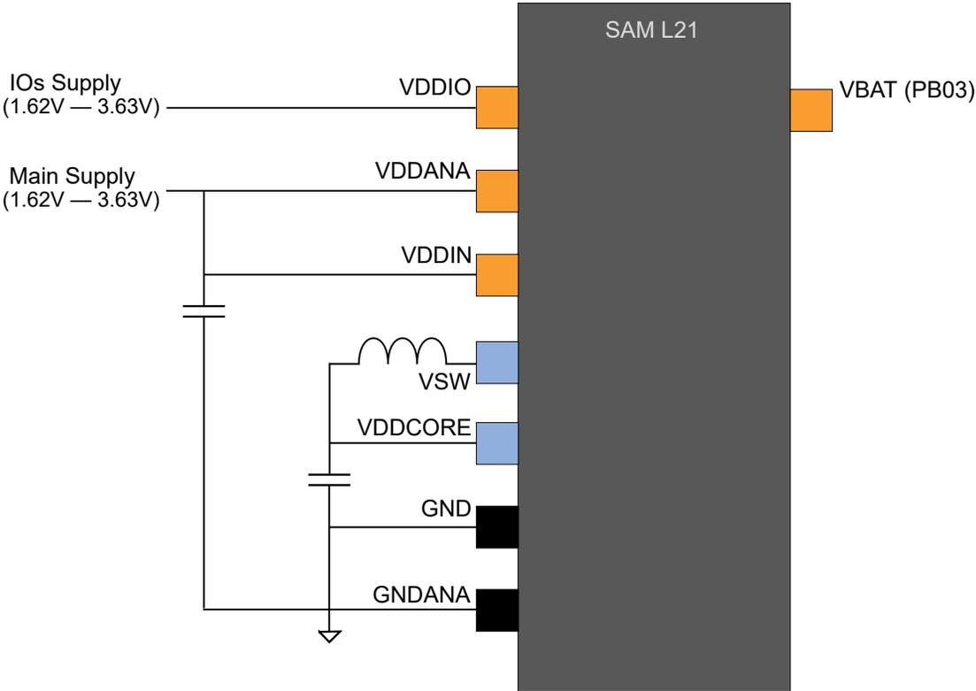
**Figure 9-3.** Power Supply Connection for Battery Backup
