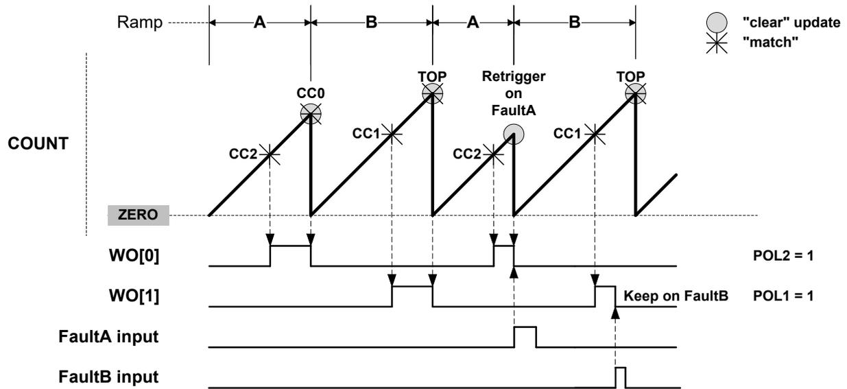
Figure 36-21. RAMP2 Critical Operation With 2 Channels
