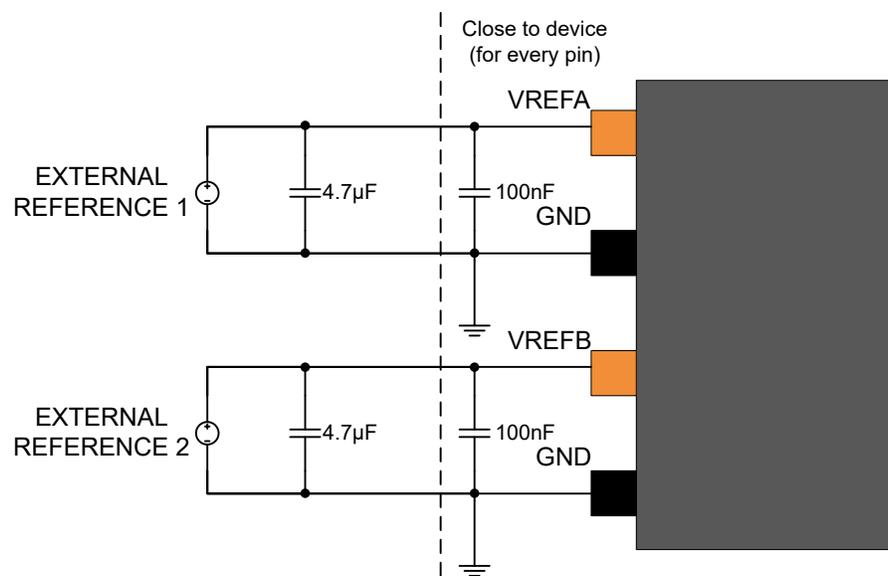
Figure 51-5. External Analog Reference Schematic With One Reference
