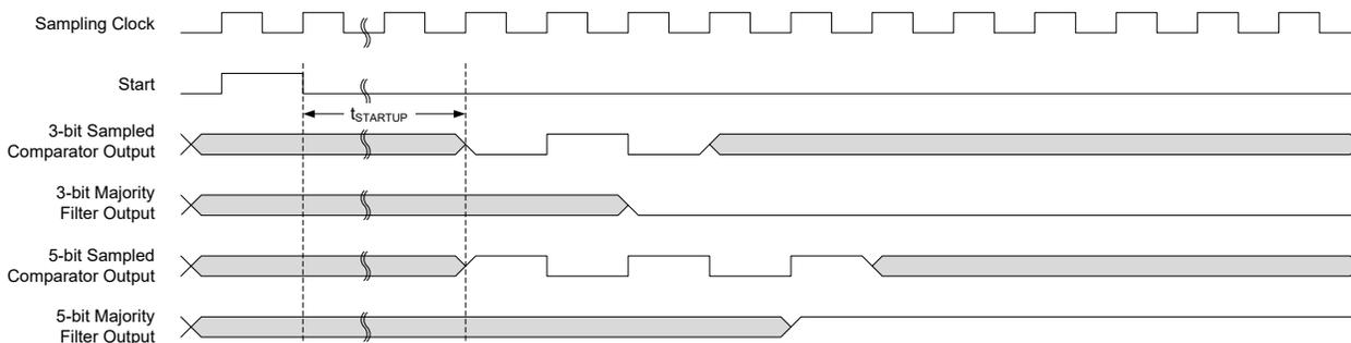
During sleep modes, filtering is supported only for single-shot measurements. Filtering must be disabled if continuous measurements will be done during sleep modes, or the resulting interrupt/event may be generated incorrectly.
