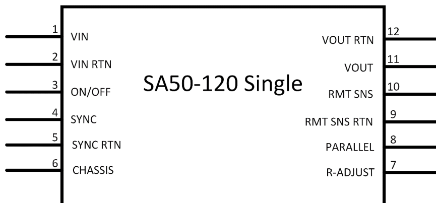
Figure 9-1. SA50 Single Pin Configuration
