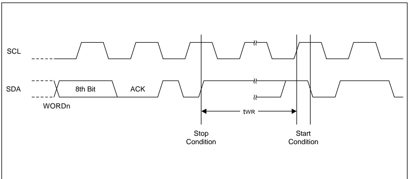
Figure 5-16. Write Cycle Timing Diagram
