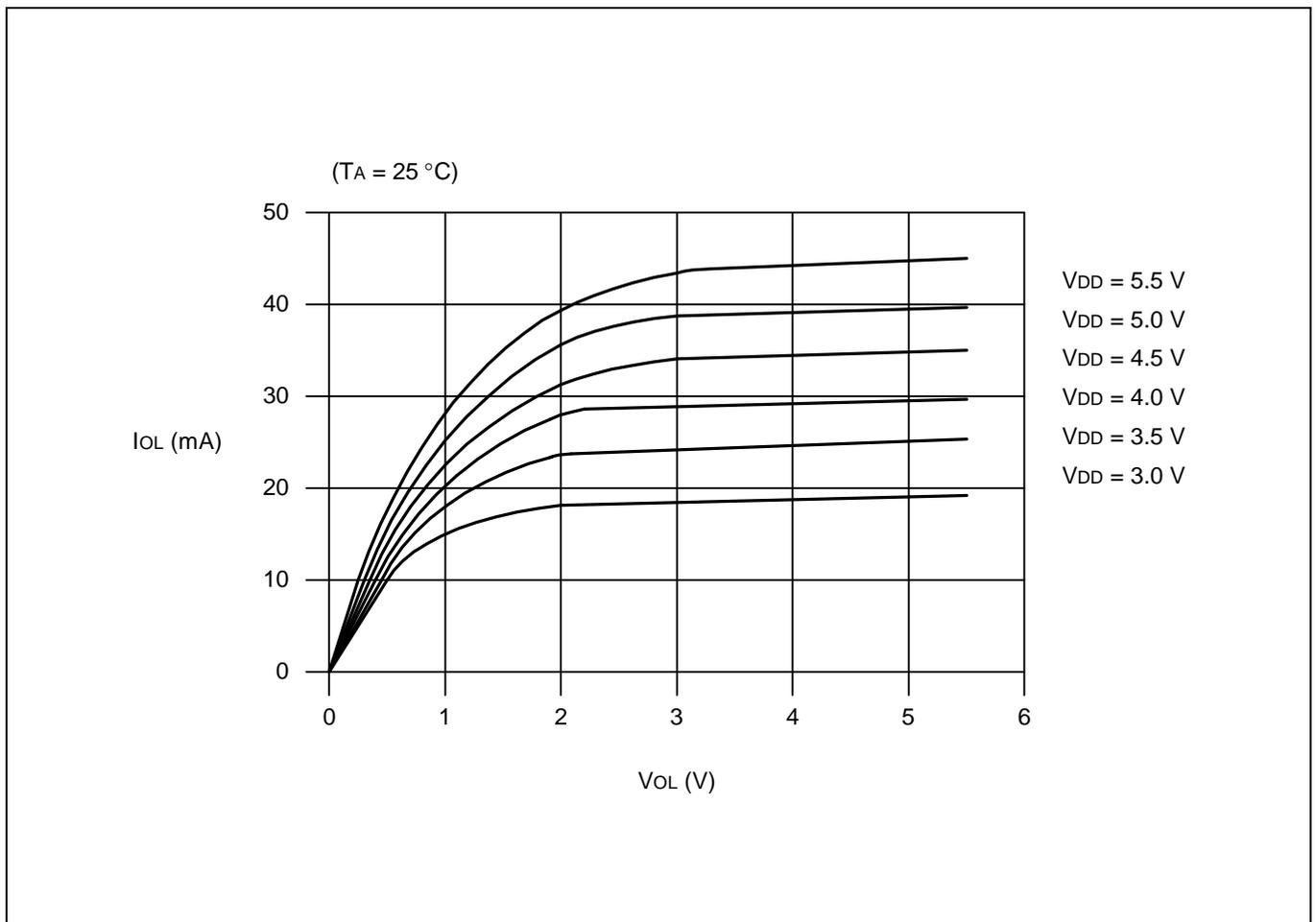
Figure 4-21. I<sub>OL</sub> (Output Low Voltage) vs. V<sub>OL</sub>
