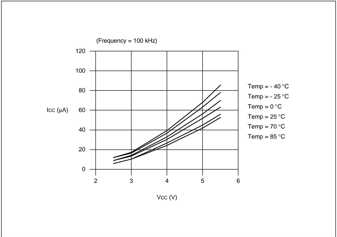
Figure 4-19. I<sub>CC</sub> (Read Current) vs. V<sub>CC</sub>
