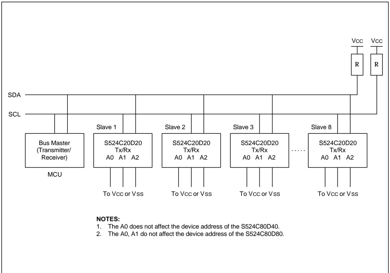
**Figure 4-6. Typical Configuration (16 Kbits of Memory on the I<sup>2</sup>C-Bus)**
