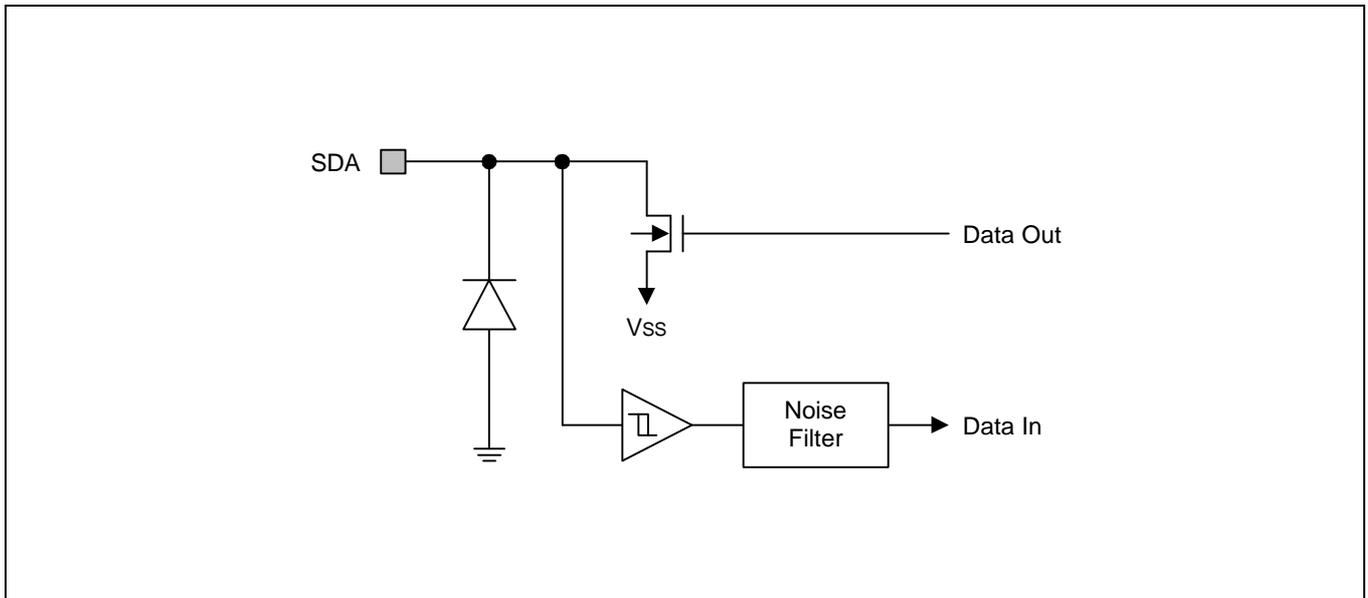
Figure 4-5. Pin Circuit Type 3
