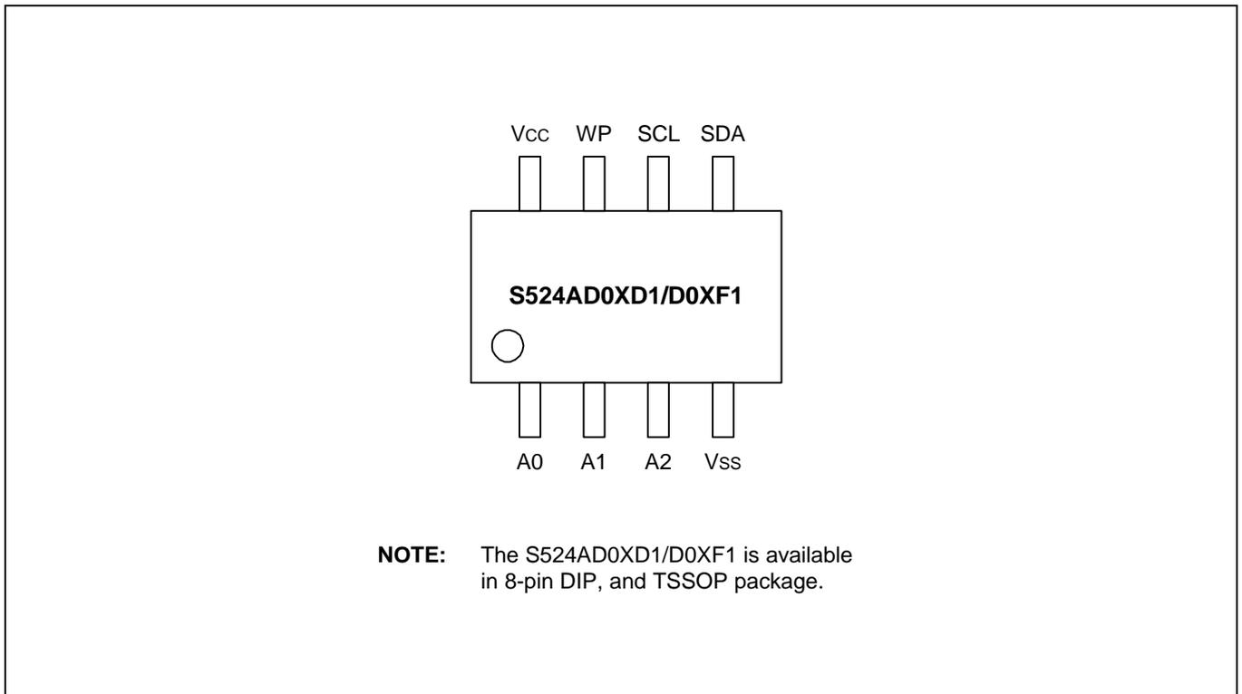
Figure 8-2. Pin Assignment Diagram
