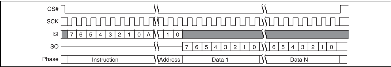
Figure 69 Fast Read Command (FAST_READ 0Bh or 0Ch) sequence without read latency
