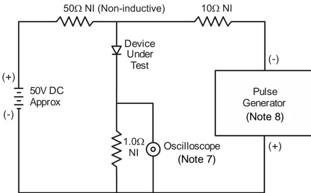
Figure 5 Reverse Recovery Time Characteristic and Test Circuit
