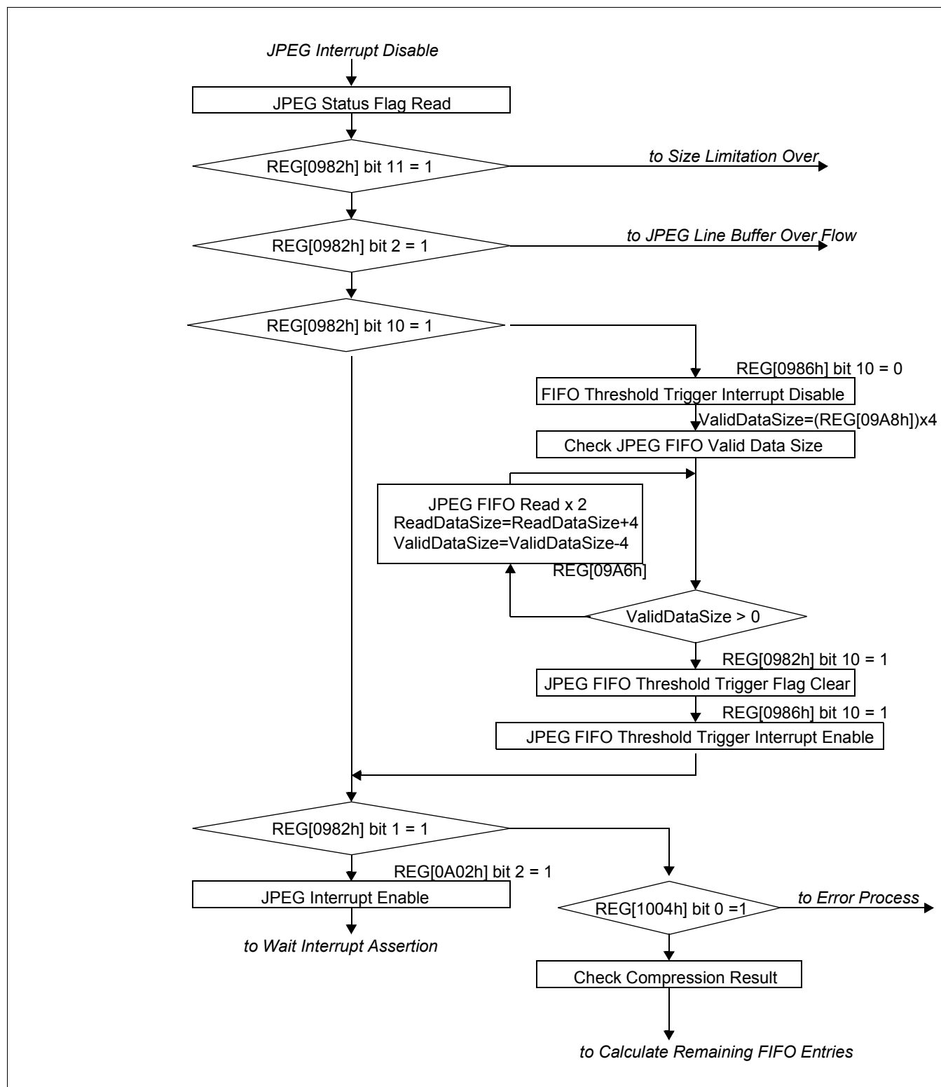
Figure 19-4: JPEG Encoding Process (3 of 4)
