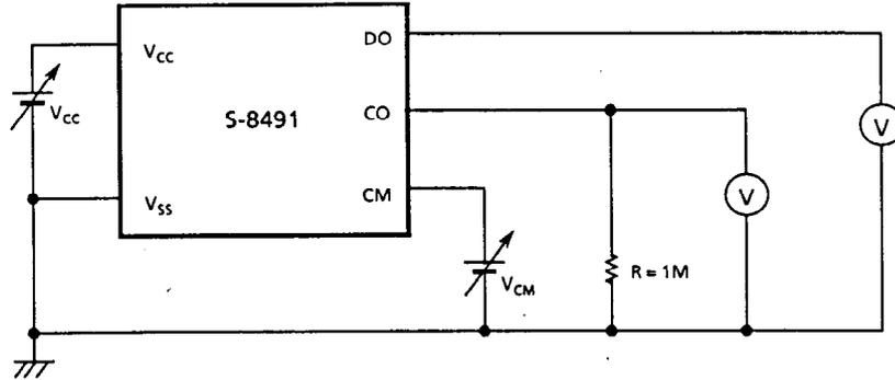
To measure excess charge detection time  $T_{CU}$ , excess discharge detection time  $T_{DD}$ , and excess current detection time  $T_{OFF}$ , follow these steps:
