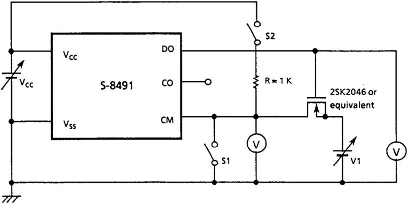
To measure excess current detection voltage  $V_{IOV}$ , follow the step:
