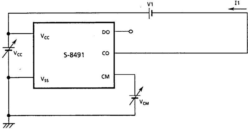
To measure CO 'H' voltage  $V_{CO(H)}$ , follow the step:
