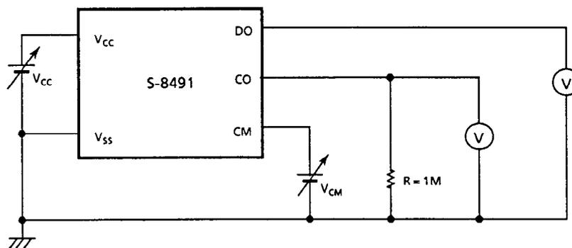
To measure excess charge detection voltage V<sub>CU</sub>, excess charge release voltage V<sub>CD</sub>, excess discharge detection voltage V<sub>DD</sub>, and excess discharge release voltage V<sub>DU</sub>, follow these steps:
